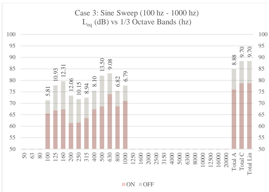
Figure 29: L_{eq} - 1/3 octave band noise measurement results for Case 3 - Sine Sweep (100 hz - 1000 hz) T_{sweep}=10s
