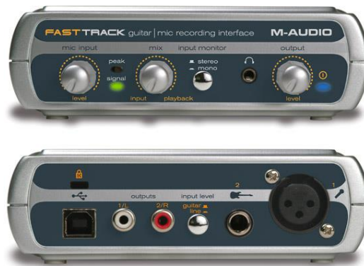
Figure 19: USB Audio interface used as a part of the noise generator system.
