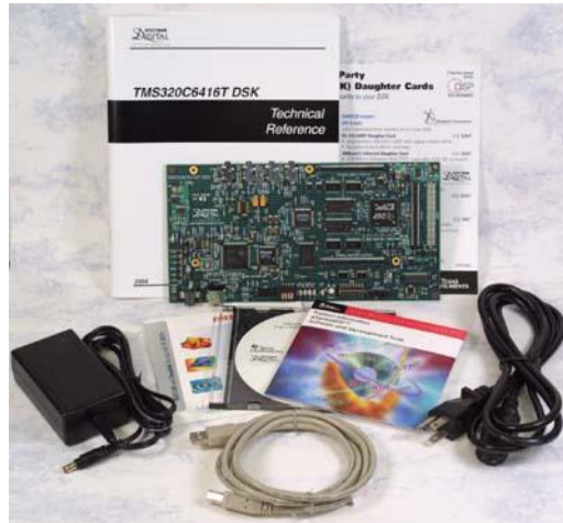
Figure 23: DSP Kit used in ANC system.
