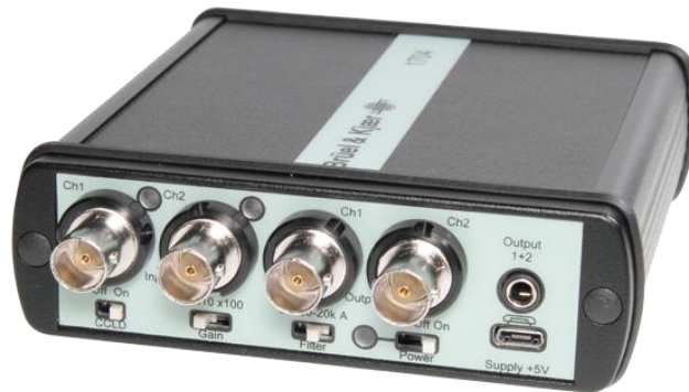
Figure 22: Signal conditioner used in ANC system.
