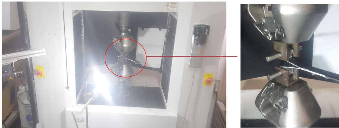
Figure A. 3: The test machine for Mode I test
