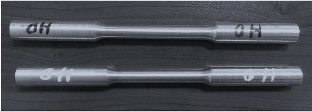
Figure 17 Preliminary tensile test specimens for the base metal (7039 as obtained) in accordance with ASTM B557
