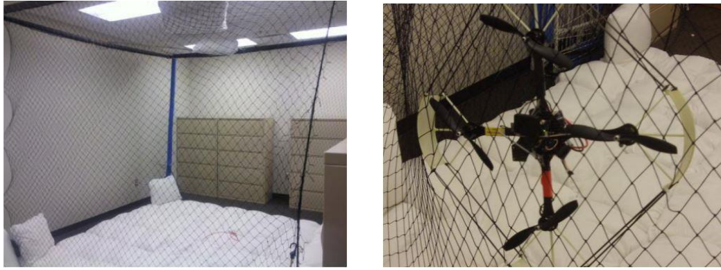
(a) Flying area with pillows and net (b) Quadrotor after hitting net
