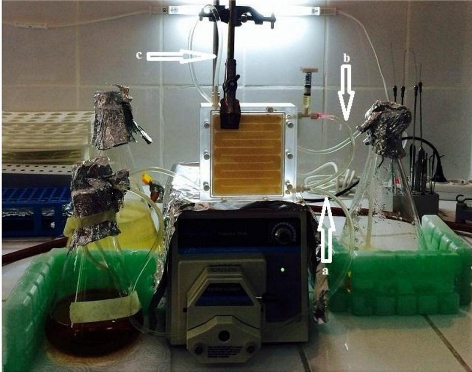
Figure 2.1 Ultrafiltration system for Panomycocin a) feed, b) return, c) filtrate.
