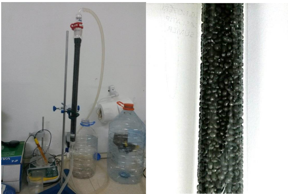
Figure 2.3 Photos of the set-up for column experiments
