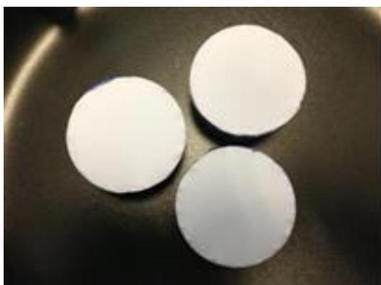
**Figure 2.5.** The photographs of nanofibrous matrices after the cross-linking treatment.
