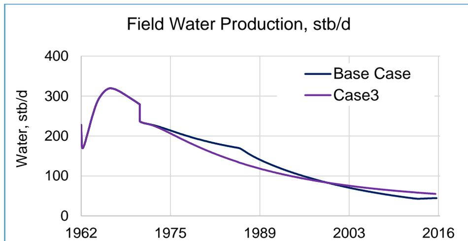
**Figure 5.11.** Comparison of base case and scenario-3 water production rates
