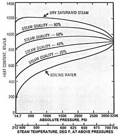
**Figure 2.12.** Heat content of boiling water and dry saturated steam at different pressure (Ali Farouq, 1989.)
