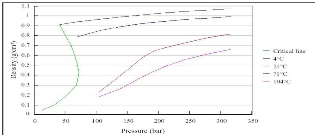
**Figure 2.6.** Density of CO<sub>2</sub> with respect to temperature and pressure (Holm, 1987)
