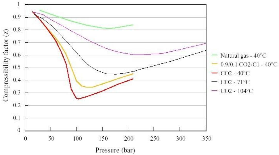
**Figure 2.7.** Compressibility of CO<sub>2</sub> with respect to pressure and temperature (McQuarrie, Donald A. (1999))
