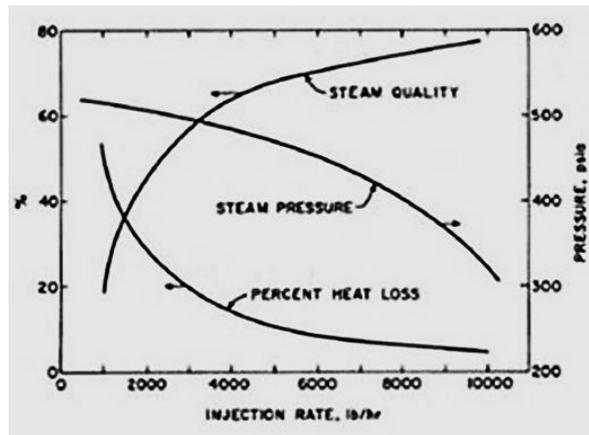
**Figure 2.13.** Heat loss in the wellbore in comparison with injection rate
