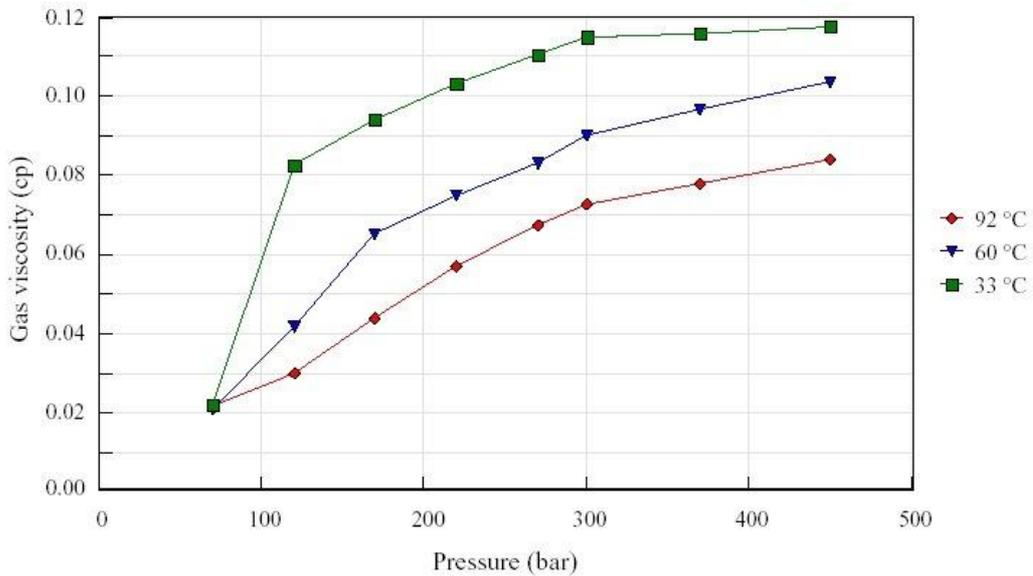
**Figure 2.8.** Viscosity of CO<sub>2</sub> with respect to temperature and pressure (Lee, A.L.et.al .1966)
