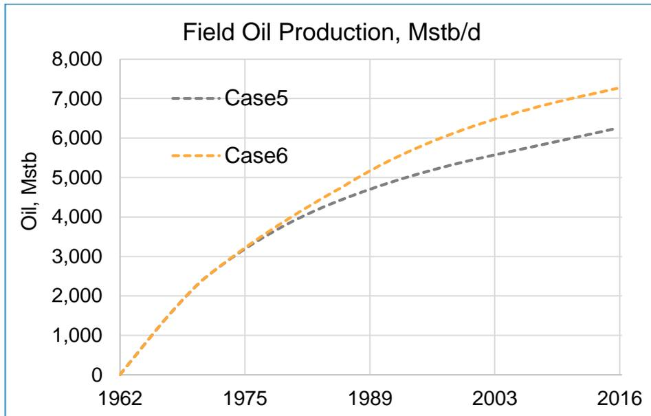
**Figure 5.24** Effect of water injection and CO<sub>2</sub> injection before steam injection on cumulative oil production
