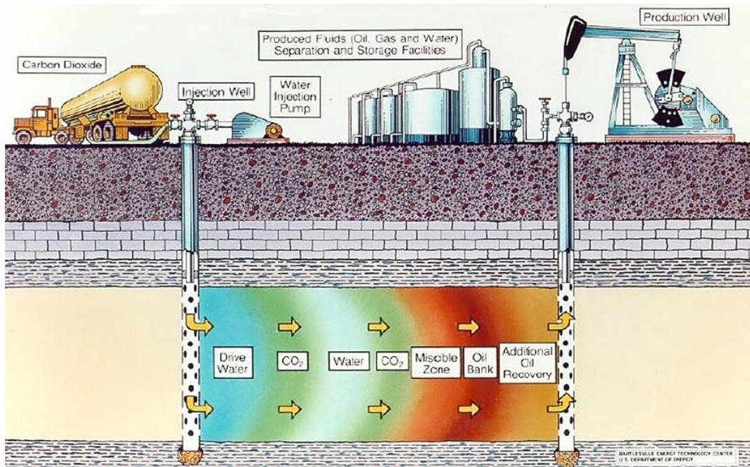
**Figure 2.3.** A schematic view of water alternating gas process of miscible CO<sub>2</sub> injection. (CO<sub>2</sub> surfactants, 2014)
