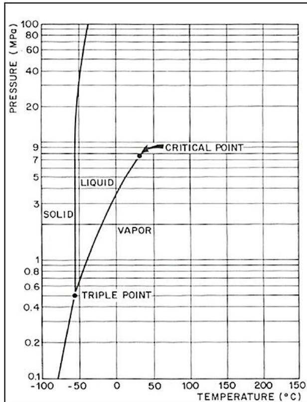
**Figure 2.5.** Phase diagram of carbon dioxide (Baviere, 1980)
