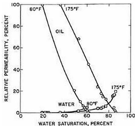
**Figure 2.11.** Effect of temperature on relative permeability (Weinbrandt and Ramey, 1972)
