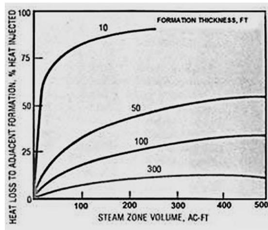
**Figure 2.14.** Variation of heat losses to the formation with formation thickness (Herbeck et.al. 1978)
