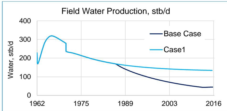
**Figure 5.6.** Comparison of base case and scenario-1 water production rates
