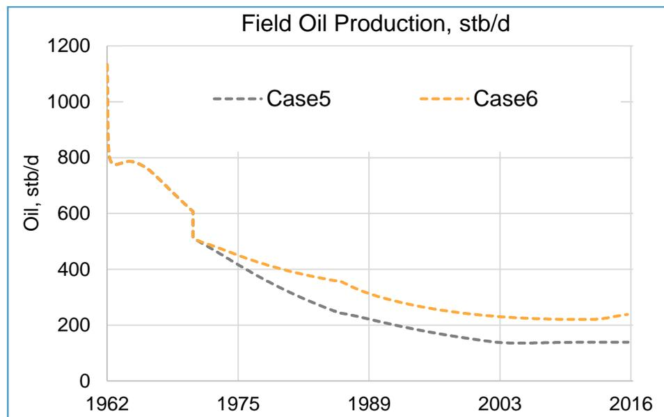
**Figure 5.23** Effect of water injection and CO<sub>2</sub> injection before steam injection on oil production rates
