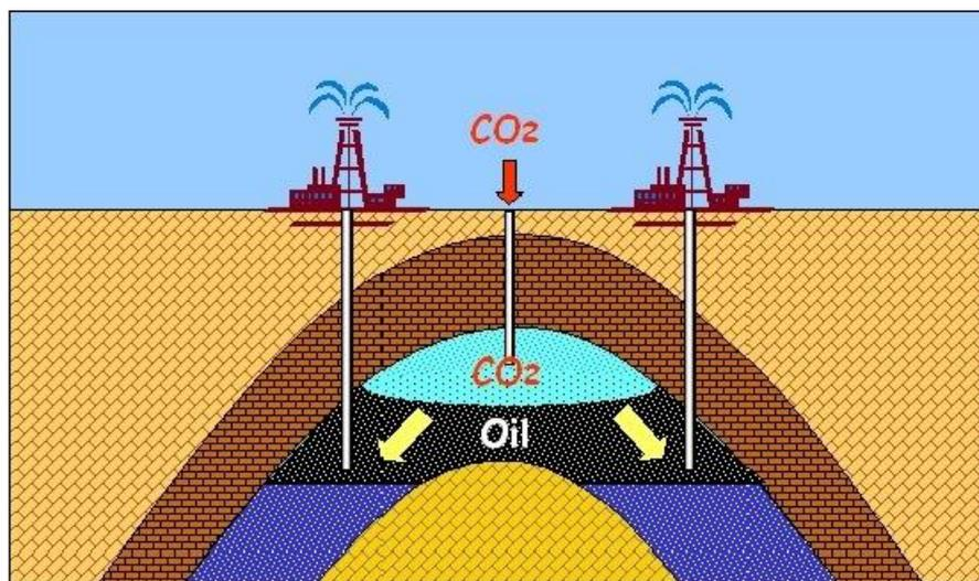
**Figure 2.4.** Schematic view of immiscible CO<sub>2</sub> injection (Tzimas et al, 2005)
