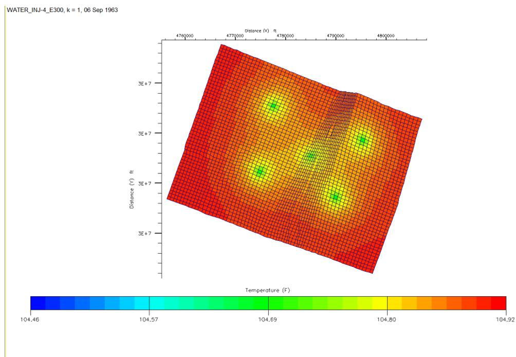
**Figure 5.19** Reservoir temperature distribution for scenario-6 on September 1963
