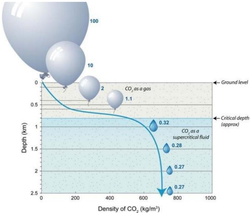
**Figure 2.1.** Depth vs. density of CO<sub>2</sub> graph (West Virginia carbon sequestration, 2008)
