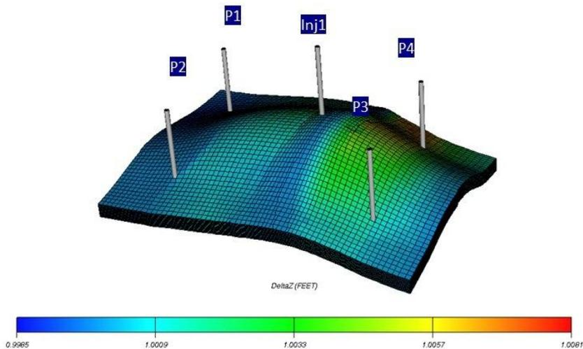
**Figure 4.6.** Central well is converted to CO<sub>2</sub>/Steam injection well
