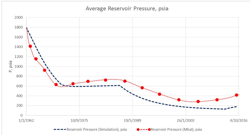
**Figure 5.34.** Average Reservoir Pressure comparison between Material Balance and Simulation
