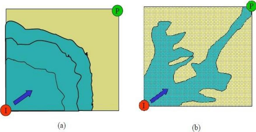
Figure 2.2. a) good recovery, b) viscous fingering (Conaway et al. 1999)
