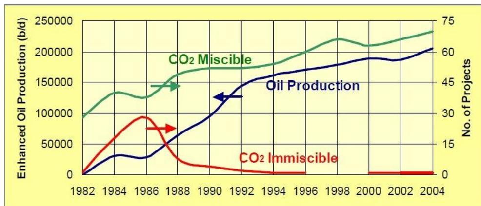
**Figure 2.9.** Development of CO<sub>2</sub> displacement techniques and cumulative rates in USA (Moritis, 2006)
