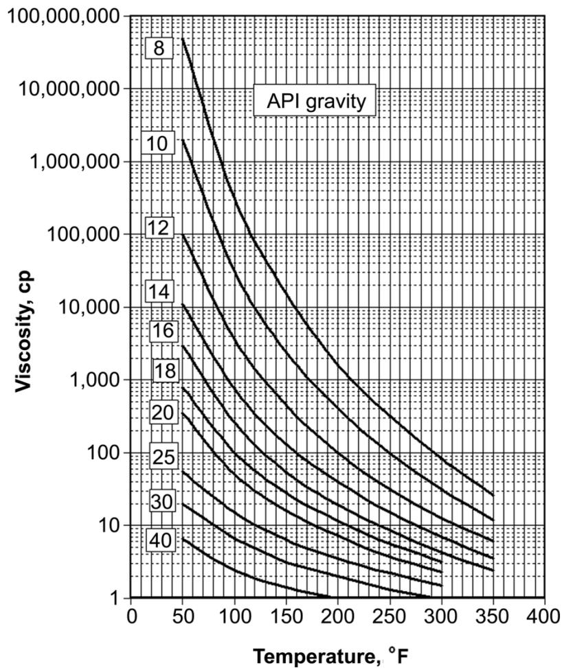
**Figure 2.10.** Viscosity of oil samples under different temperatures (Doscher and Ghassemi, 1984)
