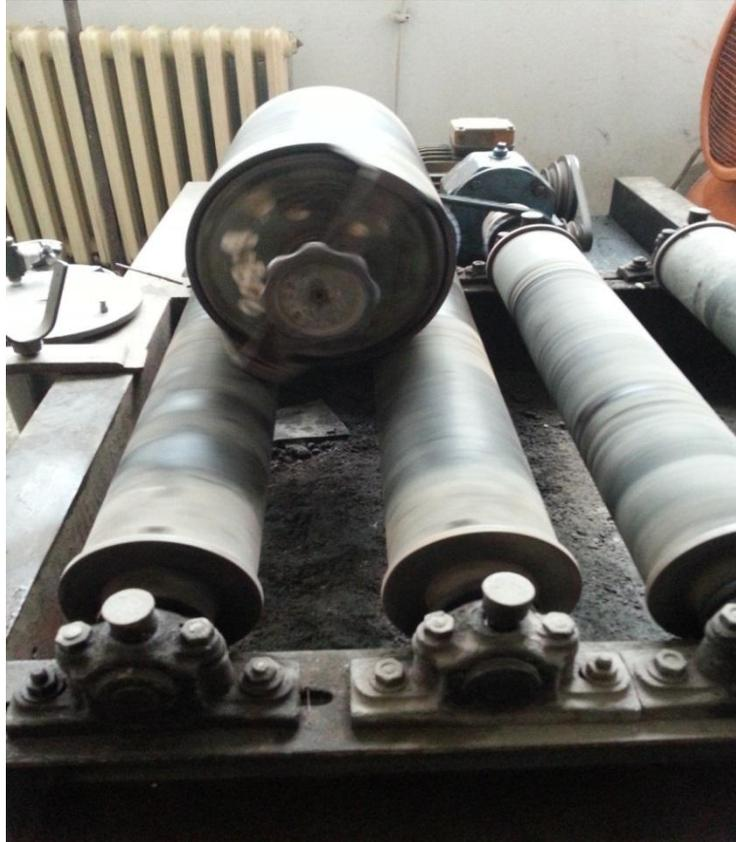
Figure 9: Laboratory Rod Mill
