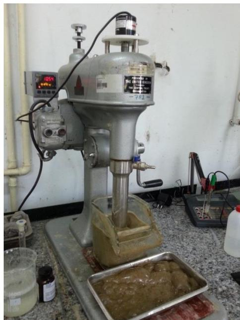
Figure 7: Denver-Sub A Laboratory Flotation Machine
