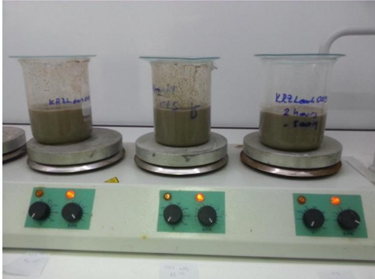
Figure 11: Agitating Sulphuric Acid Leaching Experimental Setup
