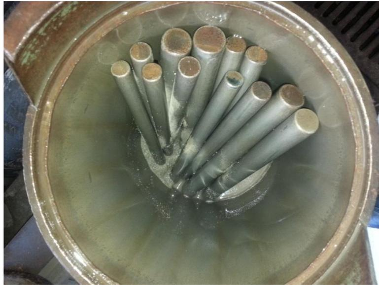
Figure 10: Grinding Mill Charge
