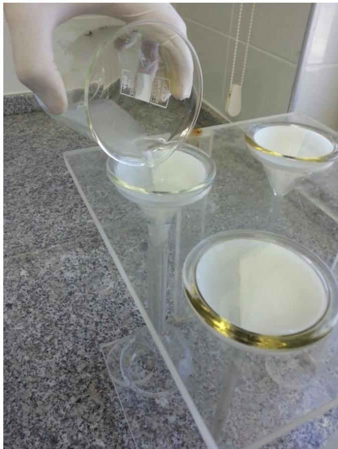
Figure 13: Filtering of the Solution
