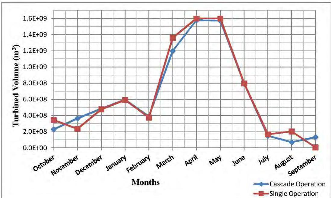
Figure 4-36: Turbined volume for LK with maximum flow data without spillway upper bound
