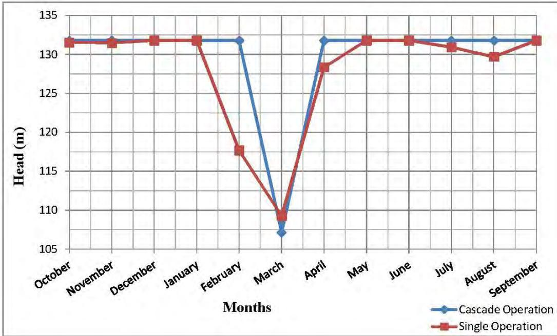
Figure 4-43: Operation head for UK with maximum flow data with spillway upper bound
