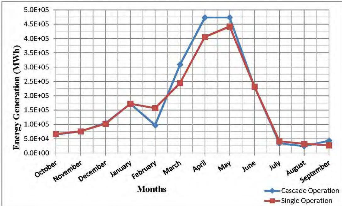
**Figure 4-51:** Energy generation for UK with maximum flow data with spillway upper bound
