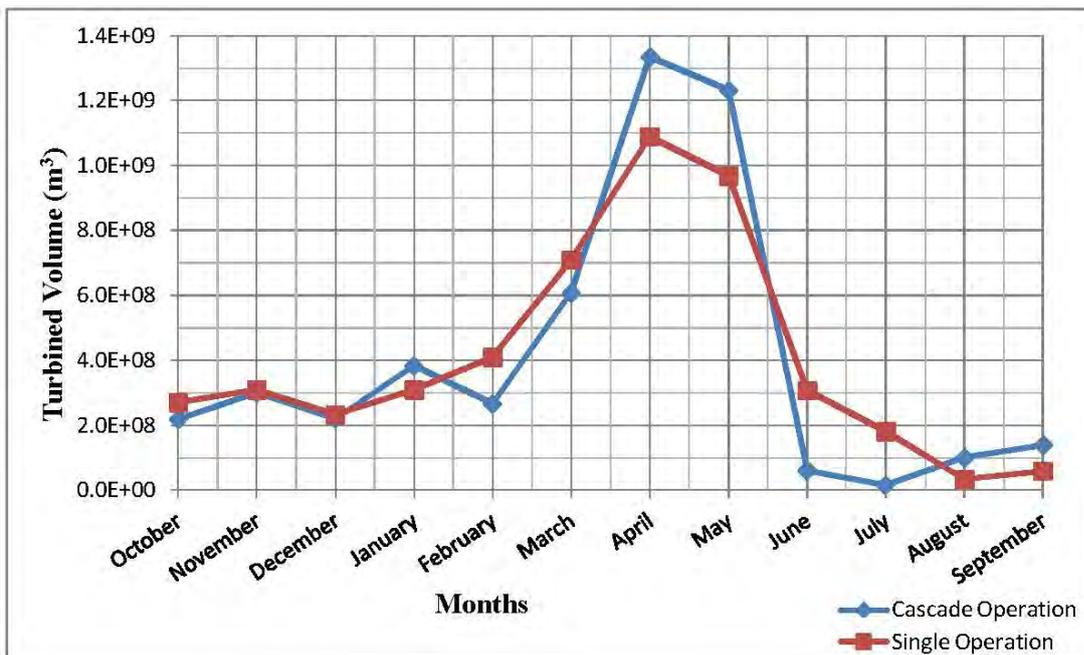
Figure 4-24: Turbined volume for LK with average flow data
