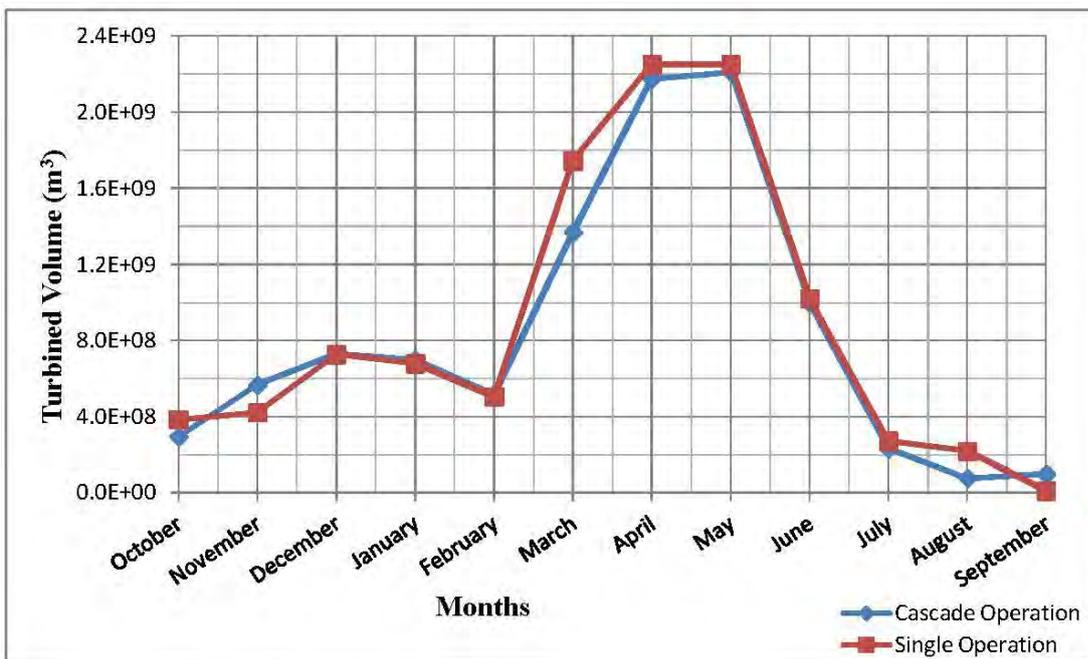
Figure 4-38: Turbined volume for B2 with maximum flow data without spillway upper bound
