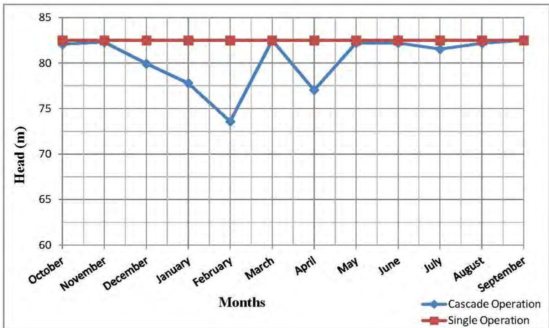
**Figure 4-32:** Operation head for LK with maximum flow data without spillway upper bound
