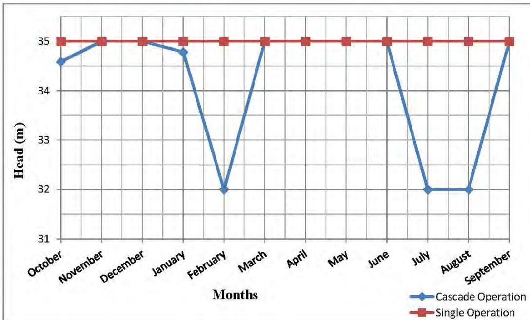
Figure 4-34: Operation head for B2 with maximum flow data without spillway upper bound
