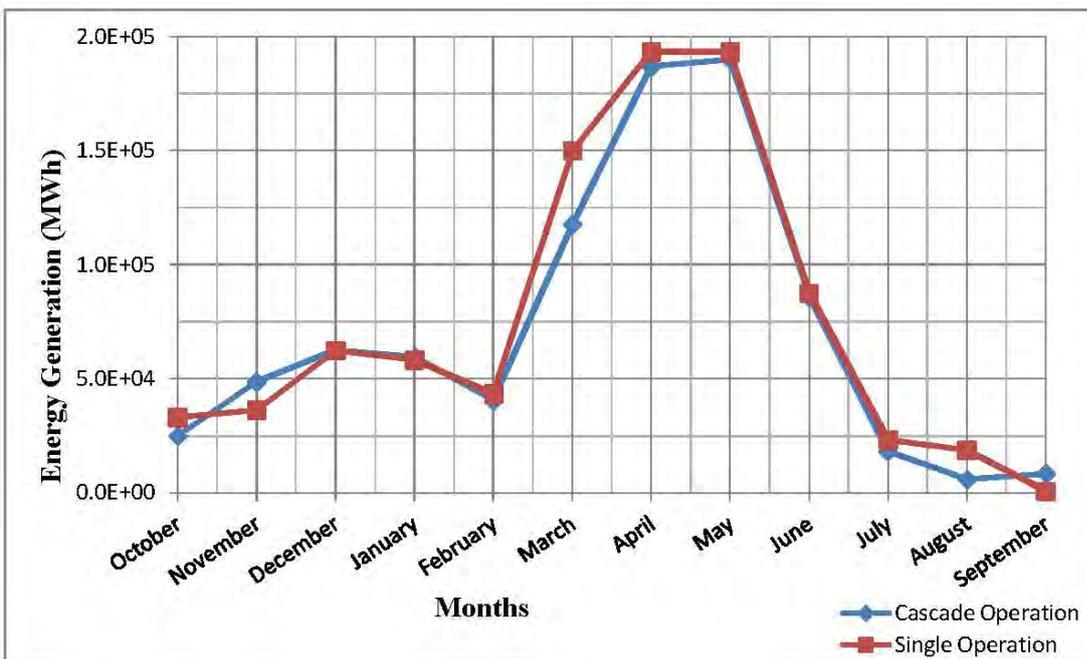
**Figure 4-42:** Energy generation for B2 with maximum flow data without spillway upper bound
