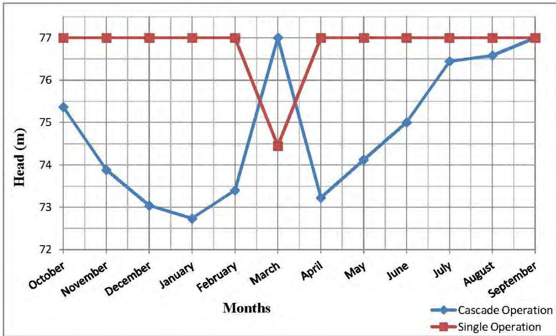
Figure 4-33: Operation head for B1 with maximum flow data without spillway upper bound
