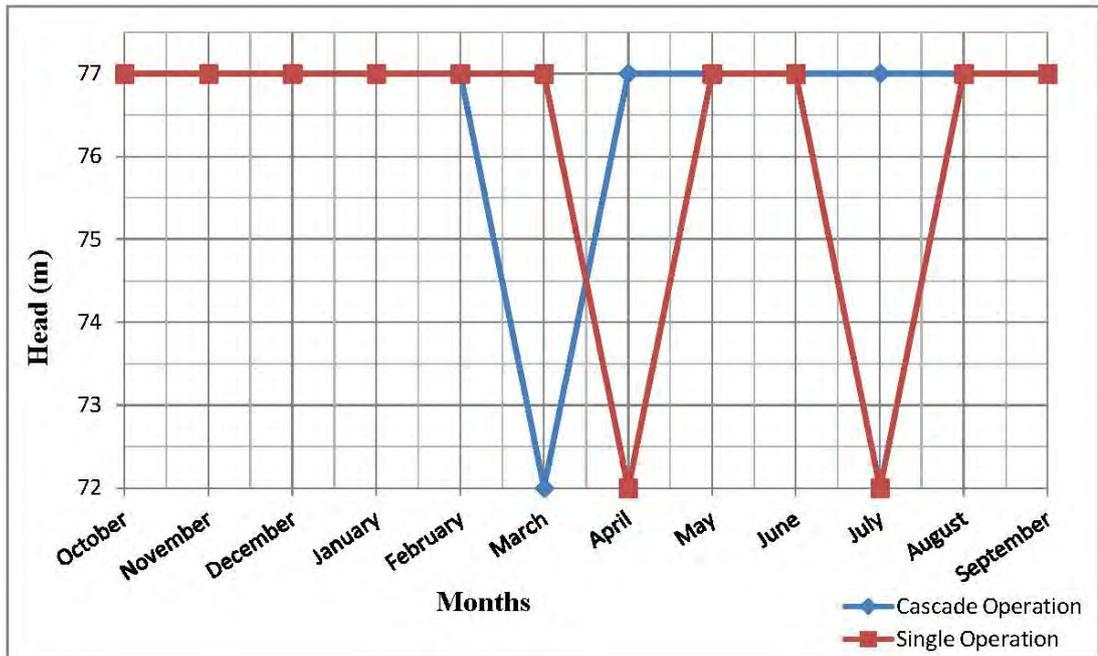
**Figure 4-45:** Operation head for B1 with maximum flow data with spillway upper bound
