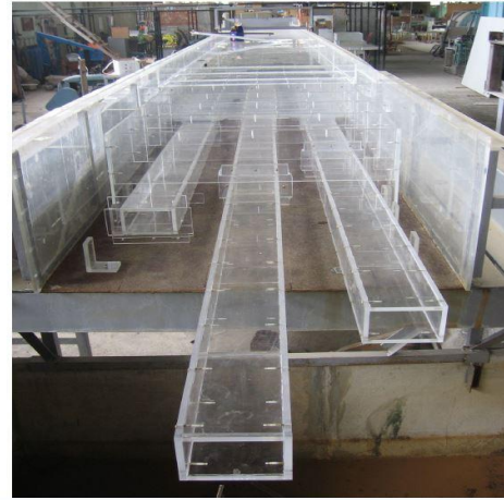
Figure 5.8b Experimental Setup (Pools for Water Collecting System)
