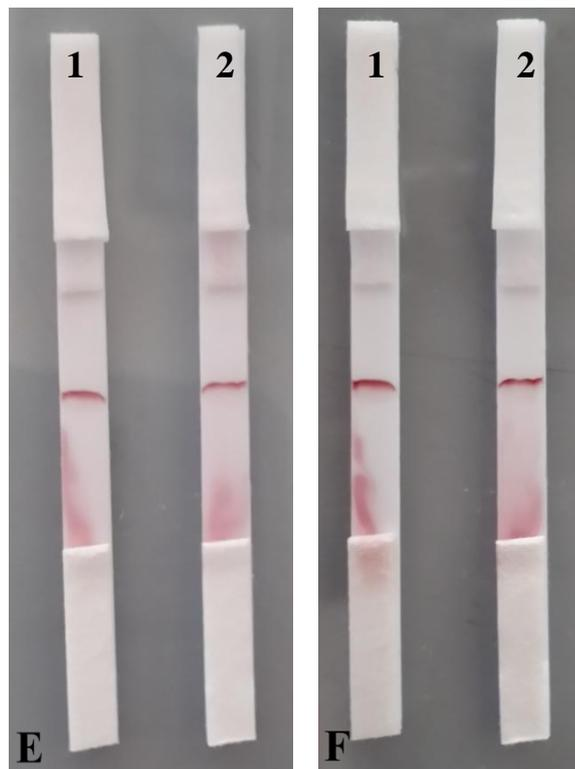
**Figure 3.24** Results of 284 bp amplicon application to the assay. E and F denote assay results before washing and after washing, respectively. 1:2 diluted 284 bp amplicon was applied to strip 1 while 1:3 diluted was applied to strip 2
