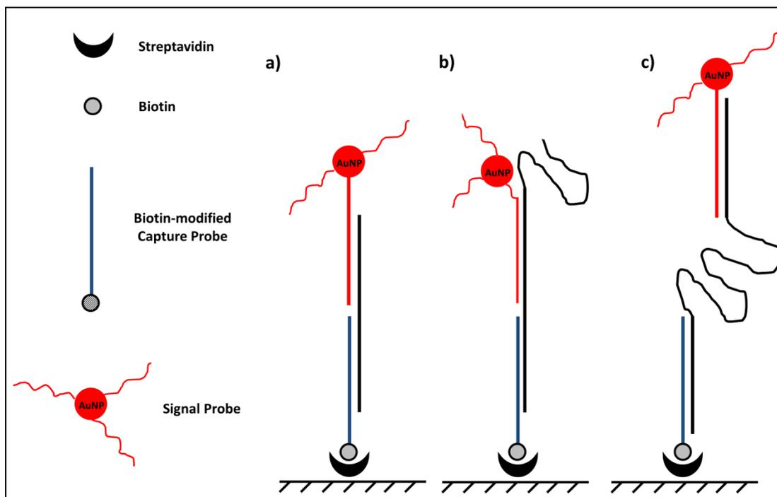
**Figure 3.19** Illustration of detection of target nucleic acids by sandwich hybridization. **a**, **b**, and **c** represent the synthetic target, 105 bp amplicon and 284 bp amplicon, respectively
