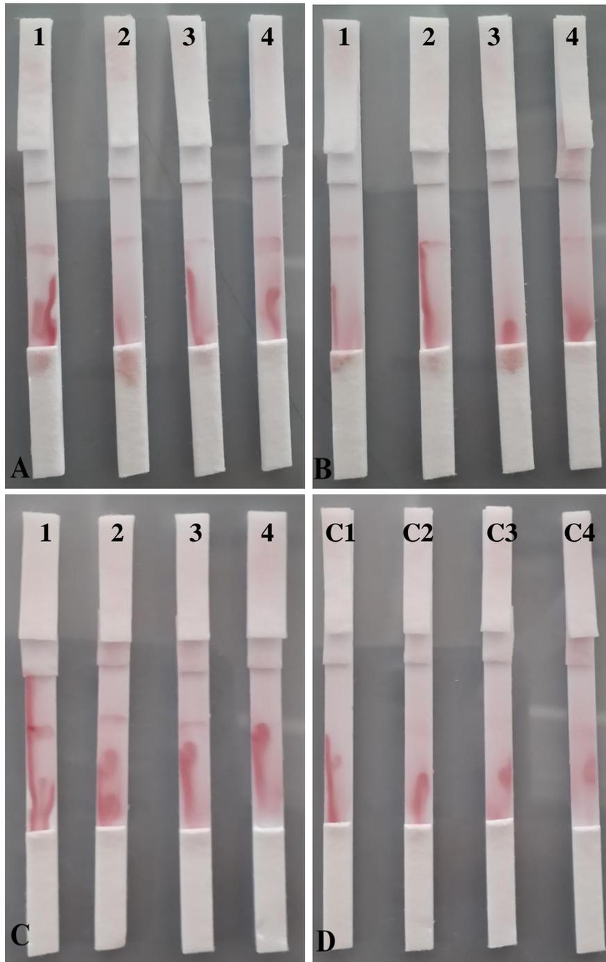
**Figure 3.25** Results of the assay, before washing. Figures A, B and C represent sources of the 284 bp target, *S. infantis*, *S. enteritidis*, and *S. typhimurium*, respectively. Numbers 1, 2, 3 and 4 in each figure indicate the dilution ratio of the target; 1:2, 1:3, 1:5 and 1:10, respectively. Controls used in the assay are shown in Figure D; C1, C2, C3 and C4 are 1:2 diluted MCS, 1:5 diluted, 1:2 diluted PCR mix containing no DNA and 5X SSC, respectively
