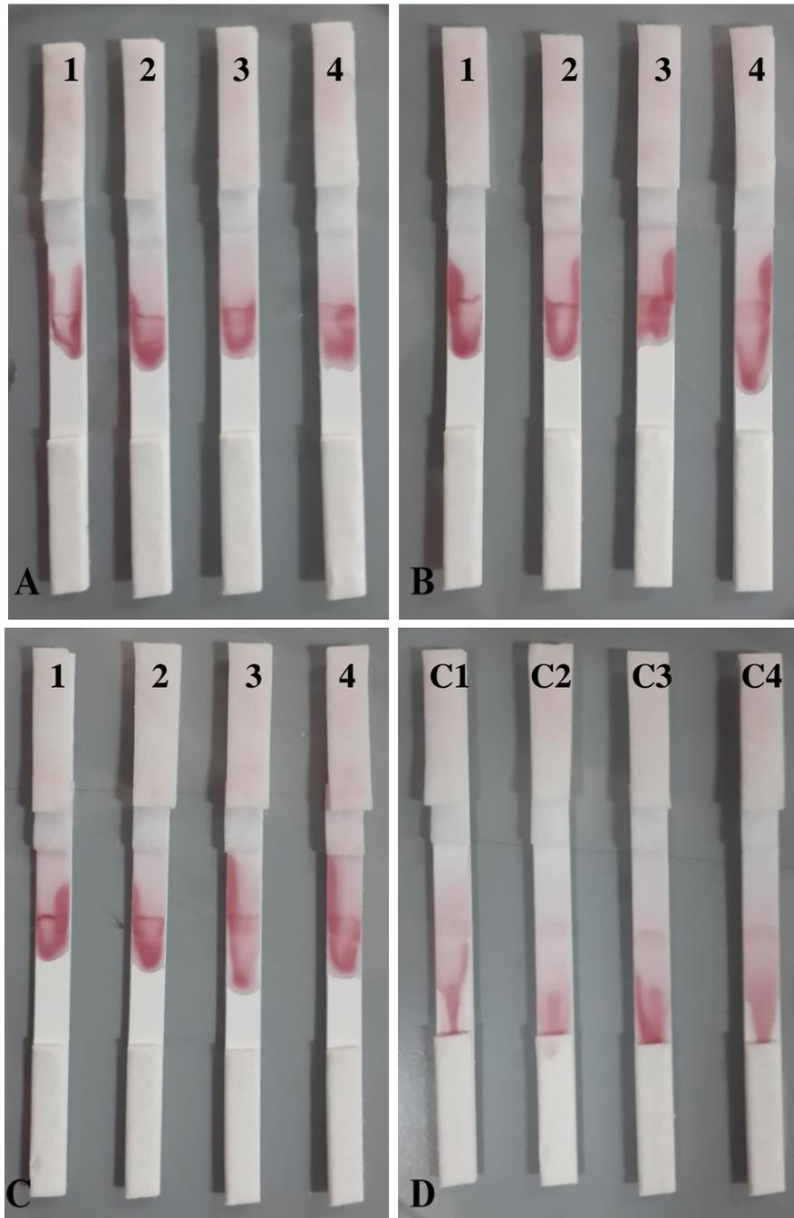
**Figure 3.22** Results of the assay, before washing. Figures A, B and C represent sources of the 105 bp target, *S. infantis*, *S. enteritidis*, and *S. typhimurium*, respectively. Numbers 1, 2, 3 and 4 in each figure indicate the dilution ratio of the target; 1:2, 1:3, 1:5 and 1:10, respectively. Controls used in the assay are shown in Figure D; 1:2 diluted MCS, 1:5 diluted MCS, 1:2 diluted PCR mix containing no DNA and 5X SSC, respectively
