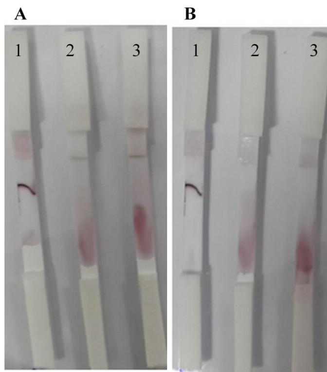
**Figure 3.20** Assay results of synthetic target. Figure A shows the strips before washing and figure B shows the strips after washing with 5X SSC. Synthetic target, uncomplementary control oligonucleotide and 5X SSC were applied to the strips 1, 2 and 3, respectively
