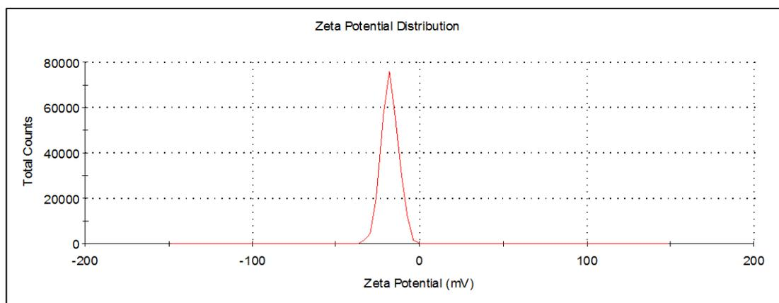
**Figure 3.16** Zeta potential distribution of signal probe 1
