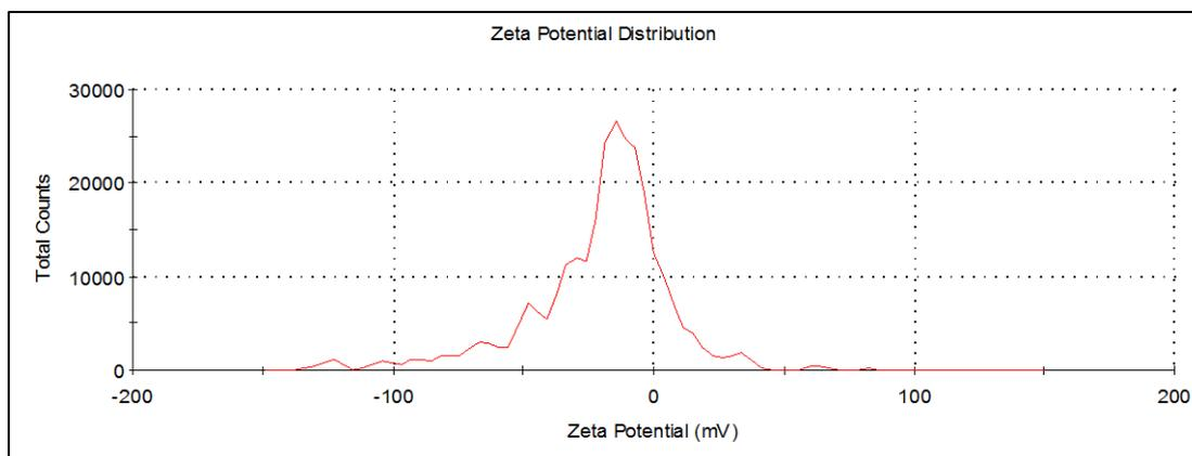
**Figure 3.11** Zeta potential distribution of 25 nm AuNPs at neutral pH
