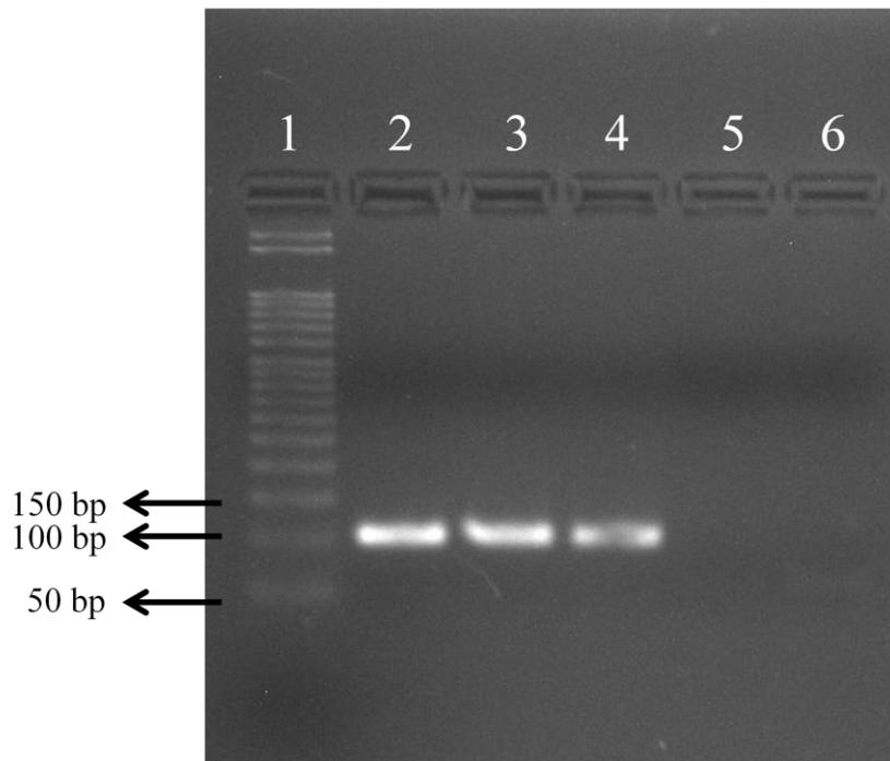
**Figure 3.7** 2.5 % agarose gel electrophoresis. Lane 1: 50 bp DNA ladder. Lanes 2, 3 and 4: 105 bp amplicons of *S. infantis*, *S. enteritidis* and *S. typhimurium*, respectively. Lane 5: *E. coli* DH5 $\alpha$ . Lane 6: Control for PCR
