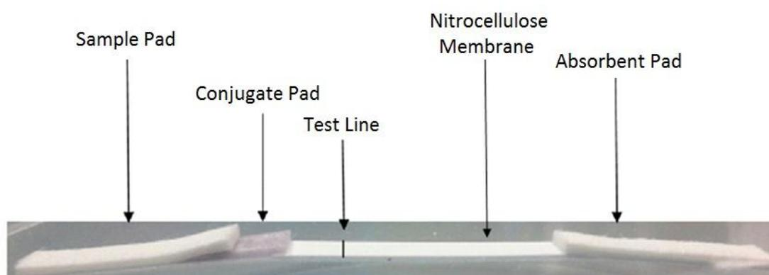
**Figure 3.18** Components of lateral flow immunochromatographic test strip
