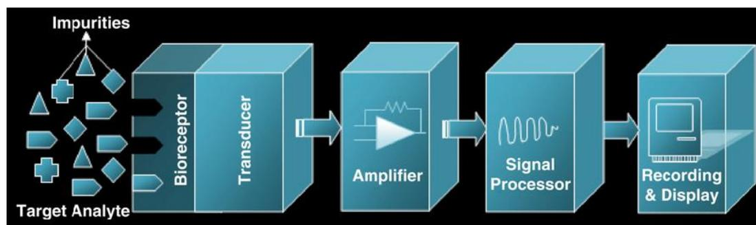
**Figure 1.10** Schematic representation of a typical biosensor (Velusamy *et al.*, 2010)
