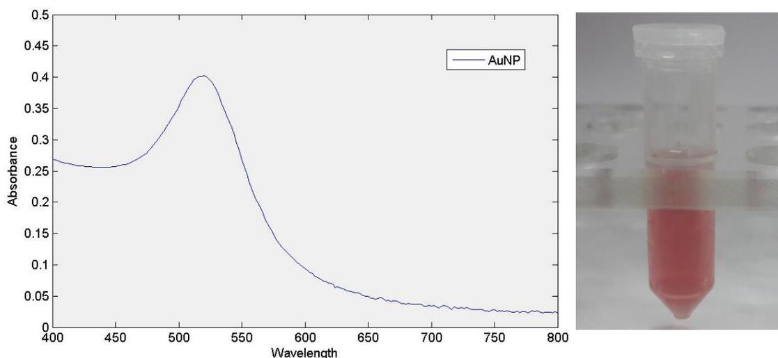
**Figure 3.9** Absorption spectrum (left) and visual appearance (right) of synthesized AuNPs
