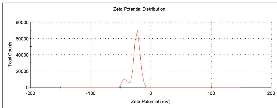
**Figure 3.17** Zeta potential distribution of signal probe 2
