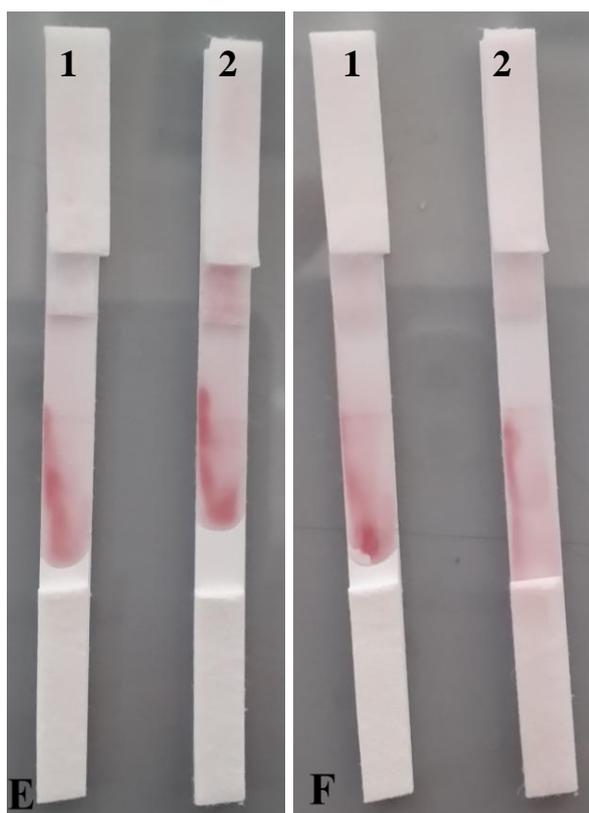
**Figure 3.27** Results of 105 bp amplicon target application to the assay. E and F denote assay results before washing and after washing, respectively. 1:2 diluted 105 bp amplicon was applied to strip 1 while 1:3 diluted was applied to strip 2
