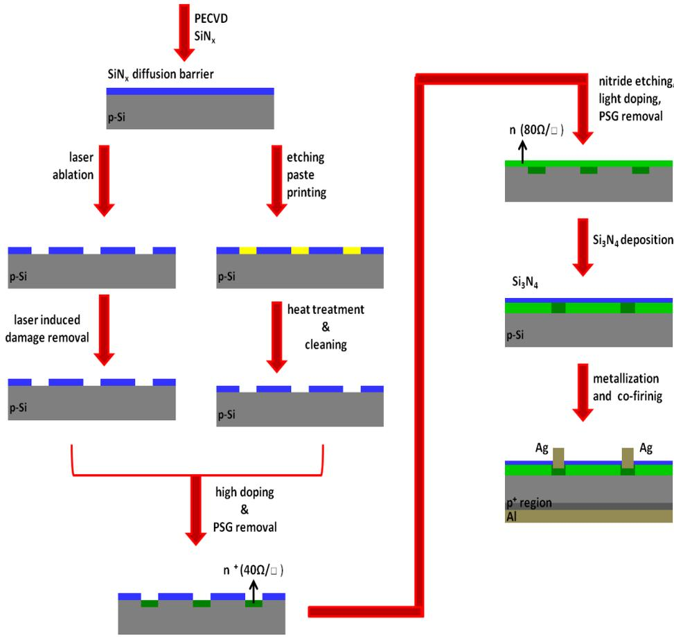
**Figure 37: Fabrication process of selective emitter solar cells using silicon nitride diffusion barrier**
