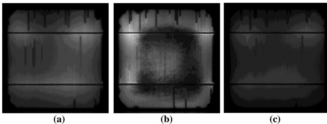
**Figure 75: Electroluminescence images of selective emitter cells with (a) 20, (b) 30, and (c) 50 nm mask oxide. Lines are for visual aid**
