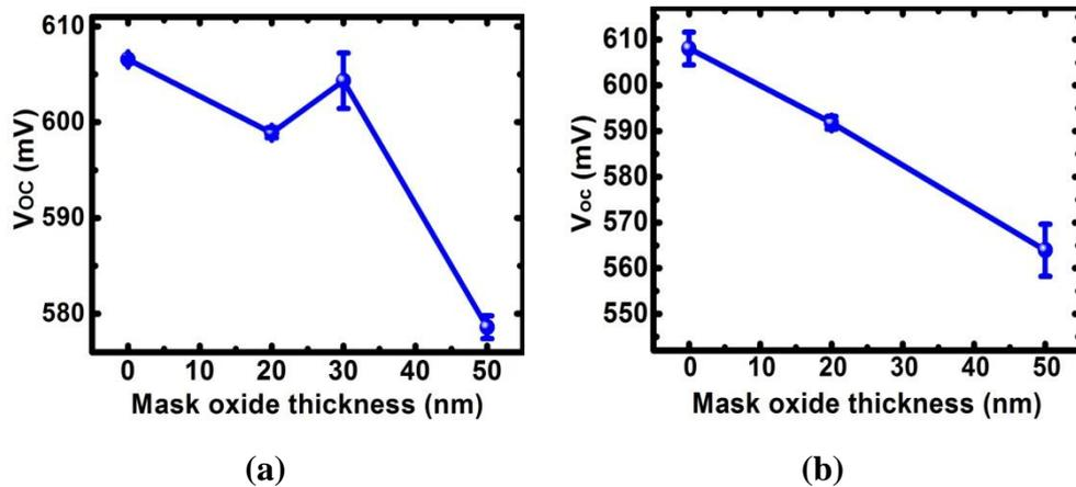
**Figure 80: Effect of mask oxide thickness on  $V_{oc}$  (a) with (b) without oxide passivation. Lines are for visual aid**
