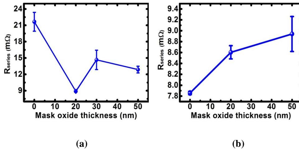
**Figure 74: Effect of mask oxide thickness on  $R_{series}$  (a) with oxide passivation, (b) without oxide passivation. Lines are for visual aid**
