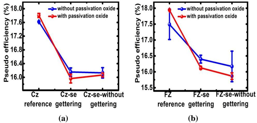
**Figure 92: Pseudo efficiency values of fabricated (a) Cz and (b) FZ Cells. Lines are for visual aid**
