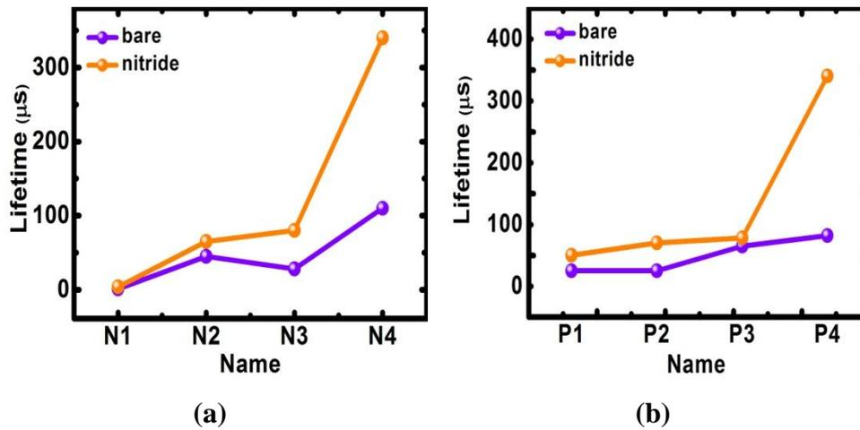
**Figure 104: Effect of standard nitride deposition on effective lifetime of (a) n-type, (b) p-type DSP wafers. Lines are for visual aid**
