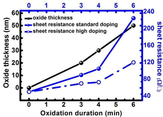
**Figure 53: Oxidation duration, oxide thickness and sheet resistance relationship**
