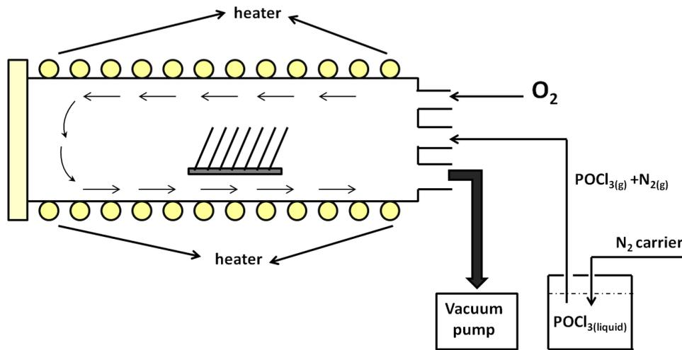
**Figure 45: Schematic of doping furnace**
