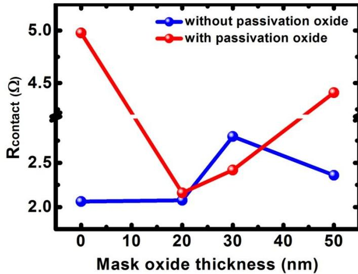
**Figure 85: Effect of mask oxide thickness on contact resistance. Lines are for visual aid**
