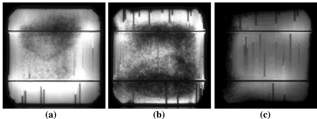
**Figure 77: Electroluminescence images of oxide passivated selective emitter cells with (a) 20, (b) 30 and (c) 50 nm mask oxide. Lines are for visual aid**
