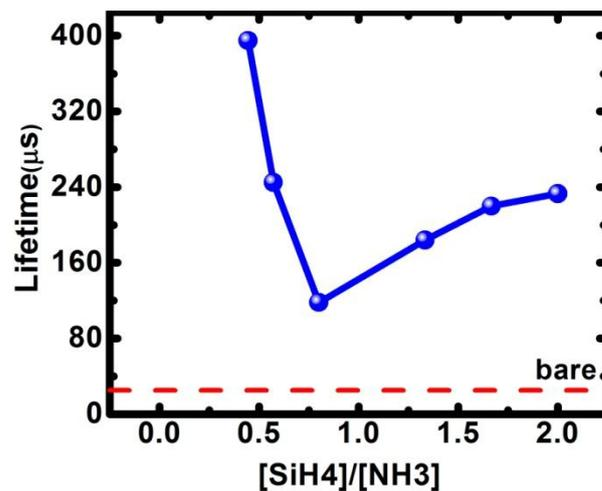
**Figure 103: Effect of process gas flow ratios on lifetime of SSP wafers**
