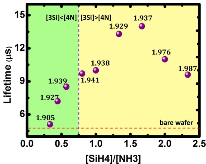
Figure 102: Effect of process gas flow ratios on lifetime
