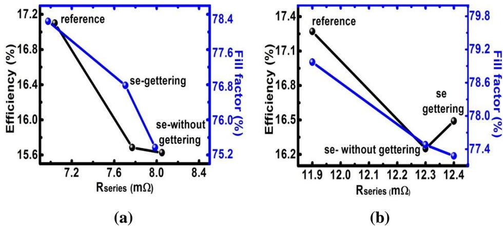
**Figure 91: Series resistance-fill factor-efficiency relationship of fabricated (a) Cz and (b) FZ cells. Lines are for visual aid**
