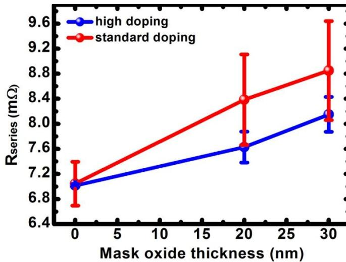
Figure 57: Effect of mask oxide thickness on series resistance
