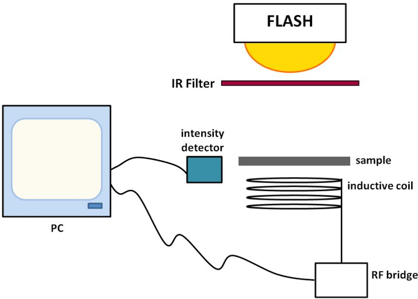
**Figure 51: Schematic of Lifetime measurement system**
