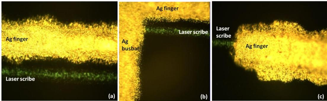
**Figure 60: Optical microscope images of (a) misaligned finger, (b) misaligned finger-busbar cross-section, (c) aligned finger under 20X magnification**
