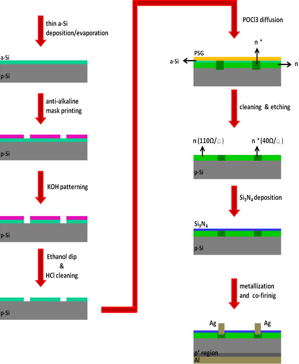
**Figure 36: Fabrication process of selective emitter solar cells using amorphous Si diffusion barrier**
