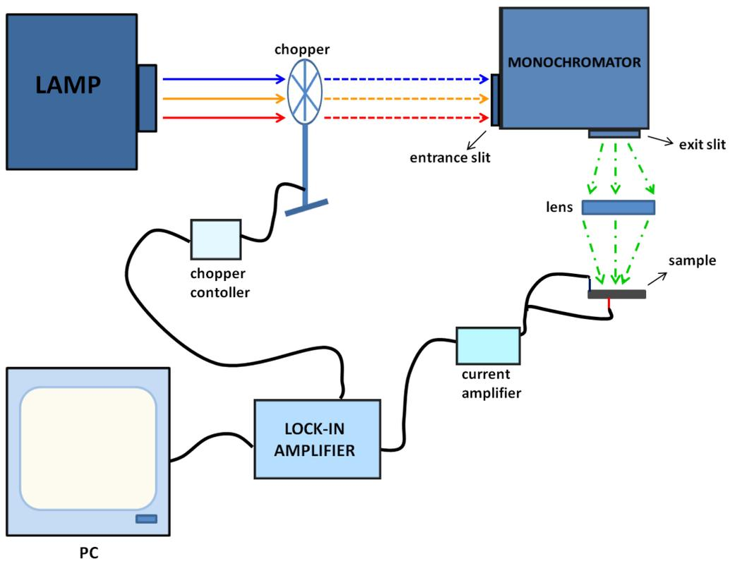
**Figure 49: Schematic of external quantum efficiency set-up placed at GUNAM Laboratories**
