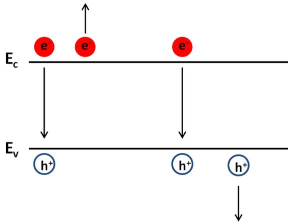
**Figure 40: Schematic of Auger recombination process**
