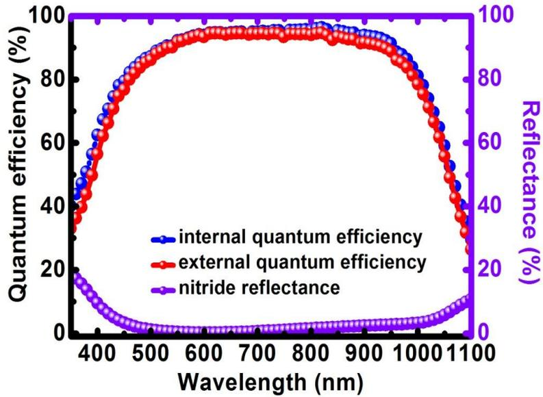
Figure 100: Internal and external quantum efficiency and corresponding reflectance spectrum of a reference cell
