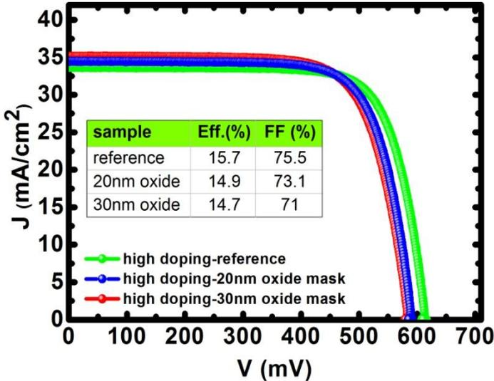
Figure 66: J-V characteristics and corresponding efficiency and fill factors of high doping selective emitter and reference cells
