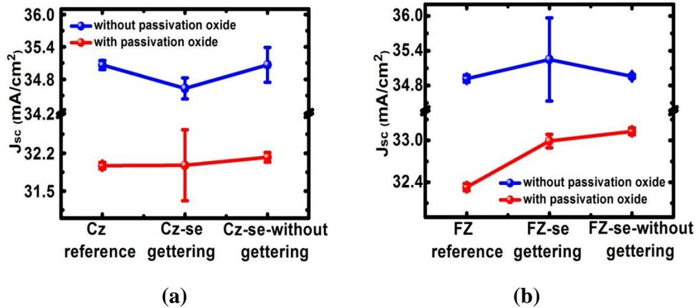
**Figure 89: Short circuit current density values of fabricated (a) Cz and (b) FZ cells. Lines are for visual aid**
