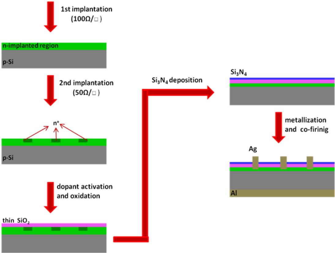
Figure 35: Fabrication process of ion implanted selective emitter solar cells
