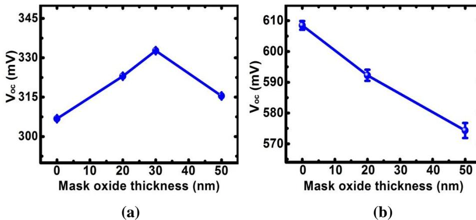
**Figure 72: Effect of mask oxide thickness on  $V_{oc}$  (a) with oxide passivation, (b) without oxide passivation. Lines are for visual aid**
