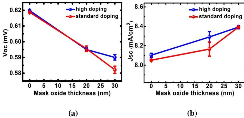
Figure 56: Effect of mask oxide thickness on (a)  $V_{oc}$ , (b)  $J_{sc}$
