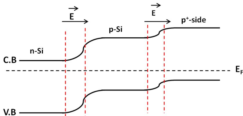
**Figure 43: Energy band diagram of a p-n junction with a back surface field at p-Side**
