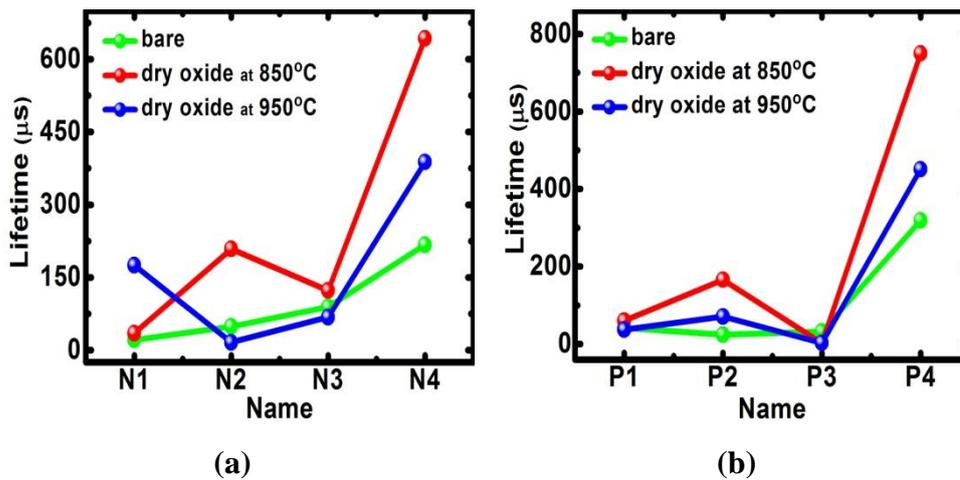
**Figure 109: Effect of oxide passivation via dry oxidation on lifetime of full (a) n-type, (b) p-type DSP wafers. Lines are for visual aid**
