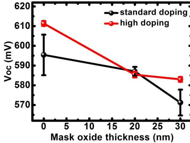
Figure 63: Effect of mask oxide thickness on  $V_{oc}$
