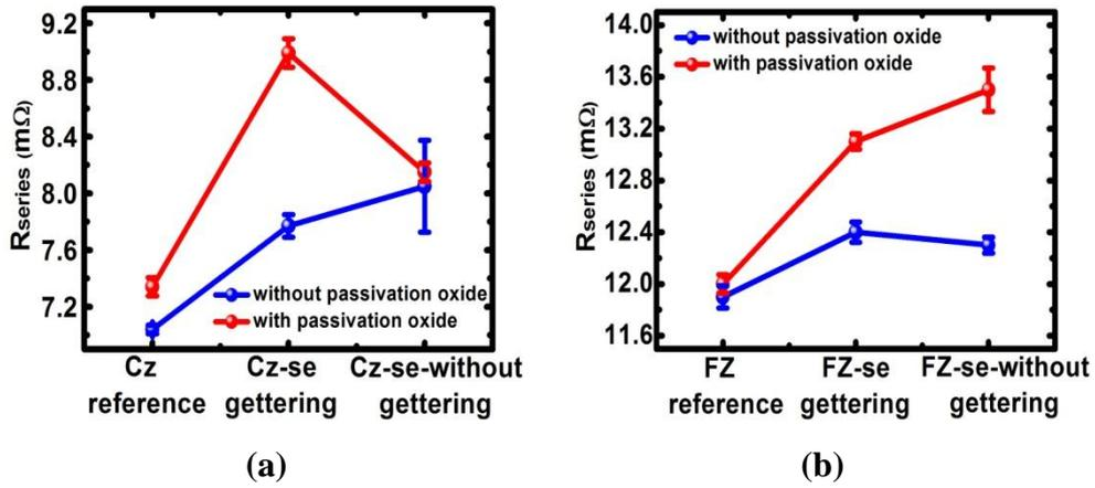
**Figure 90: Series resistance values of fabricated (a) Cz and (b) FZ cells. Lines are for visual aid**
