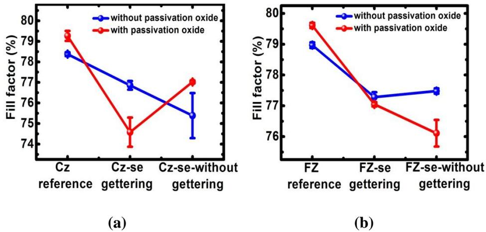
**Figure 87: Fill factor values of fabricated (a) Cz and (b) FZ cells. Lines are for visual aid**
