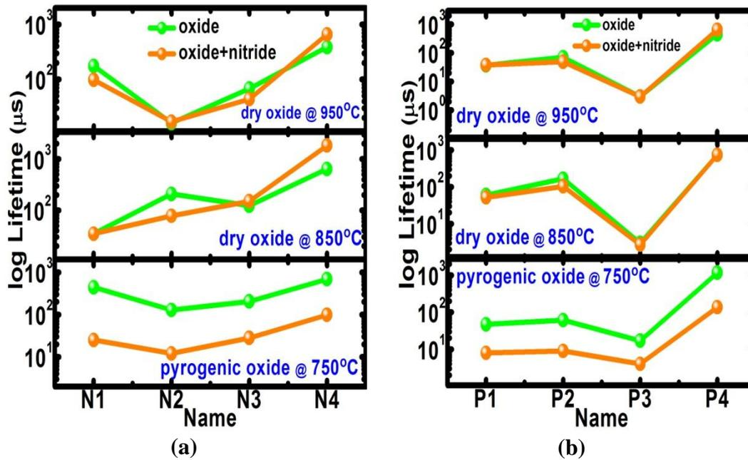
**Figure 111: Effect of nitride deposition on oxide passivated full (a) n-type, (b) p-type DSP wafers. Lines are for visual aid**
