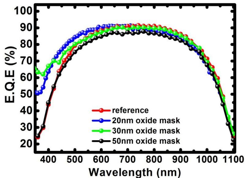
Figure 83: External quantum efficiency comparison of fabricated solar cells
