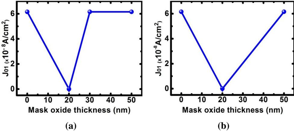
Figure 81: Effect of mask oxide thickness on J<sub>01</sub> (a) with (b) without oxide passivation. Lines are for visual aid
