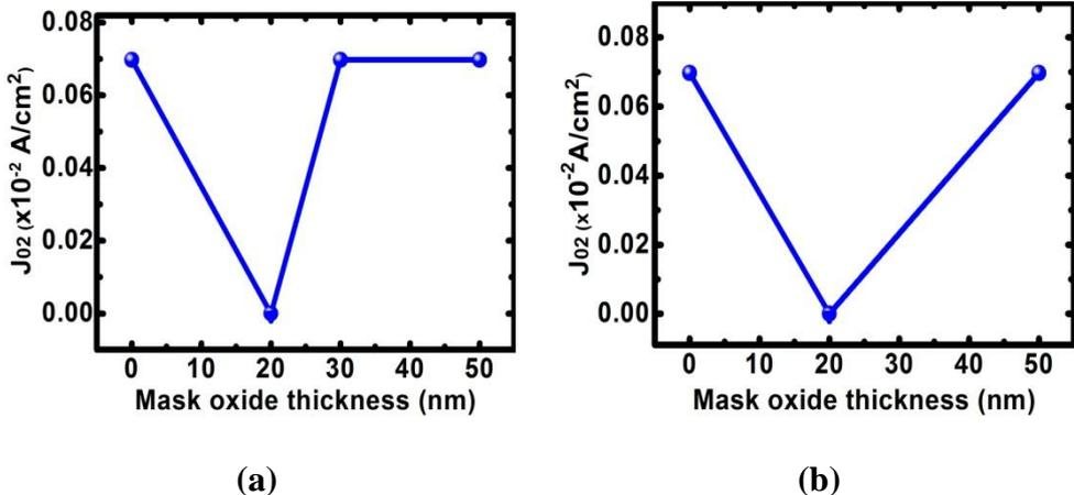
Figure 82: Effect on mask oxide thickness on J<sub>02</sub> (a) with (b) without oxide passivation. Lines are for visual aid
