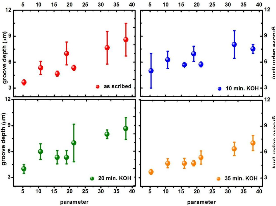
Figure 52: Effect of KOH dipping duration on groove depth
