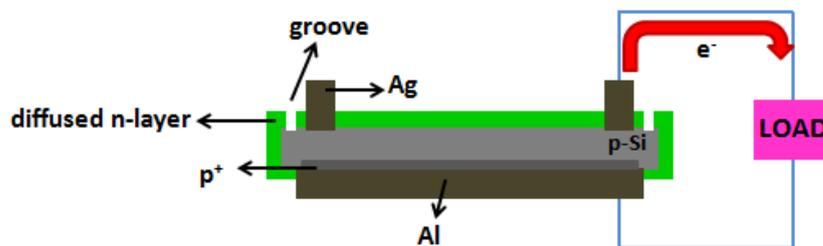
**Figure 30: Operation of a Si solar cell after edge isolation by laser ablation**
