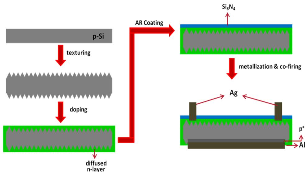
**Figure 28: Fabrication process of standard Si solar cell**
