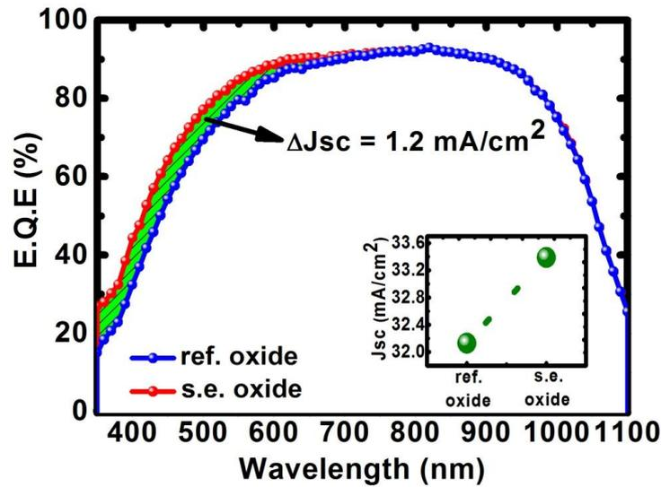
**Figure 98: EQE comparison of oxide passivated reference and selective emitter solar cells with corresponding short circuit current density enhancement**
