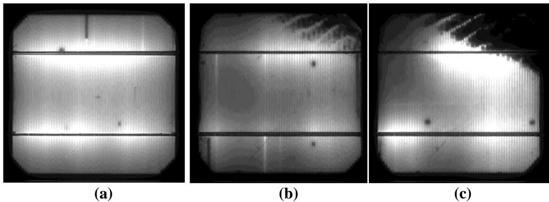
**Figure 58: Electroluminescence images of (a) reference cell, (b) selective emitter with 20 nm oxide mask, (c) selective emitter with 30 nm oxide mask for standard doping**
