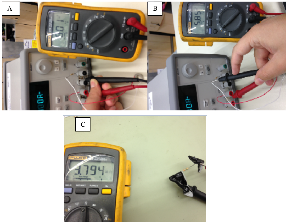
Figure 68. Leakage Resistance Measurement, A- V_{input} Calculation, B- V_{output} Calculation, C- Resistance Measurement Known Resistance.
