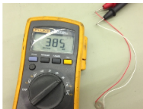
Figure 69. Capacitance Measurement of Piezoelectric Material
