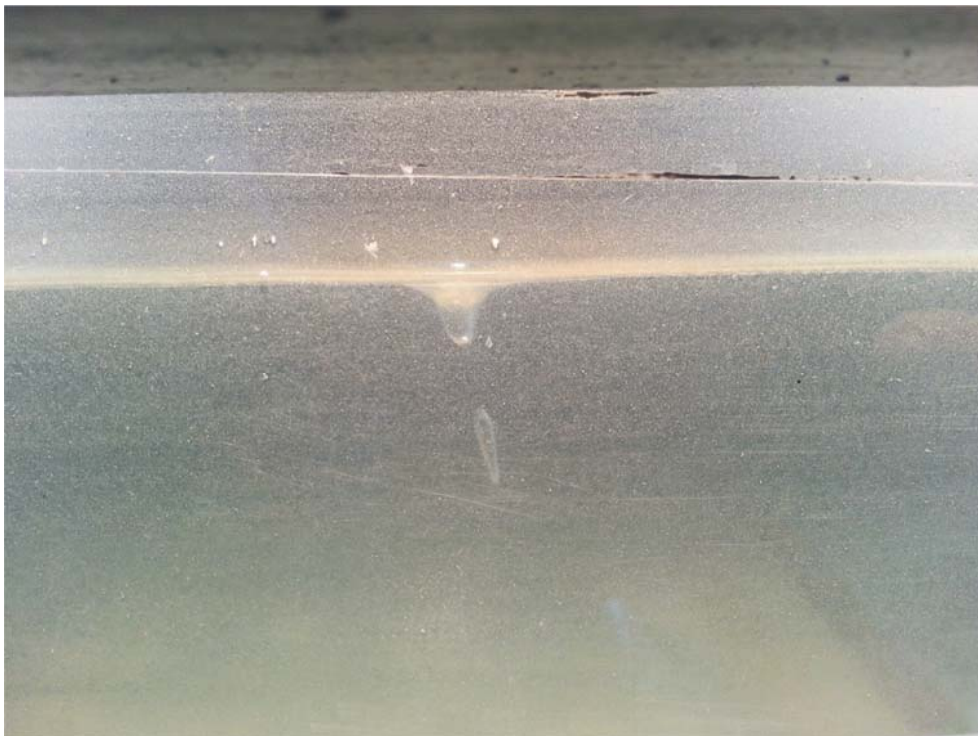
Figure 4.5 Vortex pulling air bubbles to intake
