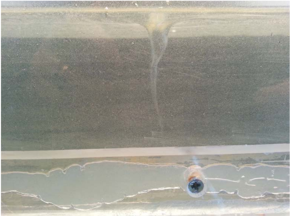
Figure 4.6 A full air core vortex moving towards the intake
