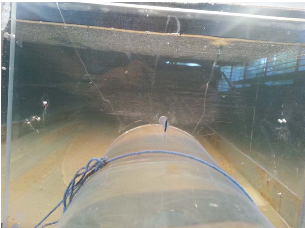
Figure 4.7 Vortex formation away from the centerline of the intake pipe
