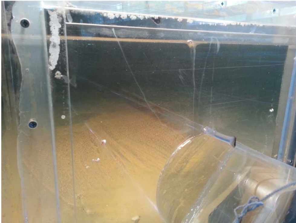
Figure 4.8 Vortex formation around the centerline of the intake pipe
