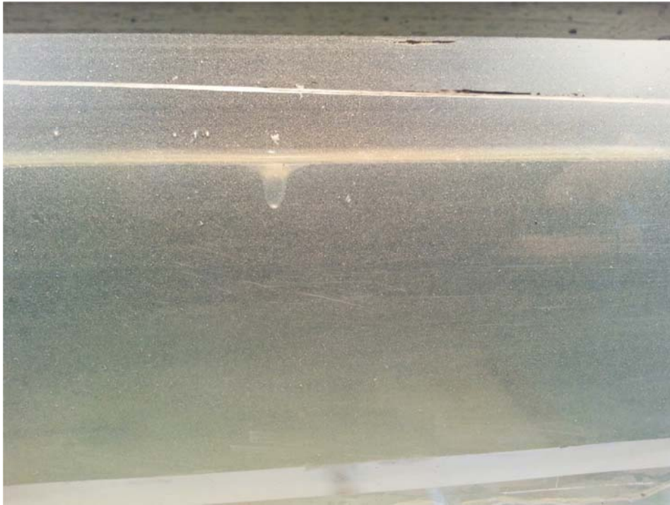
Figure 4.4 Surface dimple formation
