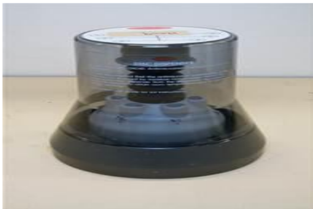
Figure 2.2 Multichannel disc dispenser used for disc diffusion
