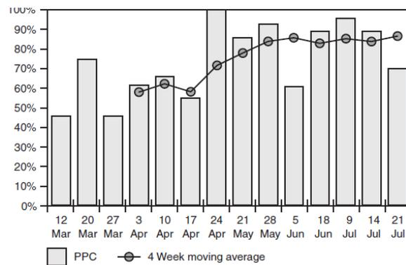
**Figure 3.17:** Example PPC Chart (Ballard et al., 2002)
