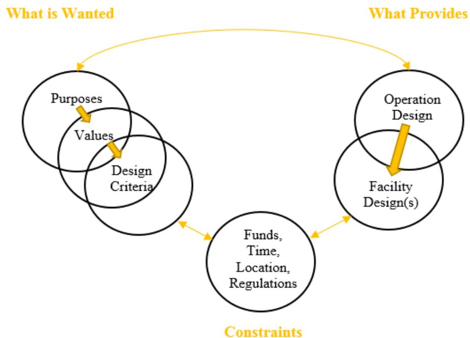
**Figure 3.9:** Project Definition Process (adapted from Ballard, 2008)
