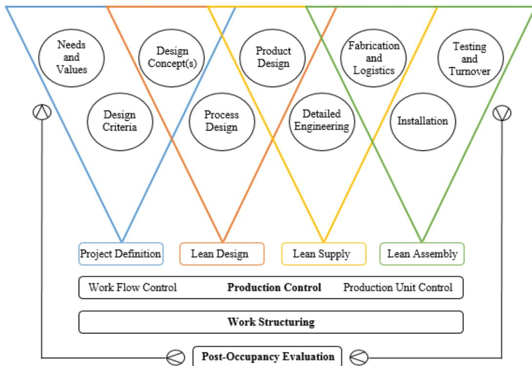
**Figure 3.8:** Triads of the Lean Project Delivery System (adapted from Ballard, 2000a)
