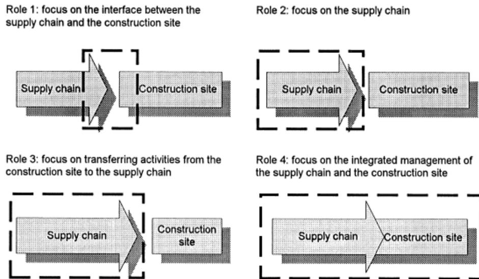
**Figure 3.12:** The Four Roles of SCM in Construction (Vrijhoef and Koskela, 2000)
