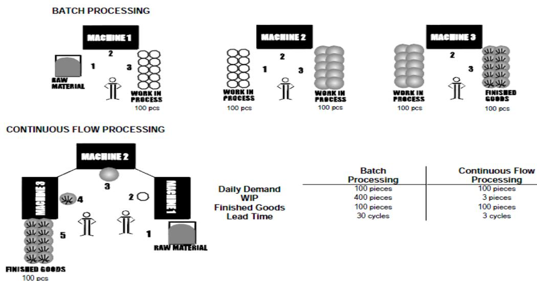
**Figure 2.4:** Continuous Flow Processing vs. Batch Processing (“Art of Lean”)
