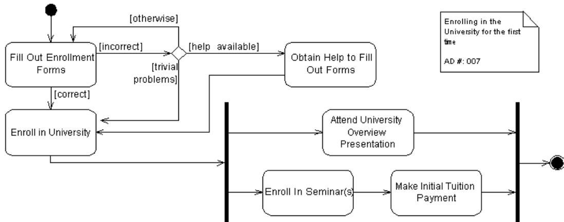
Figure 9 An example UML 2.0 activity diagram [86]
