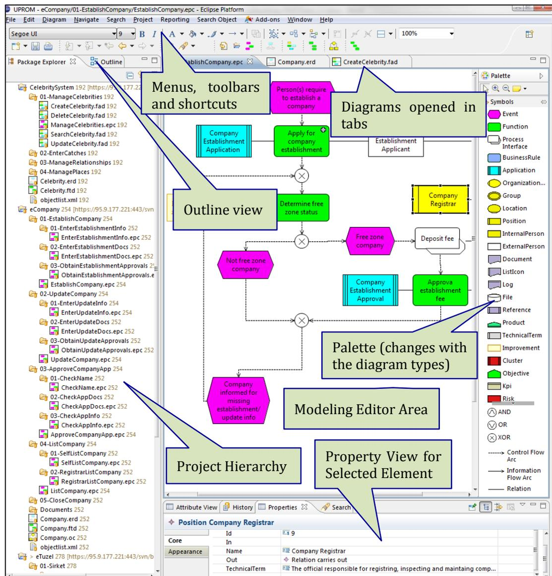
Figure 36 Typical modeling environment for UPROM tool
