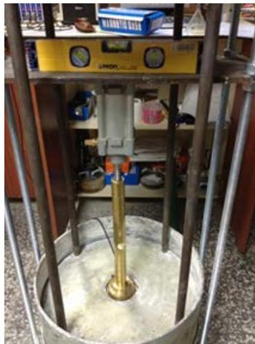
**Figure 3.24. Placing column + double stage foundation plate including the transducer**
