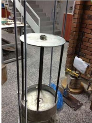
**Figure 3.23. Frame for overburden stress**
