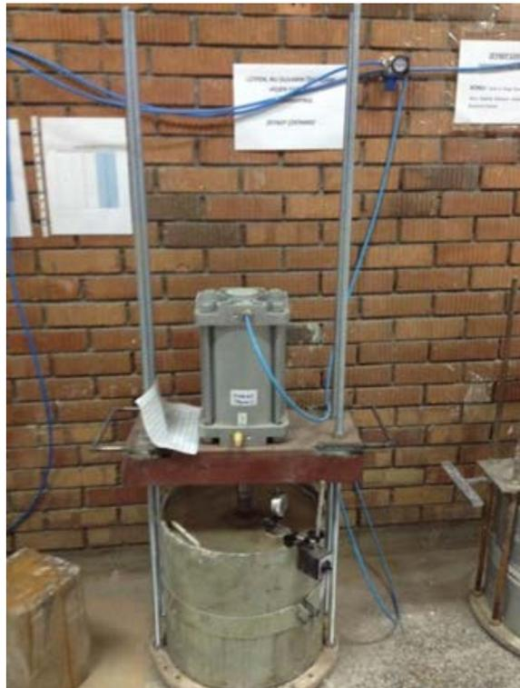
**Figure 3.19. Setup for consolidation phase**
