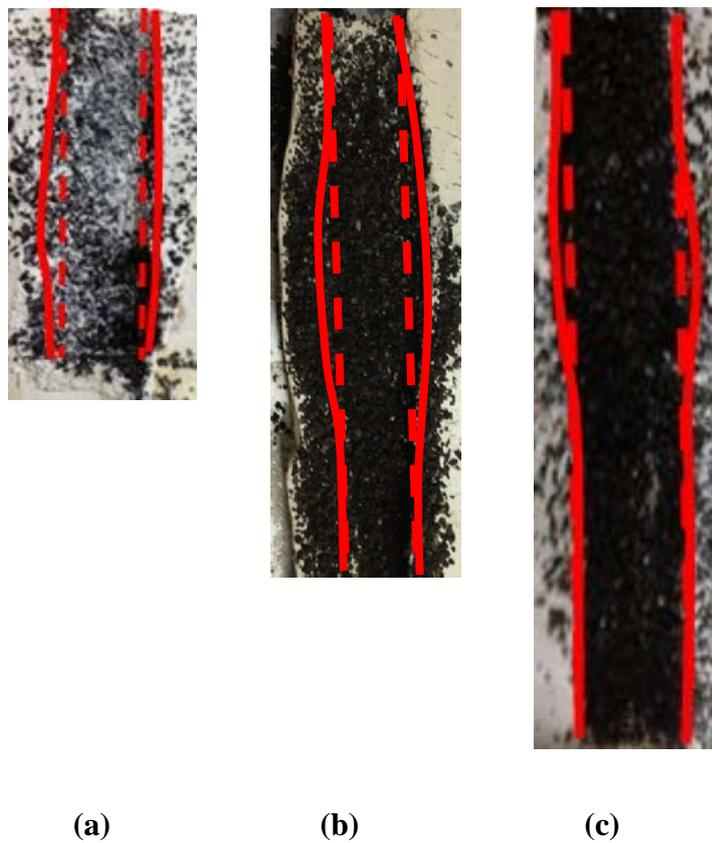
**Figure 5.3. Failure shapes of stone columns (a)  $L/H = 0.4$ , (b)  $L/H = 0.7$  and (c)  $L/H = 1.0$  (Type-S)**
