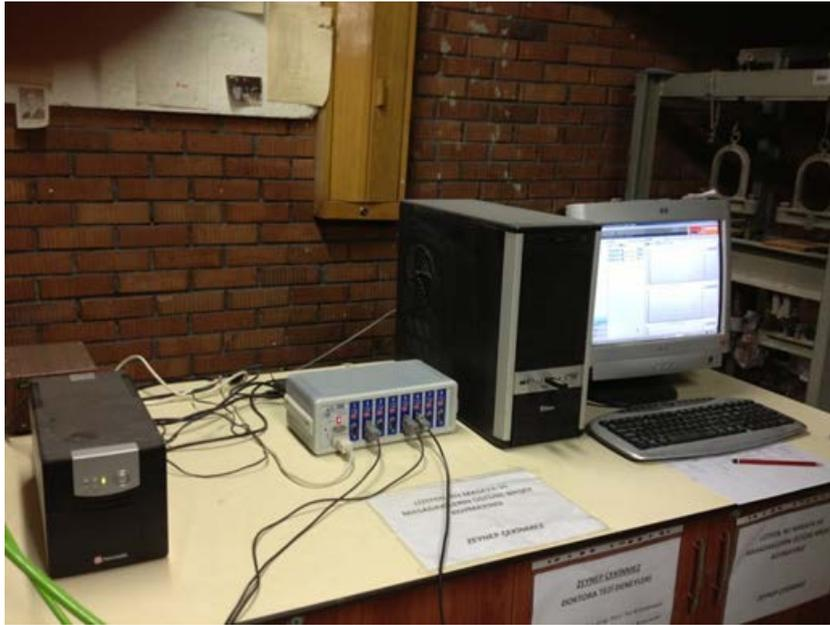
**Figure 3.27. Data acquisition system**
