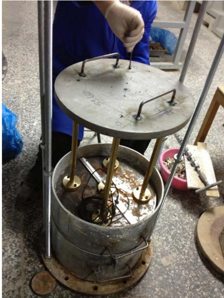
**Figure 3.25. Placing load application frame**
