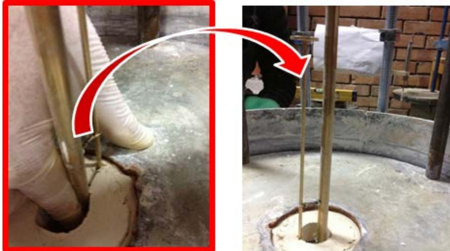
**Figure 3.21. Placement of settlement rod**
