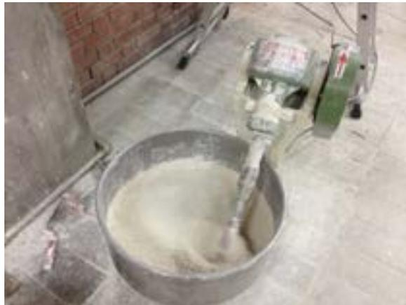
**Figure 3.18. Preparation of paste in large mixer**
