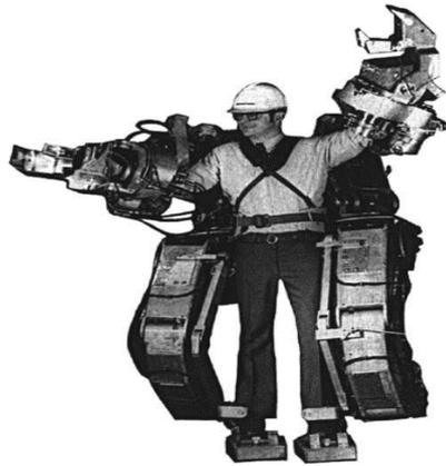
Figure 2.1: Hardiman Exoskeleton (Corliss, et. al.,1968)
