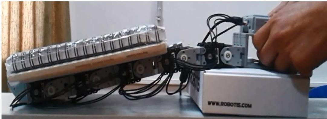
Figure 5.3: Exoskeleton with 1kg load
