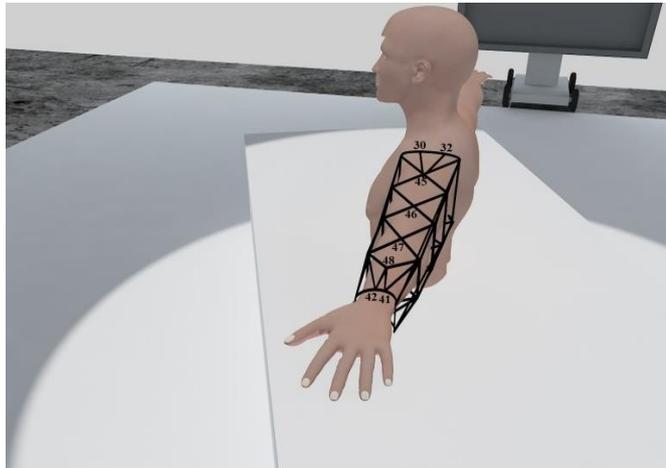
Figure 3.1: The Meshed Exoskeleton Structure That Enwraps Arm
