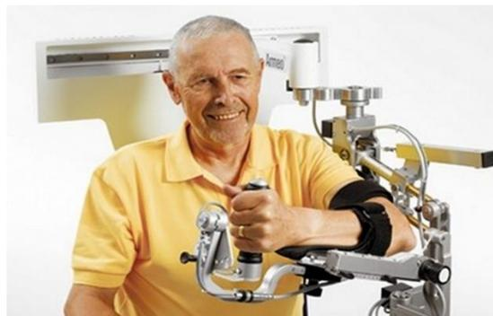
Figure 2.6: T-Wrex Exoskeleton (Sanchez et. al.,2006)
