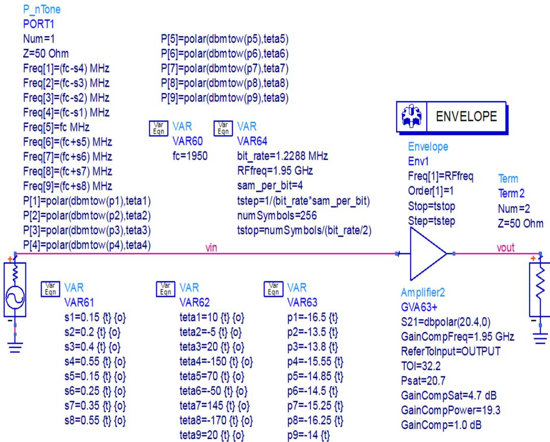
Figure 4-25 9-tone model schematic prepared in ADS
