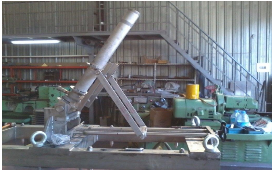
Figure 3.32: The manufactured adjustable ejector
