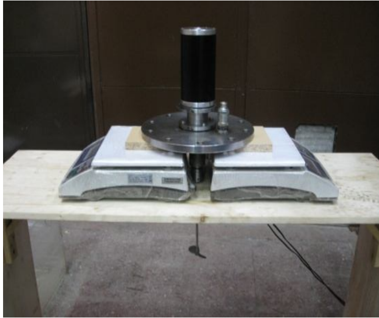
Figure 3.5: The tank test setup for measuring thrust force
