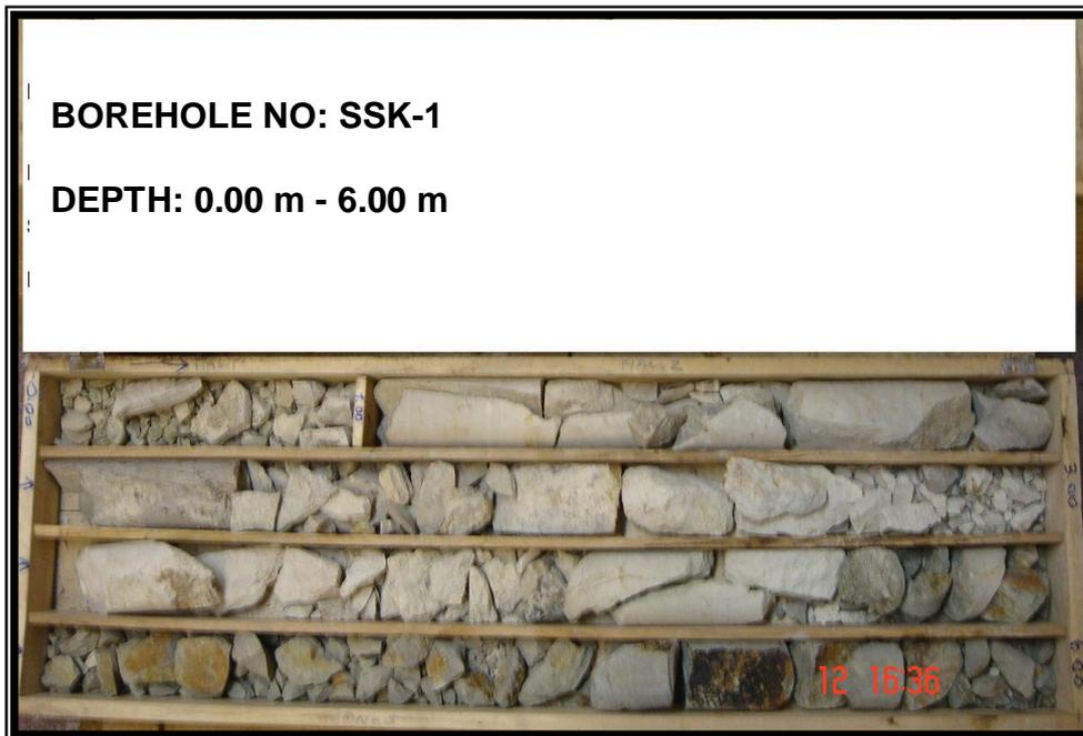
Figure 3.9. A sample picture for the SSK-1 borehole cores.
