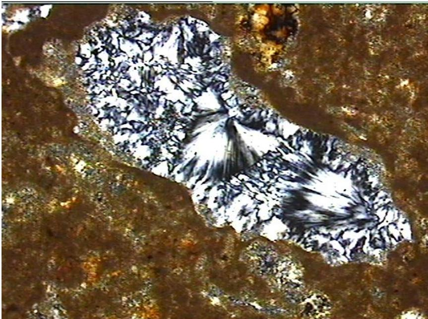
Figure 4.17. Photomicrograph of chalcedone mineral as infilling (HAN-19, XPL, 4x 10 ).
