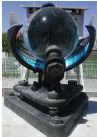
Figure 1.1. Campbell-Stokes recorder (Taken from TSMS web site)
