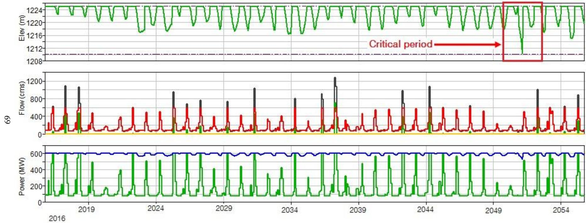
Figure 4.15 40 years time series simulation period operating cycle for Upper Kaleköy Dam and HEPP in Scenario 3
