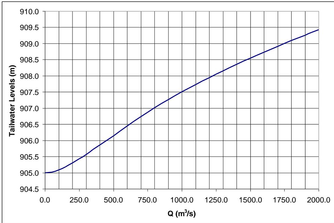
Figure 3.23 Tailwater rating curve for the dam site of Beyhan 1
