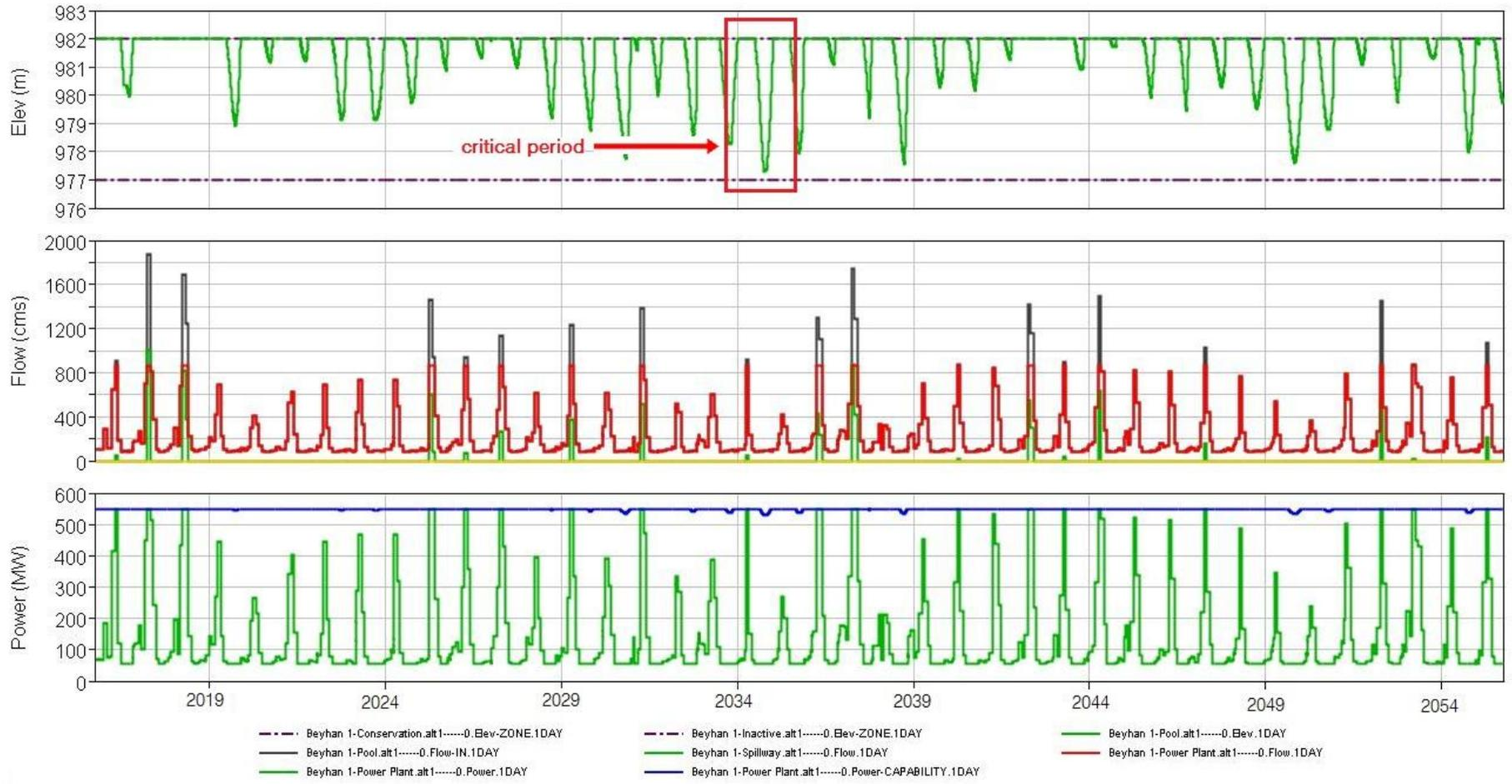
Figure 4.18 40 years time series simulation period operating cycle for Beyhan 1 Dam and HEPP in Scenario 3
