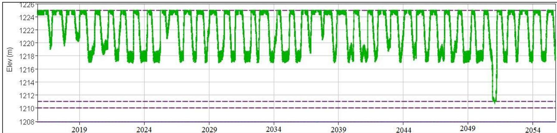
Figure 4.38 40 years long time series simulation period operating cycle for Upper Kaleköy Dam and HEPP in Scenario 8
