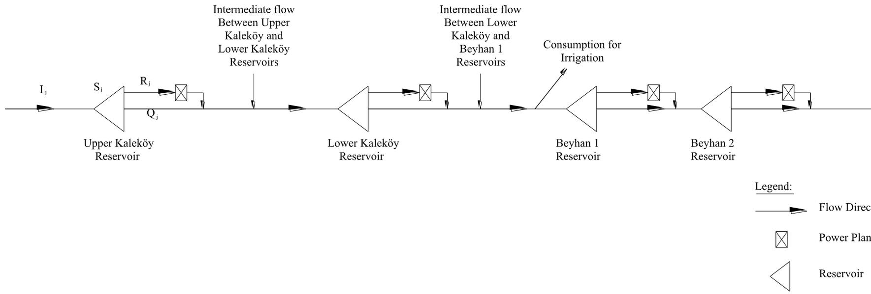
Figure 3.3 Schematic diagram of Kaleköy reservoir system
