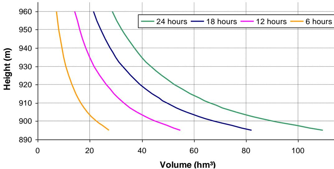
Figure 4.4 Beyhan 2 reservoir storage required vs. height for 255 MW plant with 6, 12, 18 and 24 hours of operation
