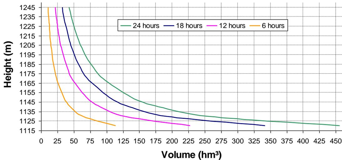
Figure 4.1 Upper Kaleköy reservoir storage required vs. height for 600 MW plant with 6, 12, 18 and 24 hours of operation
