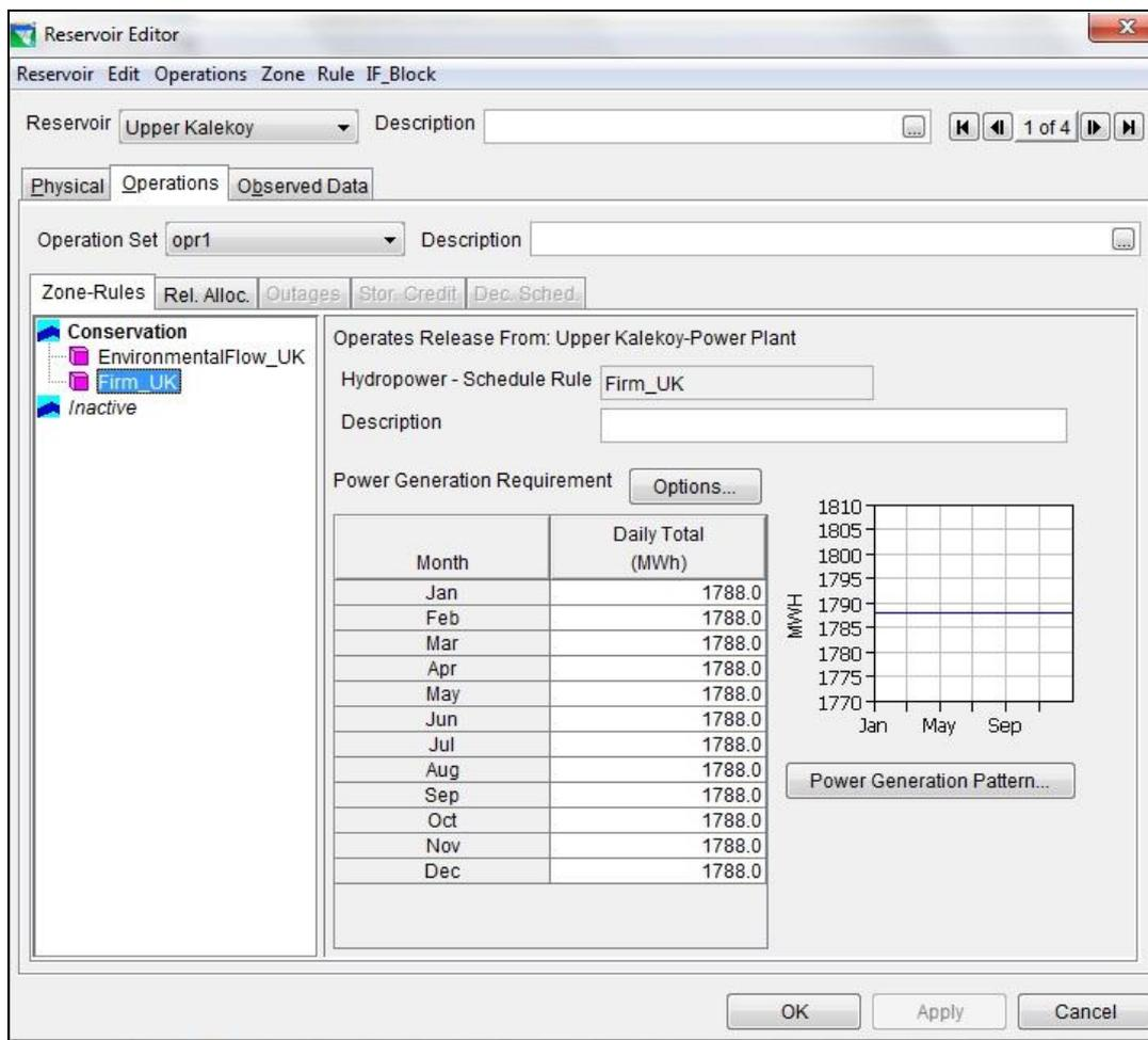
Figure 4.13 Application of firm power generation requirement rule
