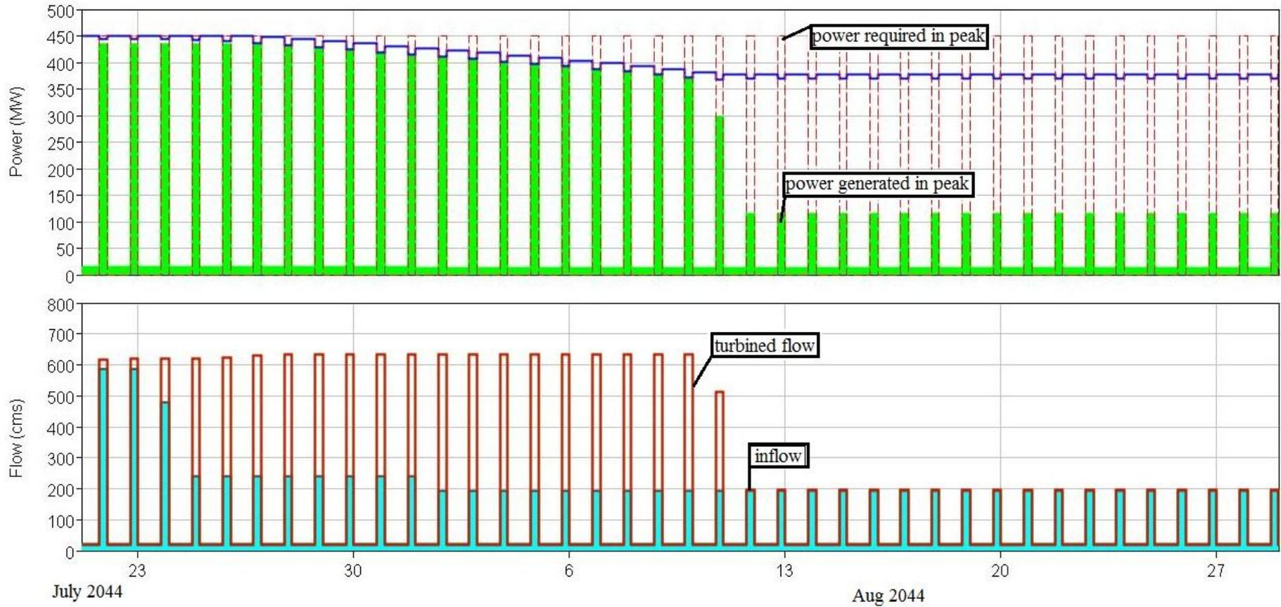
Figure 4.29 Peak power generation operation cycle for Lower Kaleköy Dam and HEPP in Scenario 7
