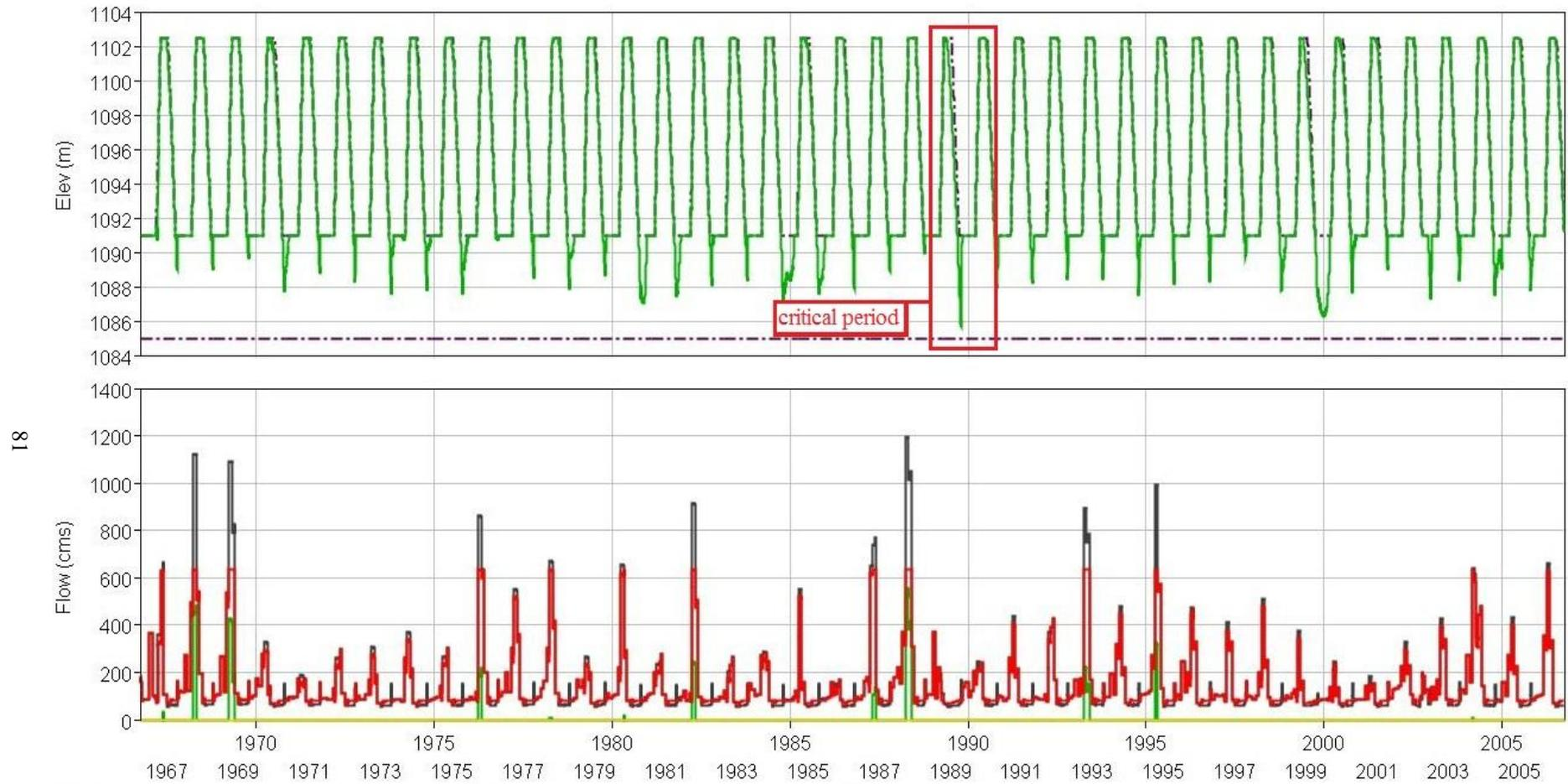
Figure 4.27 40 years time series simulation period operating cycle for Lower Kaleköy Dam and HEPP in Scenario 6
