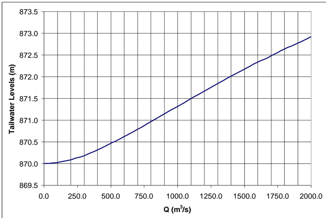
Figure 3.24 Tailwater rating curve for the dam site of Beyhan 2
