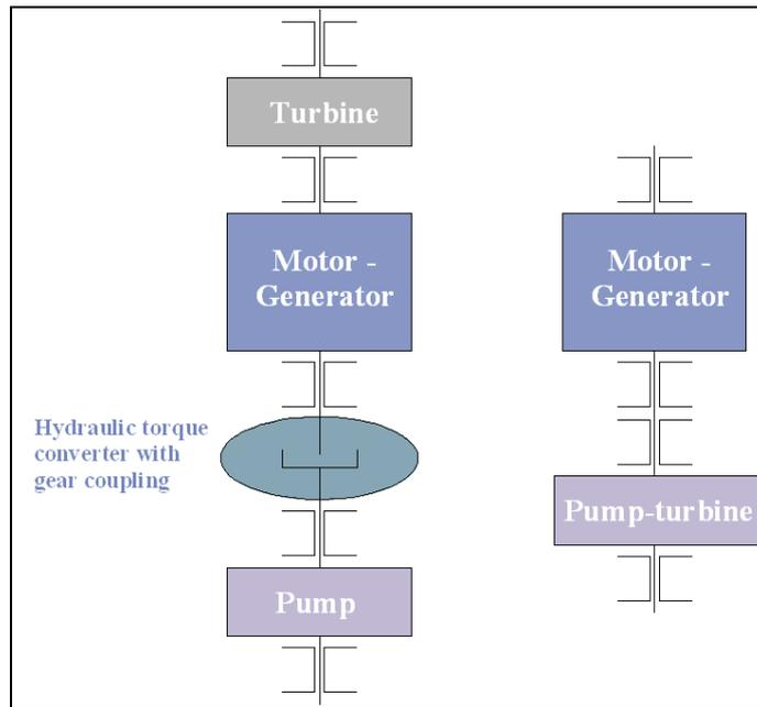
Figure 2.11 Types of pumped turbines (Voith, 2009)
