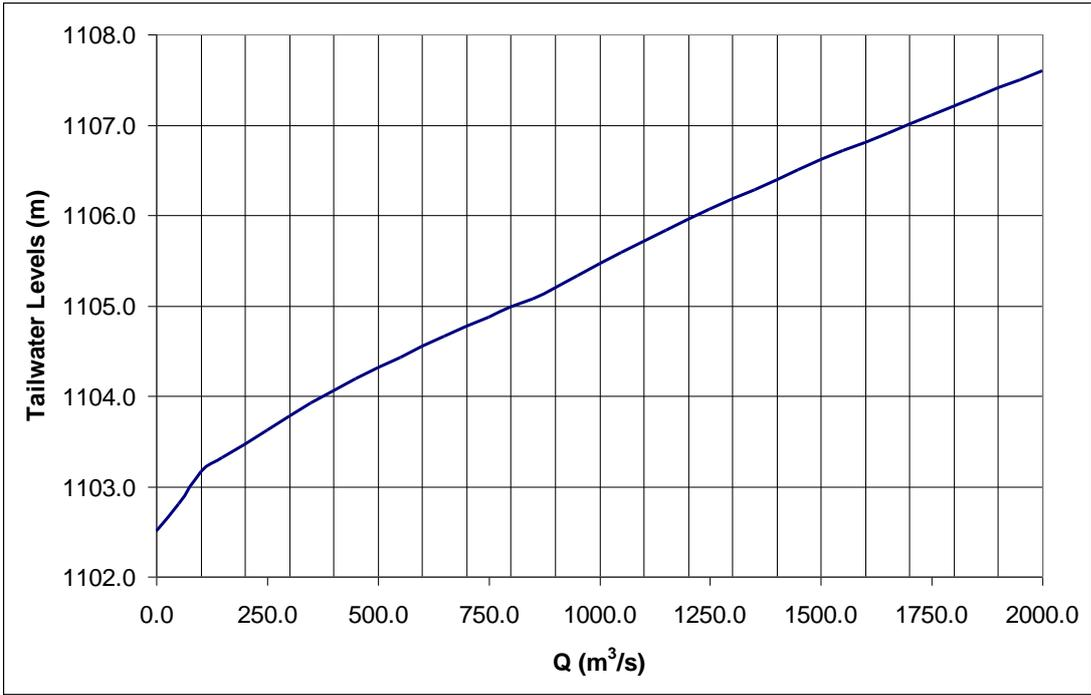
Figure 3.21 Tailwater rating curve for the dam site of Upper Kaleköy
