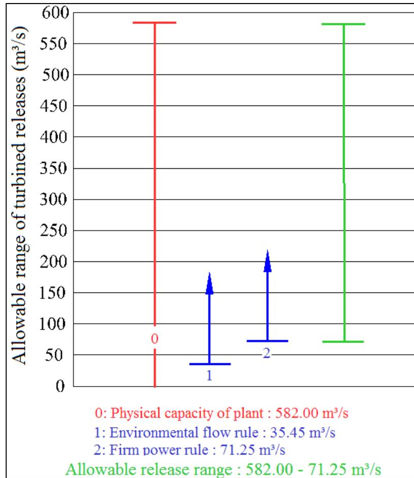
Figure 4.14 Allowable turbined release range of Upper Kaleköy in Scenario 3
