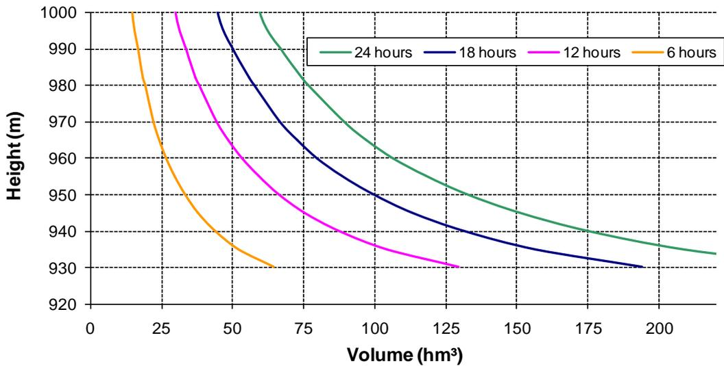
Figure 4.3 Beyhan 1 reservoir storage required vs. height for 550 MW plant with 6, 12, 18 and 24 hours of operation
