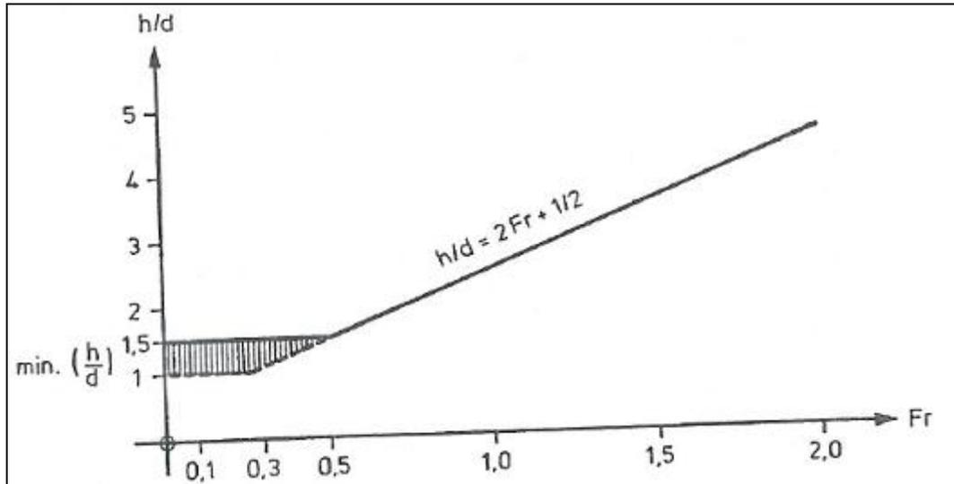
Figure 3.16 Recommended submergence for intakes (ASCE, 1995)
