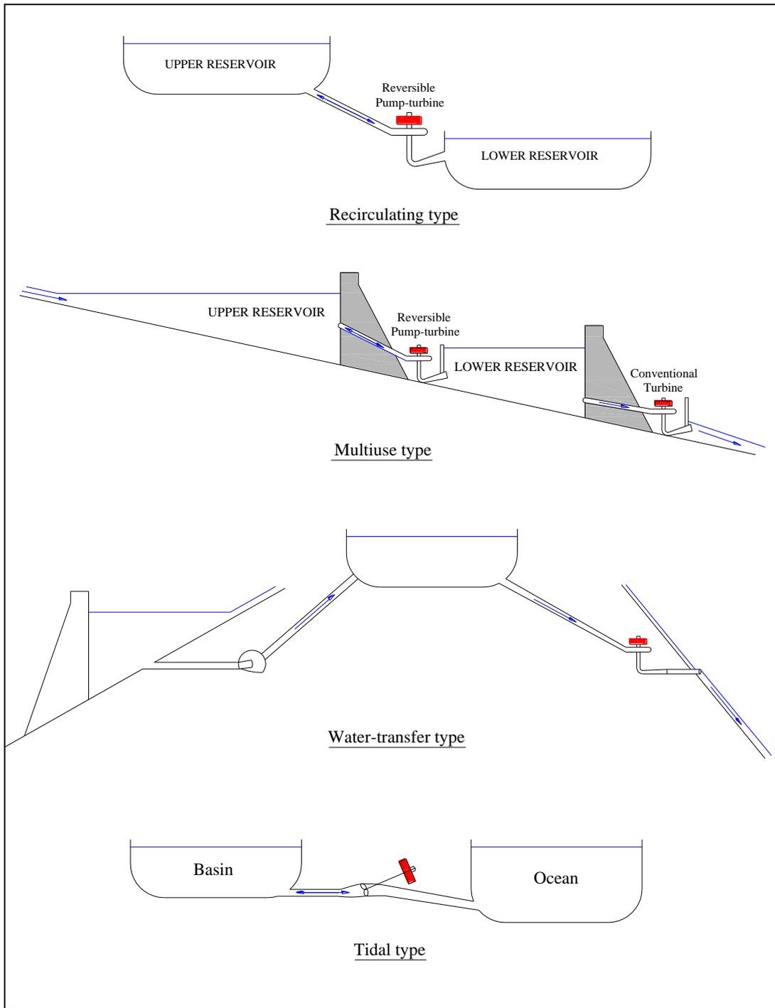
Figure 2.12 Types of pumped storages development (Voith, 2009)
