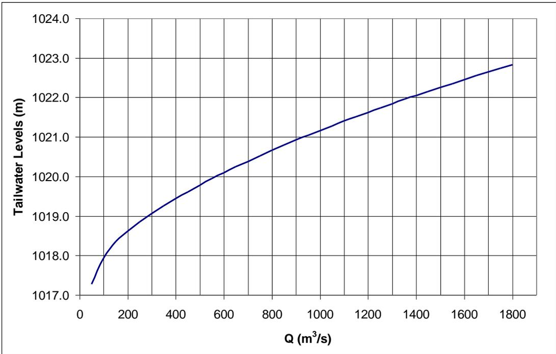
Figure 3.22 Tailwater rating curve for the dam site of Lower Kaleköy
