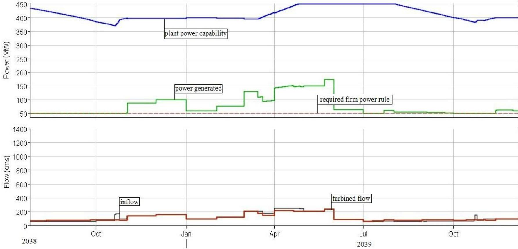
Figure 4.28 A closer look to the power plot for the critical period operating cycle for Lower Kaleköy Dam and HEPP in Scenario 6
