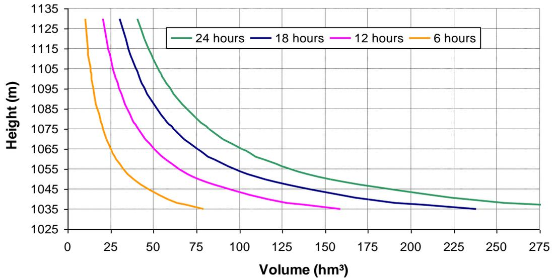
Figure 4.2 Lower Kaleköy reservoir storage required vs. height for 450 MW plant with 6, 12, 18 and 24 hours of operation
