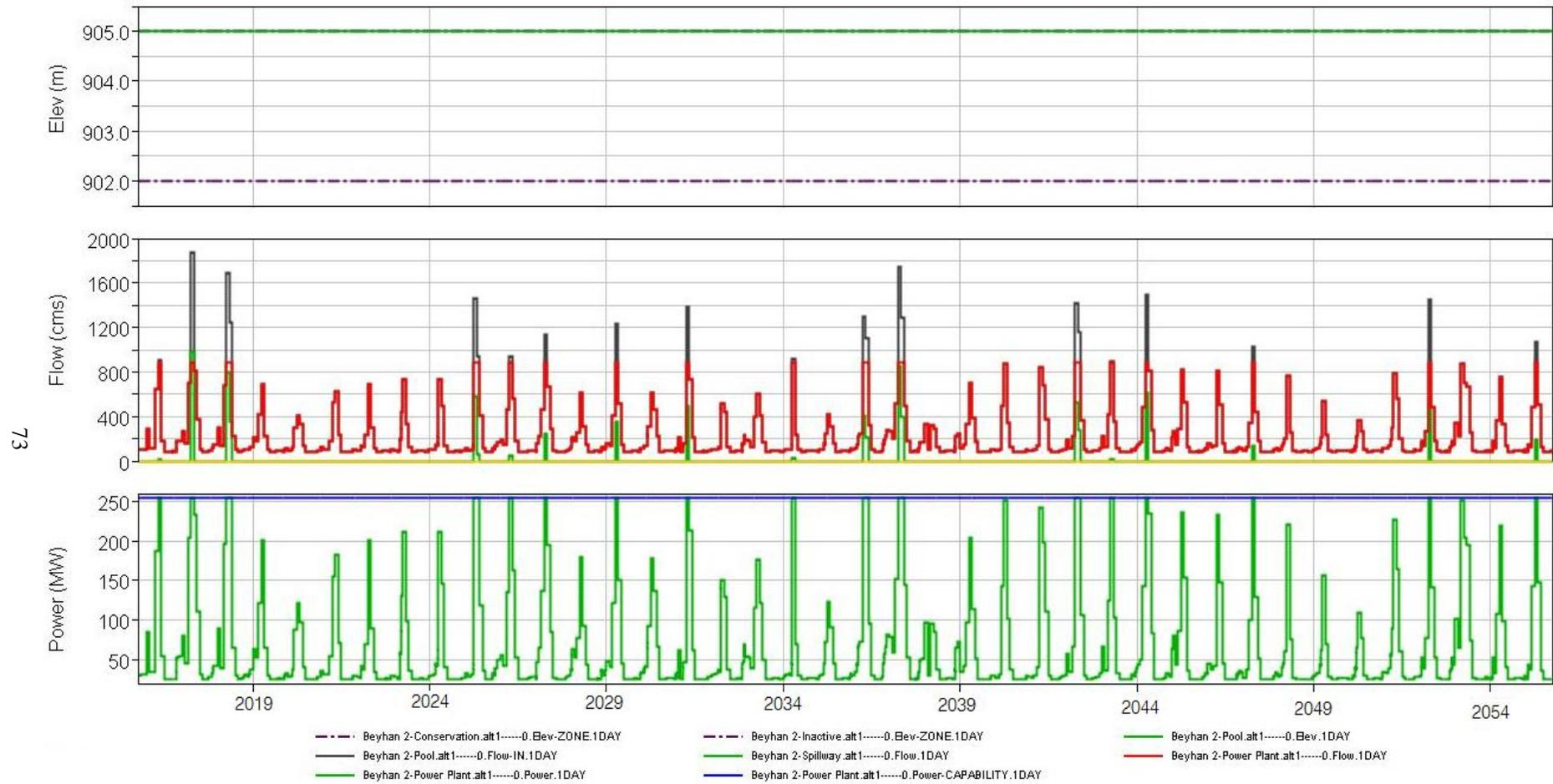
Figure 4.19 40 years time series simulation period operating cycle for Beyhan 2 Dam and HEPP in Scenario 3
