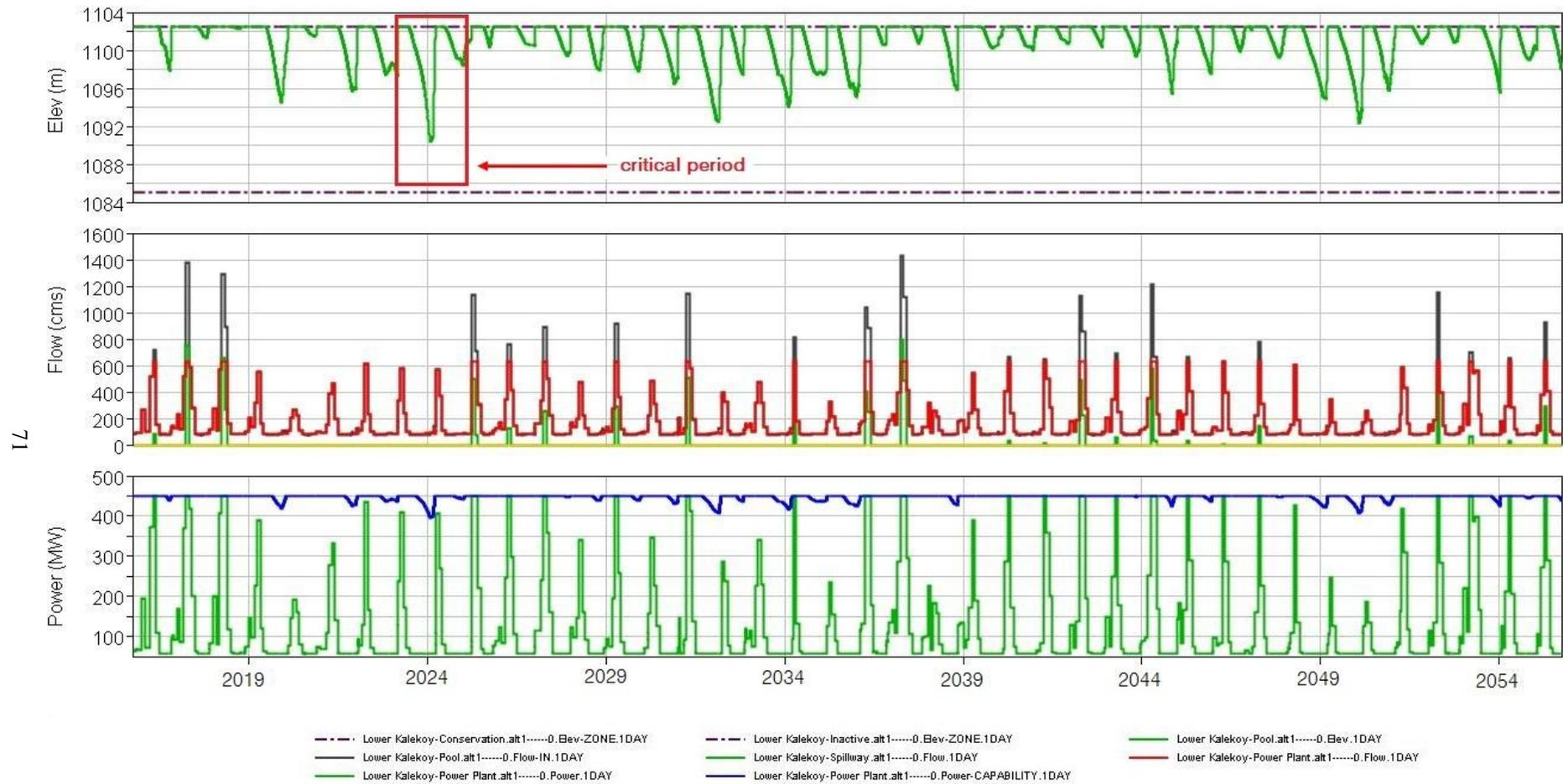
Figure 4.17 40 years time series simulation period operating cycle for Lower Kaleköy Dam and HEPP in Scenario 3
