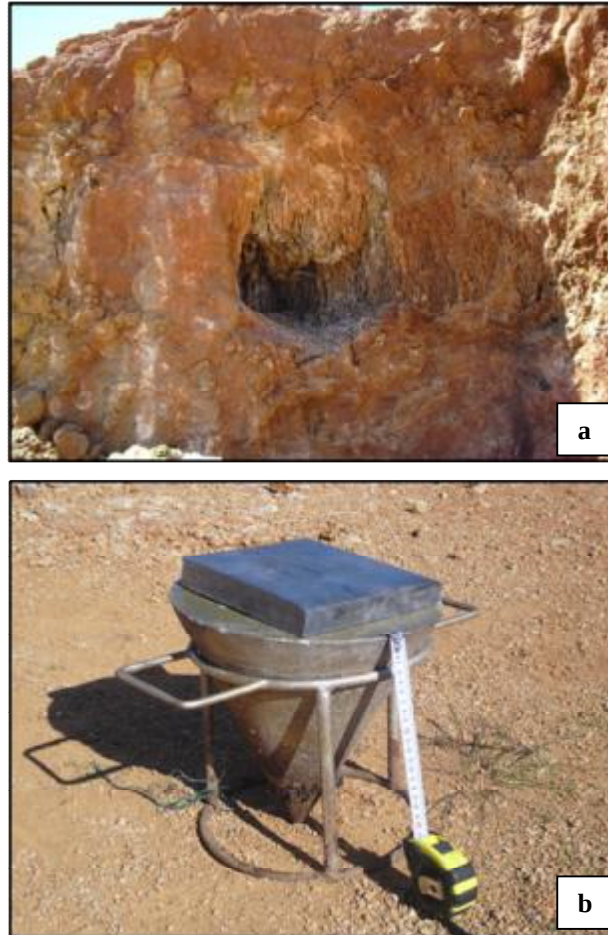
Figure 37. a) A view of a cavity which was attempted with the SRT method. b) The fabricated lead plate used during SRT measurements.
