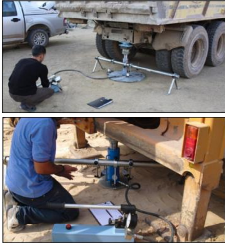
Figure 52. Views of plate load tests performed with 300 mm and 762 mm diameter plates.
