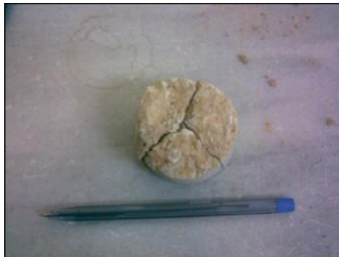
Figure 32. A view of the point load strength test.
