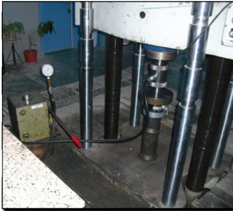
Figure 30. A view of the triaxial compressive strength test.
