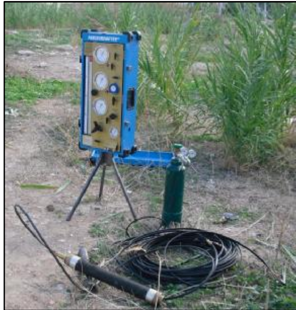
Figure 49. Menard type pressuremeter instrument utilized during testing
