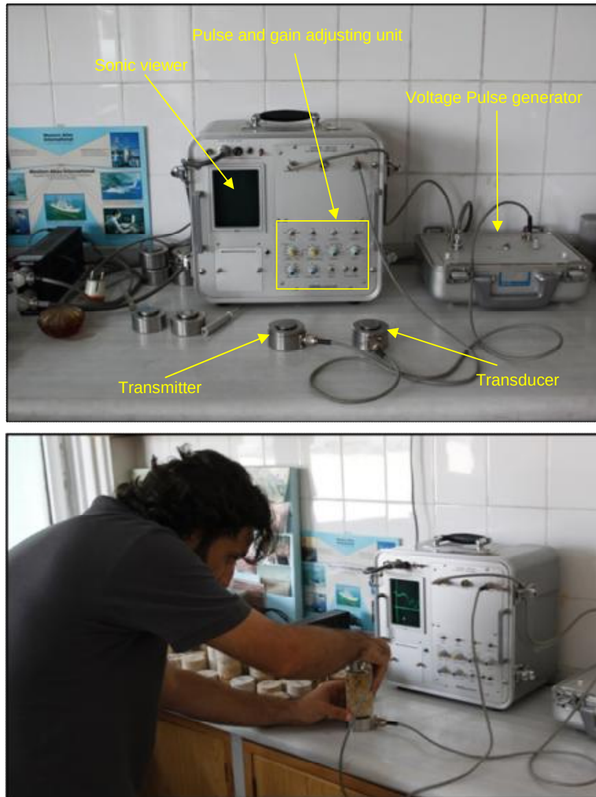
Figure 28. Views from the ultrasonic velocity measurement device and during testing.
