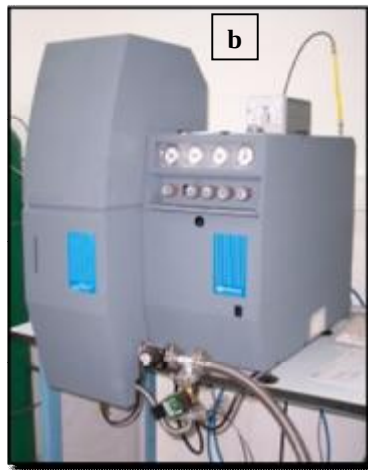
Figure 27. a) JSM 6400 NORAN System 6 X-ray Microanalysis System and Semafore Digitizer device used for SEM analyses. b) Setaram Labsys Simultaneous DTA/TGA device c) Ceramic inner liner oven for LOI analyses.
