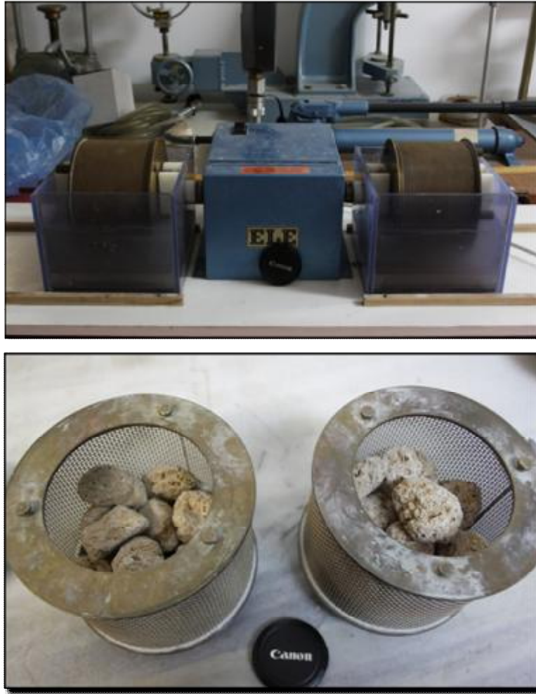
Figure 33. A View of the slake durability test.
