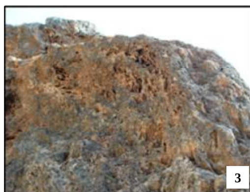
Figure 21. A typical view of tufa rock outcrop displaying quite a wide variation of pore size (October, 2007).
