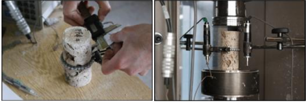
Figure 34. A circumferential extensometer used for the measurement of the elastic parameters of the tufa samples.
