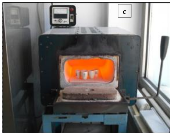
Figure 27. a) JSM 6400 NORAN System 6 X-ray Microanalysis System and Semafore Digitizer device used for SEM analyses. b) Setaram Labsys Simultaneous DTA/TGA device c) Ceramic inner liner oven for LOI analyses.
