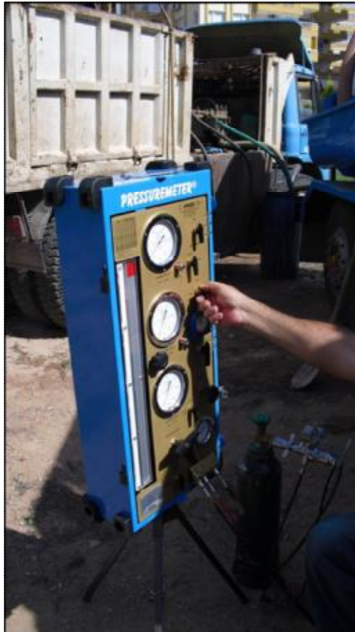
Figure 25. A view from a pressuremeter test carried out simultaneously during borehole drilling (October, 2010).
