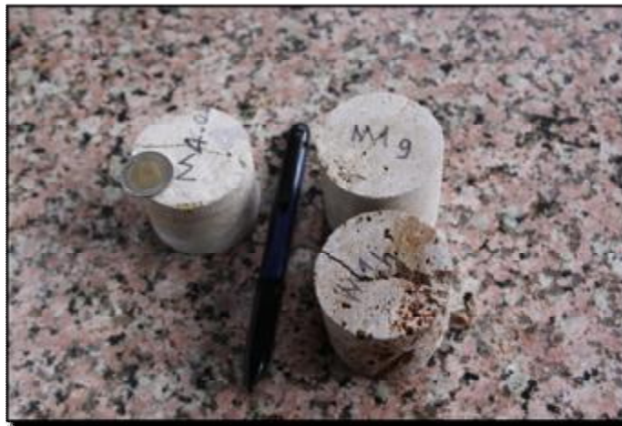
Figure 31. A view of the Brazilian indirect tensile strength test.
