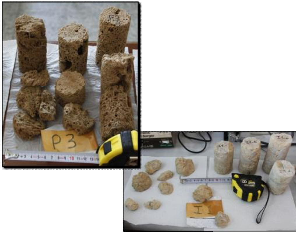
Figure 48. The fragile tufa rock masses which are hard to core in order to obtain representative core samples for laboratory testing.
