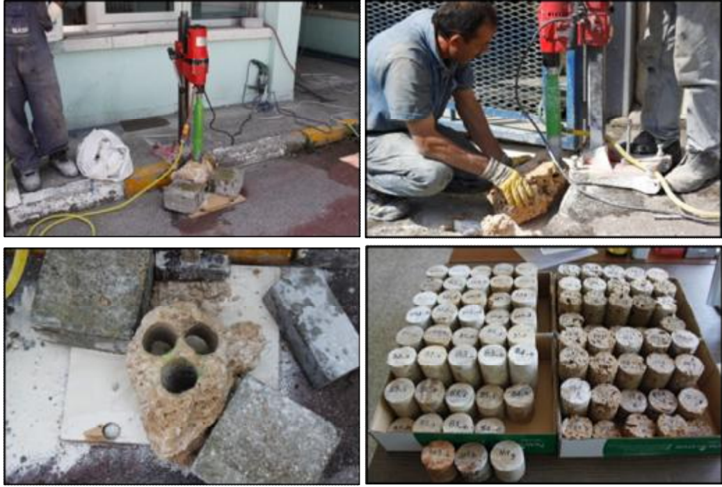
Figure 20. Views from the core sample preparation from the block samples of the Antalya tufa rock masses (July, 2010).
