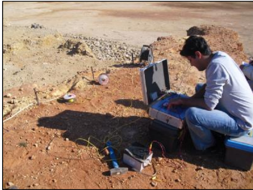
Figure 40. The resistivity measuring device utilized during the investigations.
