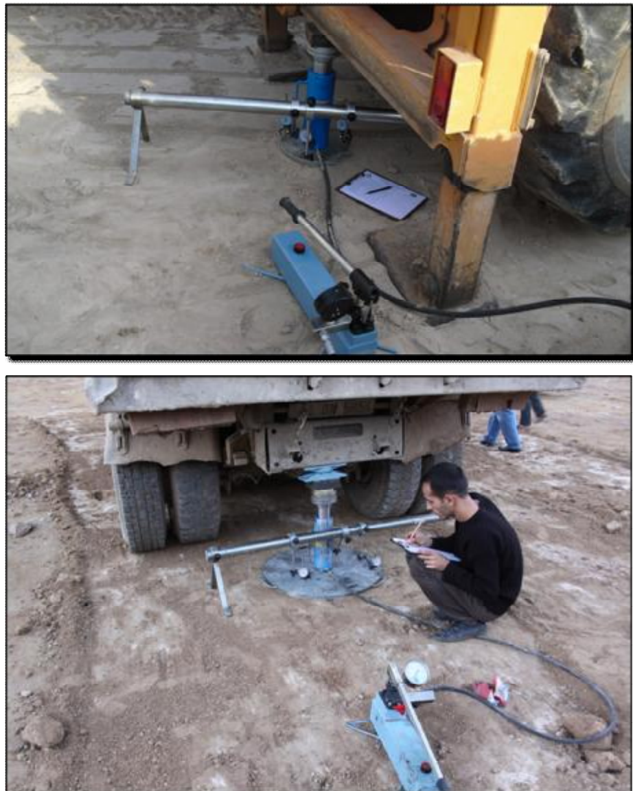
Figure 26. Views from plate load tests (January, 2011).
