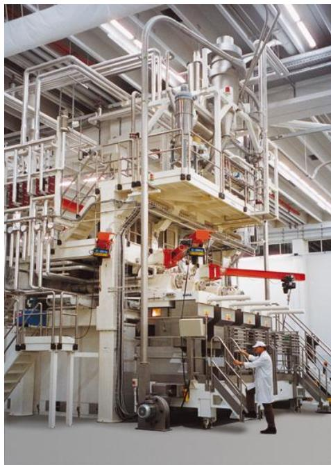
**Figure 3** Latest technology pasta production line (Source: FAVA)
