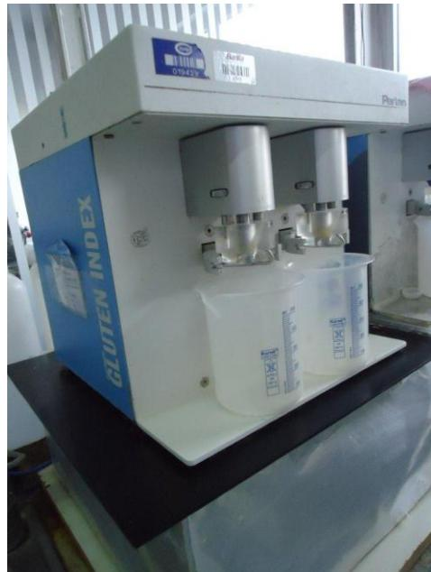
**Figure 7** Perten Glutomatic 2200 – Gluten Index-(ICC)
