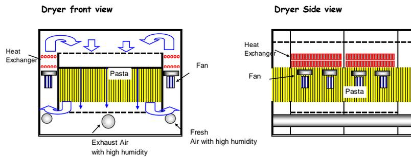
**Figure 4** Drying process of pasta (Source: Barilla)
