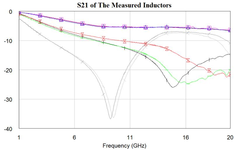
Figure 4-19. dB(S21) responses of the measured inductors with SOLT calibration and without de-embedding.
