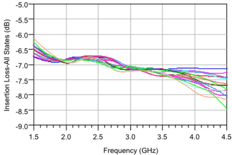
Figure 5-32. The overall performance of 2 to 4 GHz for all 16 phase shift states and the reference state  $S_{21}$  plots (Insertion losses).
