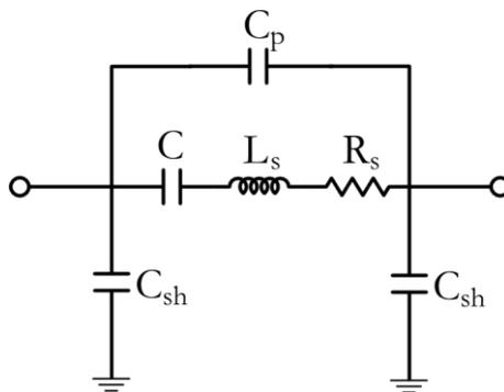
Figure 4-29. Illustration of lumped equivalent model of MIM capacitors, for alumina and/or quartz substrates.
