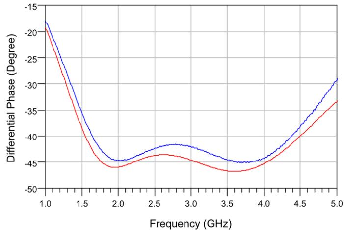
Figure 6-15. Differential phase response of 2-4 GHz 45° M phase shift bit measurement in comparison with practical design (red line represents the practical design and blue line represents the measurement result).
