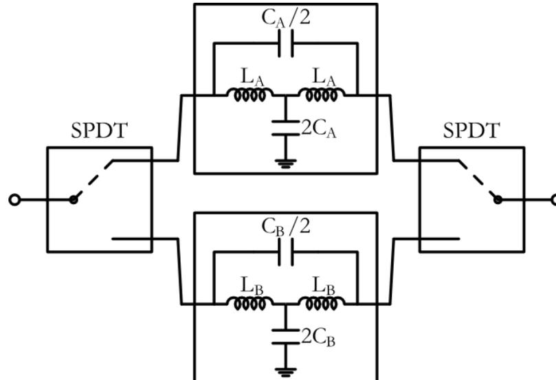
Figure 3-4. An illustration of One-Stage All-pass Phase Shift bit with series-C configuration.
