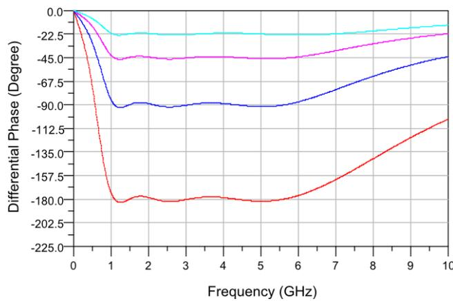
Figure 3-28. Ideal differential phase characteristics of three-stage, four-bit, 1 to 6 GHz phase shifter.
