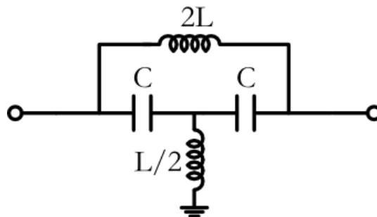
Figure 3-1. All pass network with series-L configuration
