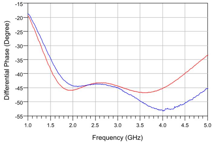
Figure 6-16. Differential phase response of 2-4 GHz 45° DCF phase shift bit measurement in comparison with practical design (red line represents the practical design and blue line represents the measurement result).
