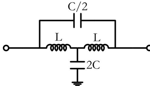
Figure 3-2. All pass network with series-C configuration
