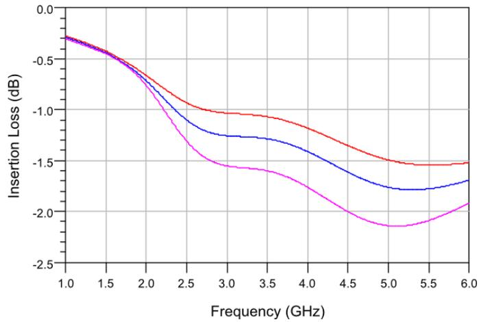
Figure 5-45. Insertion loss graphs of 5.625° and 11.25° practically constructed phase shifter; reference state (blue line), 5.625° phase shift state (red line), and 11.25° phase shift state (pink line).
