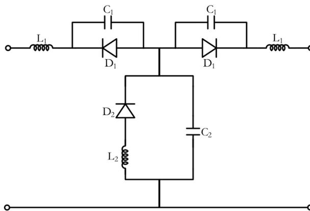
Figure 2-8. The proposed phase shifter circuit with three diodes.
