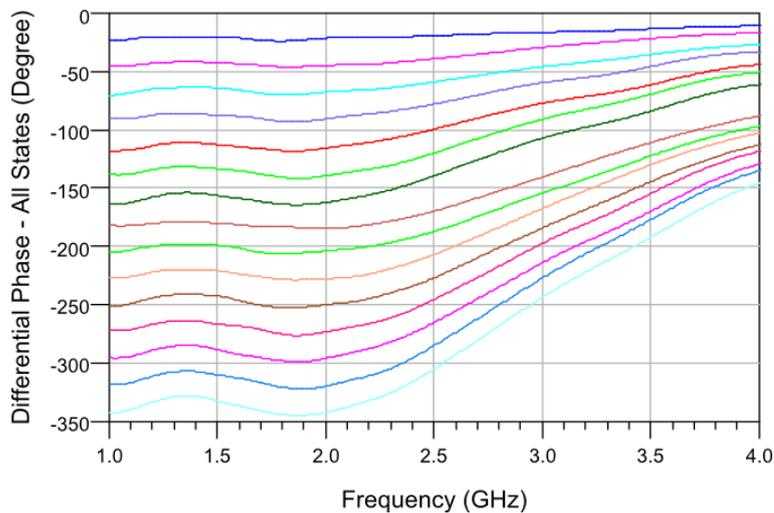
Figure 5-29. The overall differential phase shift performance of 1 to 2 GHz phase shifter for all 15 phase shift states with respect to reference phase shift state.
