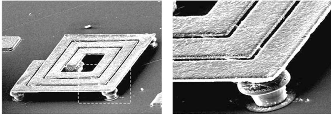
Figure 4-3. SEM image of a suspended inductor with T-shape pillar (zoomed in version on the right) [52].
