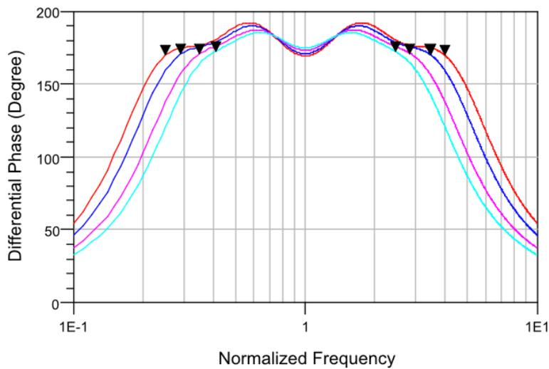
Figure 3-18. Differential phase shift plots for 180° bit four-stage for bandwidths of 6:1 (turquoise line), 8:1 (pink line), 12:1 (blue line), and 16:1 (red line).
