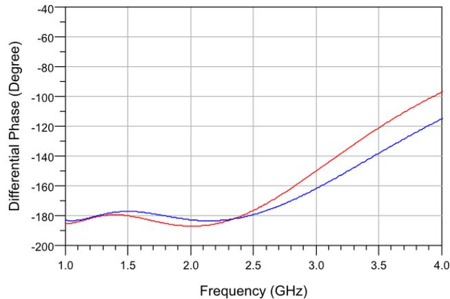
Figure 5-6. The differential phase shift response of 1 to 2 GHz phase shifter 180° phase shift bit configuration # 1 with iterated shunt MIM capacitors and added Tee junctions (red line represents the present case, and blue line represents the ideal case).
