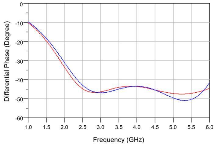
Figure 6-18. Differential phase response of 3-6 GHz 45° DCM phase shift bit measurement in comparison with practical design (red line represents the practical design and blue line represents the measurement result).
