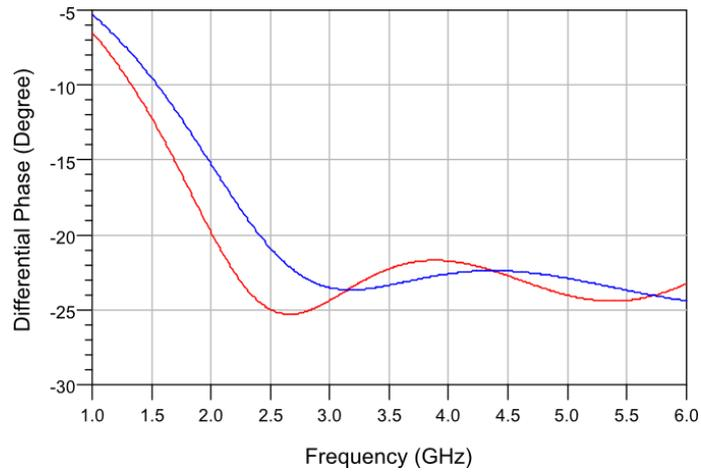
Figure B-14. The differential phase shift response of 3 to 6 GHz phase shifter 22.5° phase shift bit layout considered, and iterated shunt MIM capacitors (red line represents the present case, and blue line represents the ideal case).
