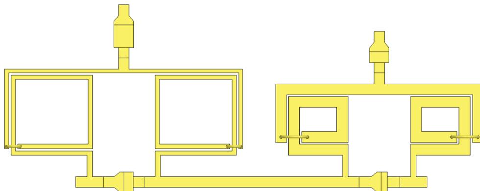
Figure A-7. Upper branch of 2 to 4 GHz phase shifter 90° phase shift bit (Length: 4.351 mm, Width: 1.741 mm, Separation between inductors: 300 μm).
