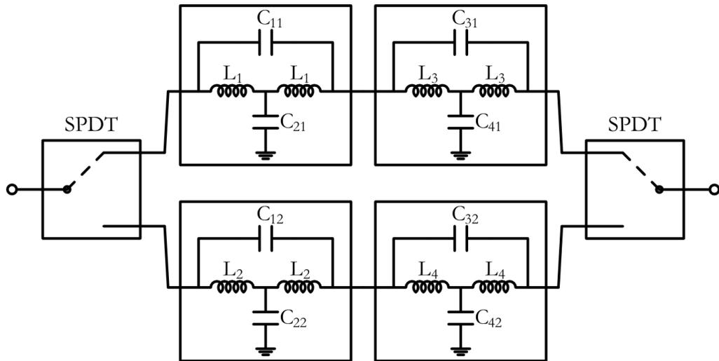
Figure 3-7. An illustration of a Two-Stage All-pass Phase Shift bit with series-C configuration.
