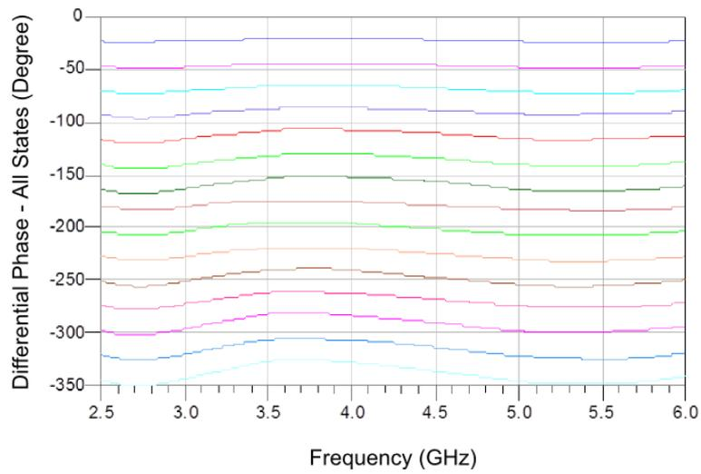
Figure 5-37. The overall differential phase shift performance of 3 to 6 GHz phase shifter for all 15 phase shift states with respect to reference phase shift state.
