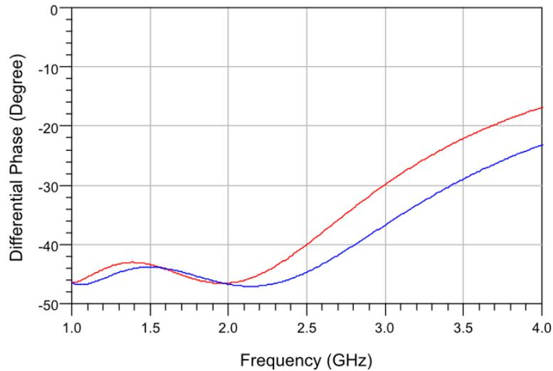
Figure 5-20. The differential phase shift response of 1 to 2 GHz phase shifter 45° phase shift bit configuration # layout considered, and iterated shunt MIM capacitors (red line represents the present case, and blue line represents the ideal case).
