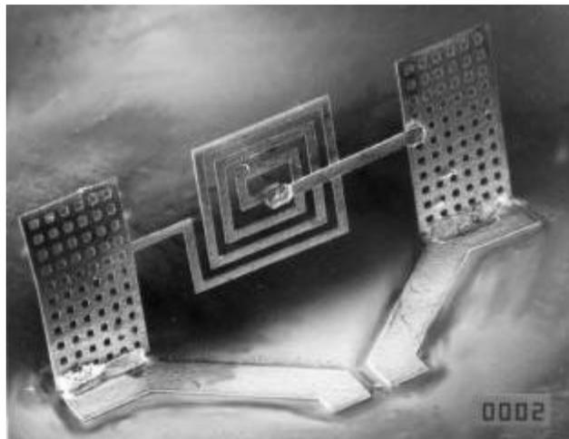
Figure 4-5. SEM image of a self-assembled inductor [62].
