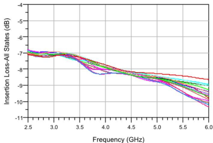
Figure 5-36. The overall performance of 3 to 6 GHz for all 16 phase shift states and the reference state  $S_{21}$  plots (Insertion losses).
