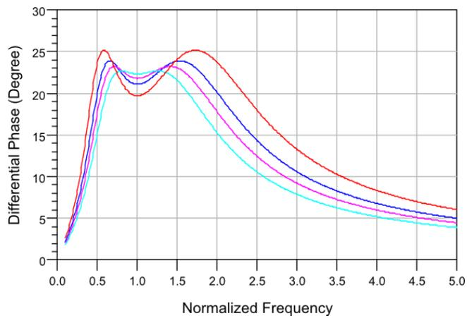
Figure 3-10. Differential phase shift plots for 22.5° bit two-stage for bandwidths of 2:1 (turquoise line), 3:1 (pink line), 4:1 (blue line), and 6:1 (red line).
