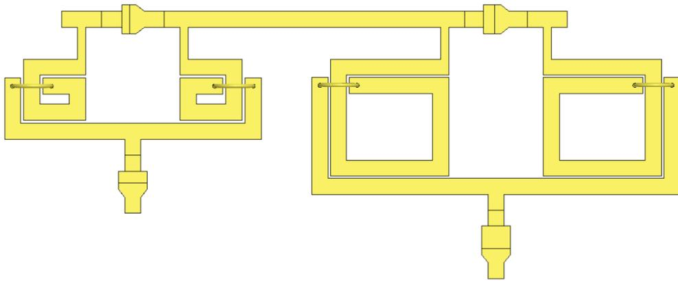
Figure A-4. Lower branch of 2 to 4 GHz phase shifter 180° phase shift bit (Length: 4.202 mm, Width: 1.719 mm, Separation between inductors: 316  $\mu\text{m}$ ).
