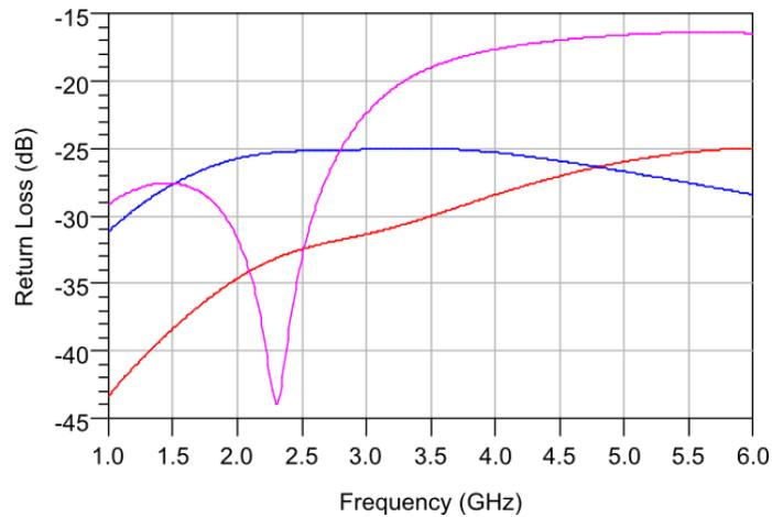
Figure 5-41. Return loss graphs of 5.625° and 11.25° phase shifter constructed with ideal elements; reference state (blue line), 5.625° phase shift state (red line), and 11.25° phase shift state (pink line).
