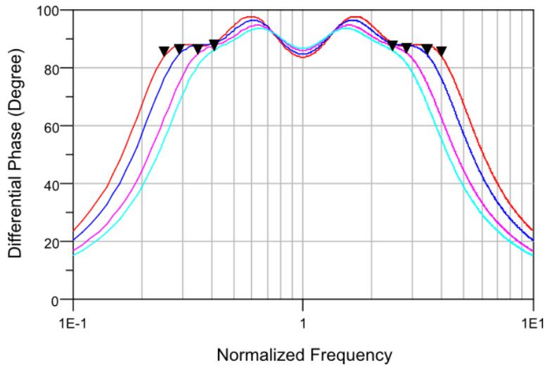
Figure 3-17. Differential phase shift plots for 90° bit four-stage for bandwidths of 6:1 (turquoise line), 8:1 (pink line), 12:1 (blue line), and 16:1 (red line).
