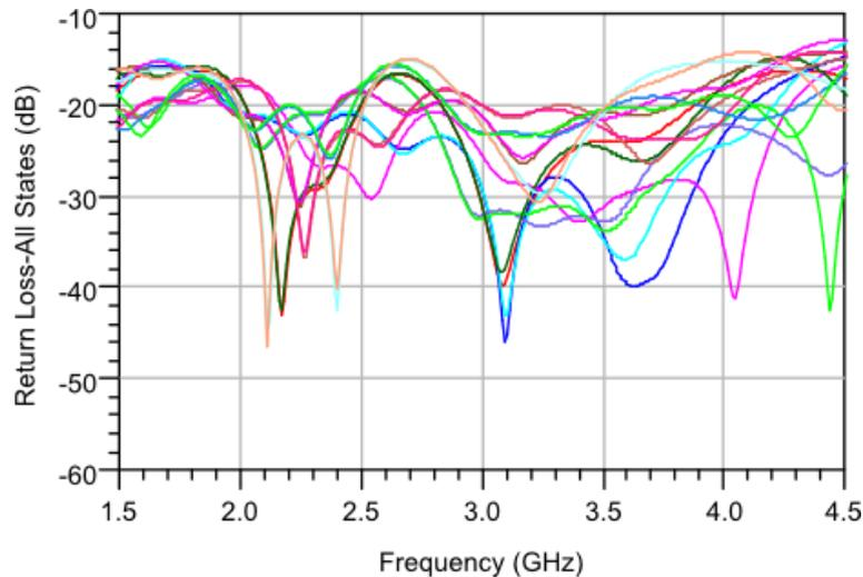
Figure 5-31. The overall performance of 2 to 4 GHz for all 16 phase shift states and the reference state  $S_{11}$  plots (Return losses).
