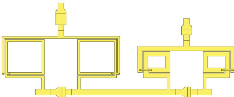
Figure A-11. Upper branch of 2 to 4 GHz phase shifter 45° phase shift bit (Length: 4.014 mm, Width: 1.652 mm, Separation between inductors: 308 μm).
