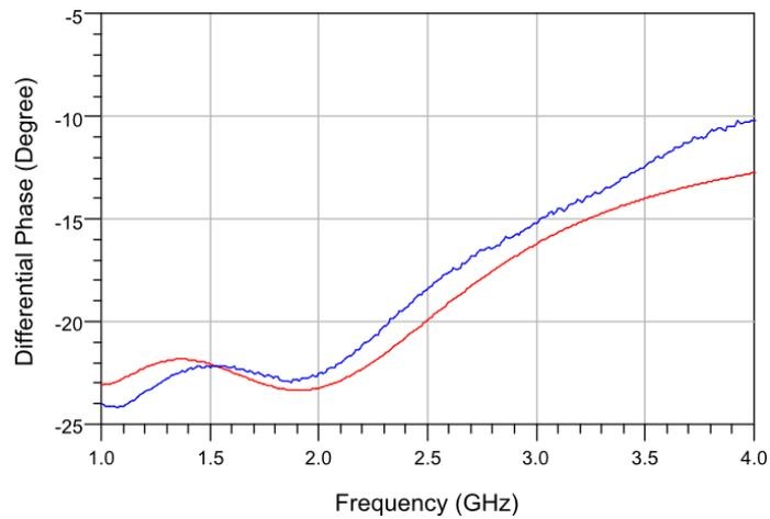
Figure 6-12. Differential phase response of 1-2 GHz 22.5° DCF phase shift bit measurement in comparison with practical design (red line represents the practical design and blue line represents the measurement result).
