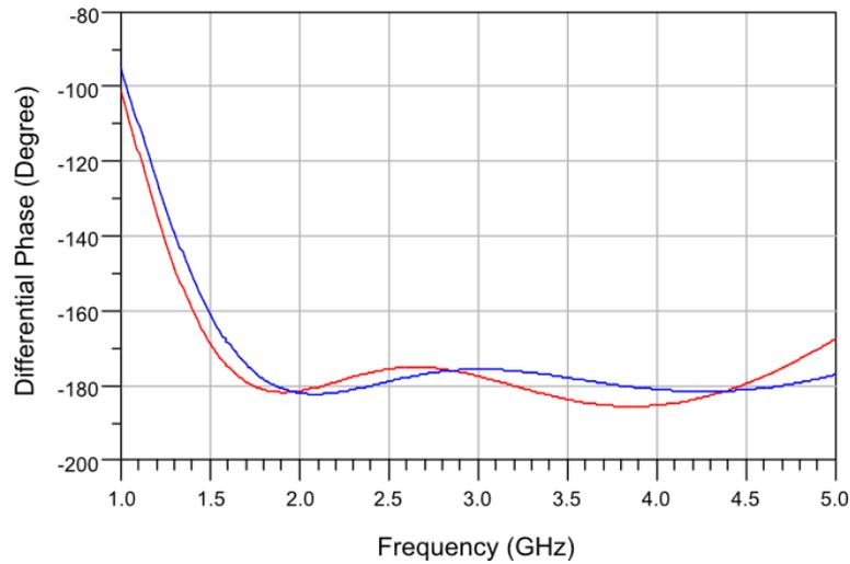
Figure A-2. The differential phase shift response of 2 to 4 GHz phase shifter 180° phase shift bit layout considered, and iterated shunt MIM capacitors (red line represents the present case, and blue line represents the ideal case).
