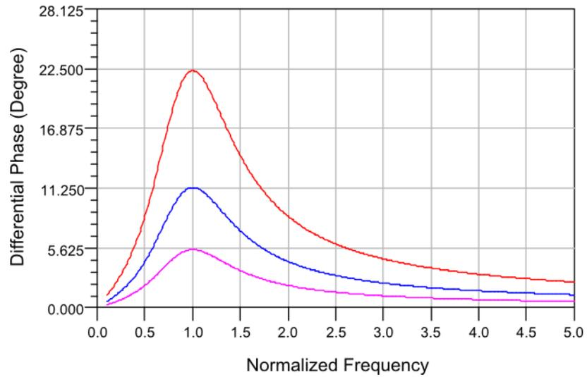
Figure 3-5. Differential phase shift plots for 5.625° (pink line), 11.25° (blue line), and 22.5° (red line).
