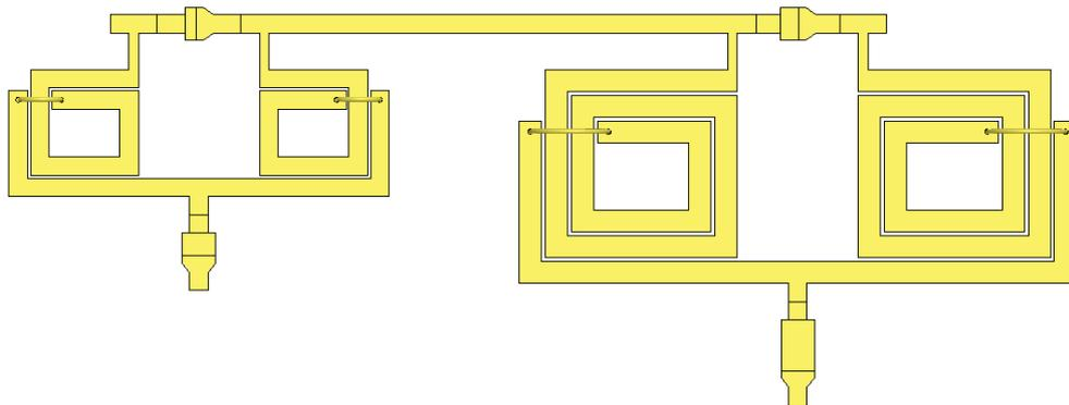
Figure 5-14. Lower branch of 1 to 2 GHz phase shifter 180° phase shift bit (Length: 5.722 mm, Width: 2.18 mm, Separation between inductors: 696  $\mu\text{m}$ ).
