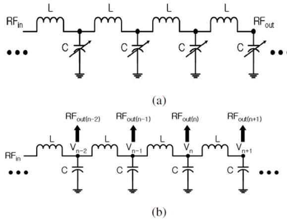
Figure 2-17. (a) The distributed analog phase shifter (b) The digital distributed phase shifter [12].
