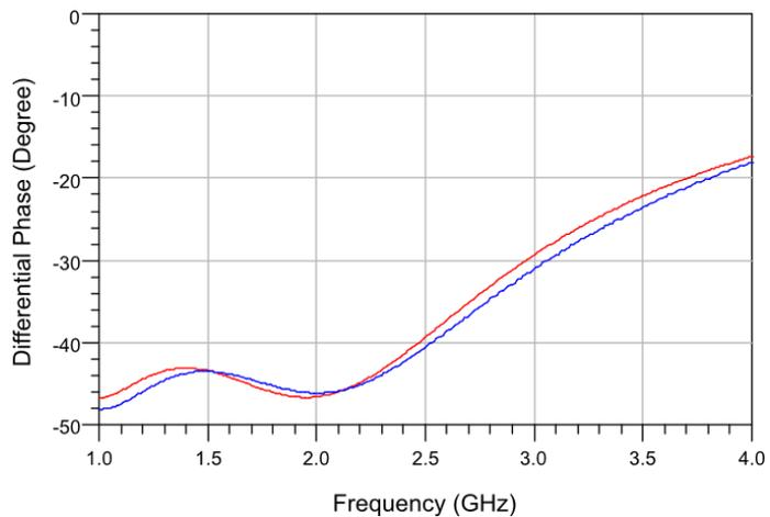
Figure 6-10. Differential phase response of 1-2 GHz 45° DCF phase shift bit measurement in comparison with practical design (red line represents the practical design and blue line represents the measurement result).
