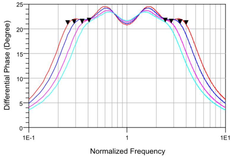
Figure 3-15. Differential phase shift plots for 22.5° bit four-stage for bandwidths of 6:1 (turquoise line), 8:1 (pink line), 12:1 (blue line), and 16:1 (red line).
