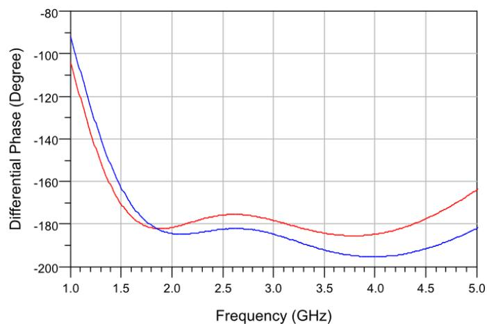
Figure 6-13. Differential phase response of 2-4 GHz 180° DCF phase shift bit measurement in comparison with practical design (red line represents the practical design and blue line represents the measurement result).
