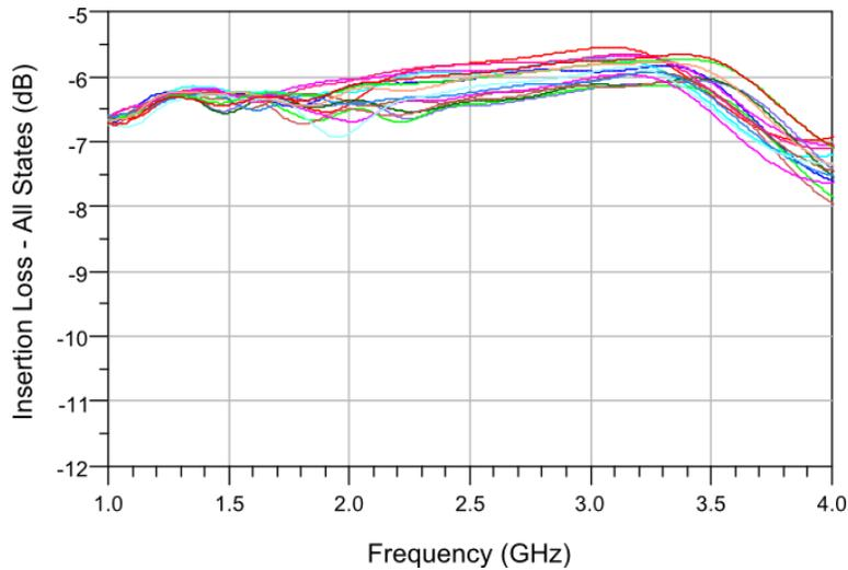
Figure 5-28. The overall performance of 1 to 2 GHz for all 16 phase shift states and the reference state  $S_{21}$  plots (Insertion losses).
