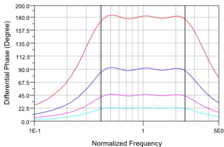
Figure 3-24. Differential phase shift plots for 22.5° (turquoise line), 45° (pink line), 90° (blue line), and 180° (red line) with achieving optimum center frequencies of all-pass filters, for three-stage 6:1 bandwidth.
