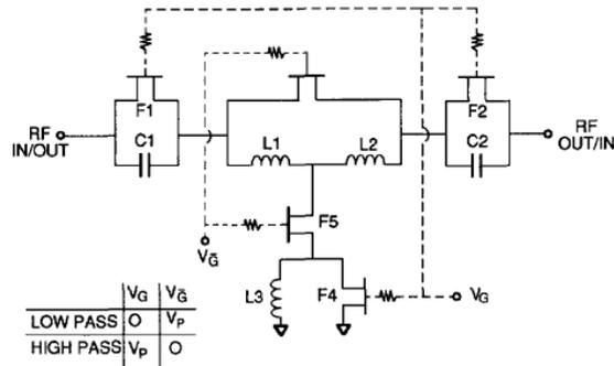
Figure 2-15. Schematic diagram of 45° and 90° bits [11].
