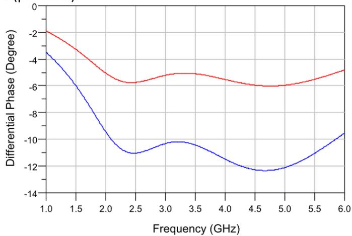
Figure 5-46. Differential phase graphs of 5.625° phase shift state (red line), and 11.25° phase shift state (blue line) of the practically constructed phase shifter.
