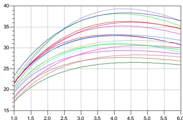
Figure 4-14. Q-factor calculations on 1.75 turn 1.44 nH planar spiral inductors for all of the trace width and spacing values.
