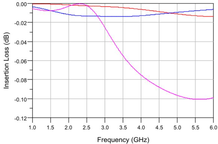
Figure 5-42. Insertion loss graphs of 5.625° and 11.25° phase shifter constructed with ideal elements; reference state (blue line), 5.625° phase shift state (red line), and 11.25° phase shift state (pink line).
