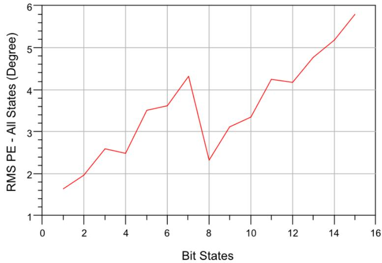
Figure 5-30. Phase rms error graph for bit states of 1 to 2 GHz 4-bit phase shifter.
