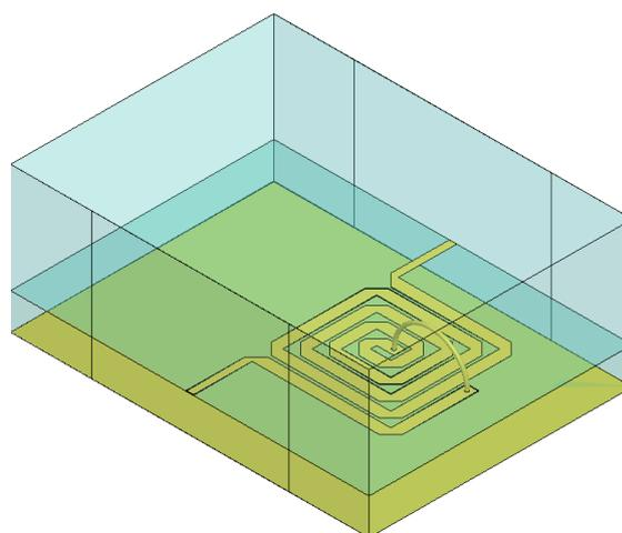
Figure 4-22. An illustration of a 4.75 turn mitered square planar spiral inductor on alumina substrate.
