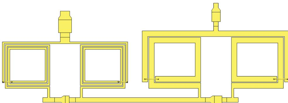
Figure 5-13. Upper branch of 1 to 2 GHz phase shifter 180° phase shift bit (Length: 6.116 mm, Width: 2.19 mm, Separation between inductors: 302 μm).
