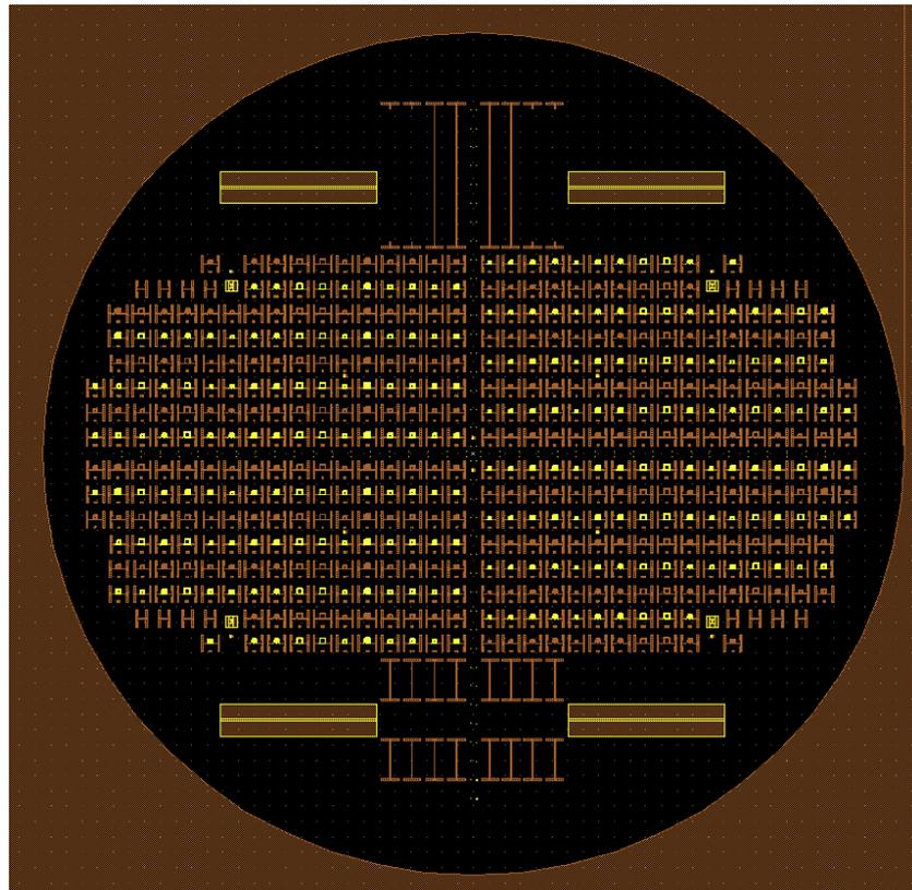
Figure 4-15. The mask layout of square planar spiral inductors.
