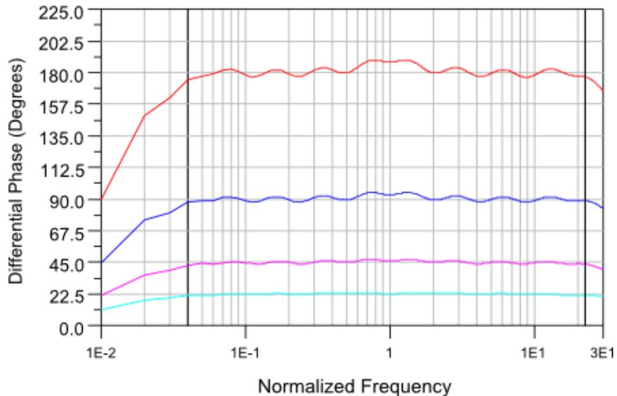
Figure 3-21. Ideal differential phase characteristics of sixteen-stage all-pass network phase shifter (Frequency is scaled to center frequency-normalized frequency in logarithmic scale) for a bandwidth of 500:1 (between the black vertical lines).
