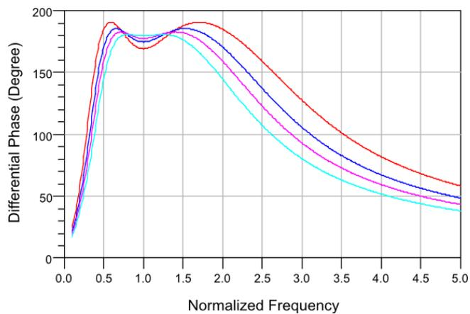
Figure 3-13. Differential phase shift plots for 180° bit two-stage for bandwidths of 2:1 (turquoise line), 3:1 (pink line), 4:1 (blue line), and 6:1 (red line).
