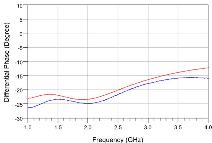
Figure 6-11. Differential phase response of 1-2 GHz 22.5° M phase shift bit measurement in comparison with practical design (red line represents the practical design and blue line represents the measurement result).
