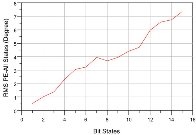
Figure 5-34. Phase rms error graph for bit states of 2 to 4 GHz 4-bit phase shifter.
