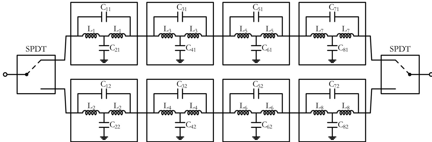
Figure 3-14. The four-stage all-pass network phase shifter with component names. Only one bit is illustrated.
