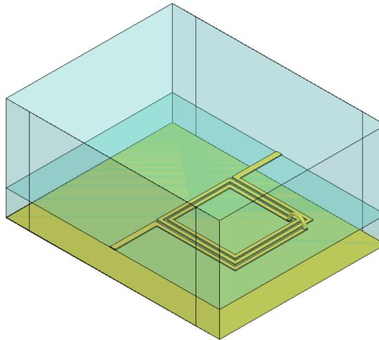
Figure 4-13. 2.75 turn square planar spiral inductor drawn parametrically in 3D EM simulator HFSS [76] (the substrate is chosen as alumina, and the metal is chosen as gold with a thickness  $7\ \mu\text{m}$ ).
