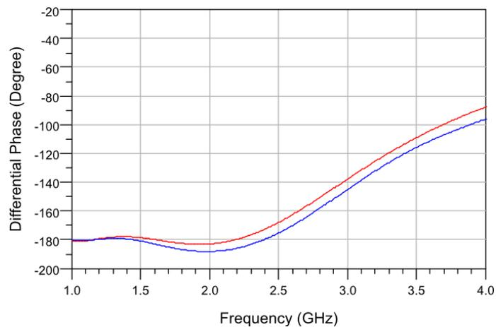
Figure 6-4. Differential phase response of 1-2 GHz 180° DCM phase shift bit measurement in comparison with practical design (red line represents the practical design and blue line represents the measurement result).
