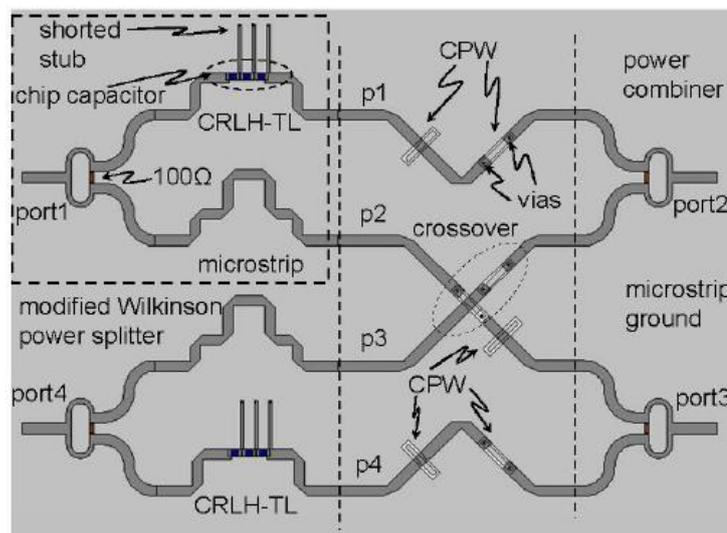
Figure 2-24. Complete structure of the proposed broadband four-port quadrature hybrid. [17]
