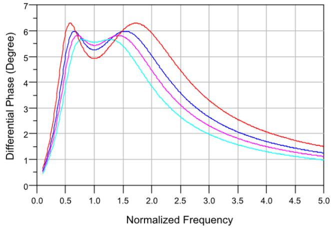
Figure 3-8. Differential phase shift plots for 5.625° bit two-stage for bandwidths of 2:1 (turquoise line), 3:1 (pink line), 4:1 (blue line), and 6:1 (red line).
