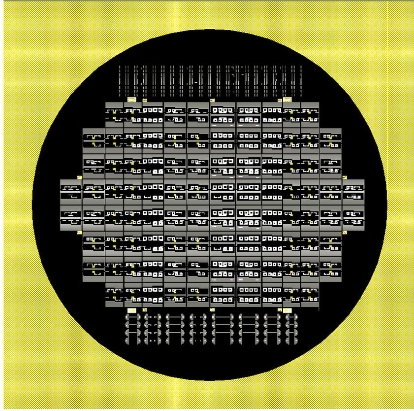
Figure 6-2. Mask Set of Phase Shifters.
