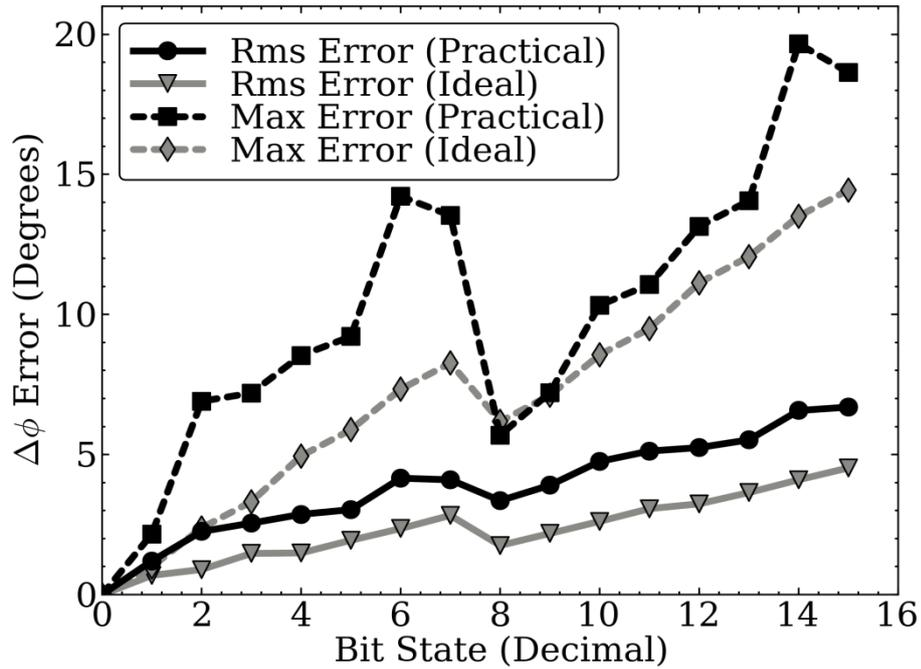
Figure 5-49. rms phase error, and maximum phase error analysis of all bit states for 1 to 6 GHz phase shifter.
