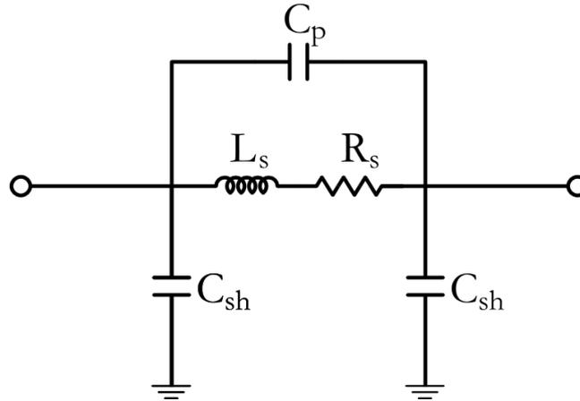
Figure 4-10. Lumped equivalent circuit for planar spiral inductors on alumina or quartz.
