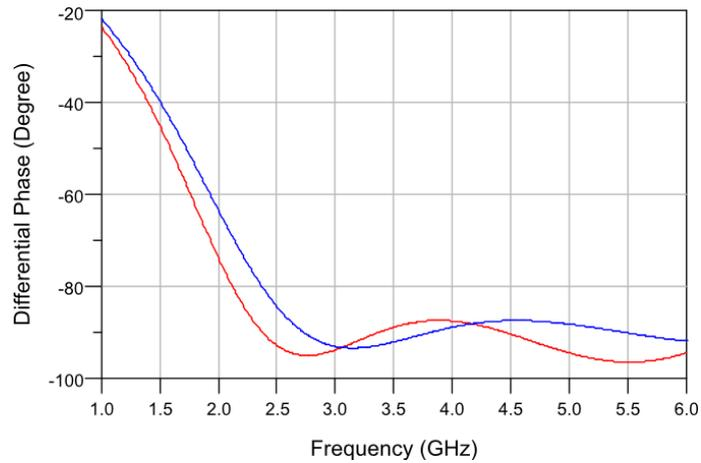
Figure B-6. The differential phase shift response of 3 to 6 GHz phase shifter 90° phase shift bit layout considered, and iterated shunt MIM capacitors (red line represents the present case, and blue line represents the ideal case).
