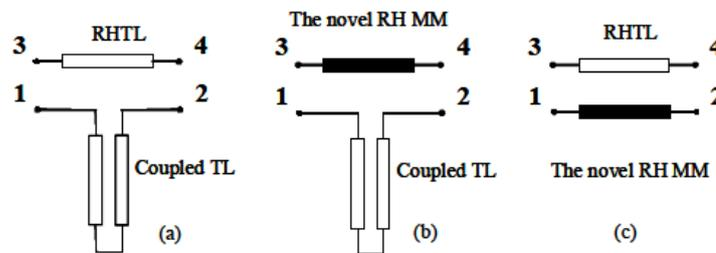
Figure 2-26. Three circuit schemes for (a) Standard Schiffman phase shifter, (b) Type-A: new differential phase shifter based on the coupled TL and RH MM TL, (c) Type-B: new differential phase shifter using the RH MM TL and conventional RHTL [19].
