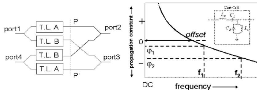
Figure 2-23. (a) Architecture of the broadband quadrature hybrid. (b) Dispersion diagram of the metamaterial transmission line, CRLH-TL. [17]
