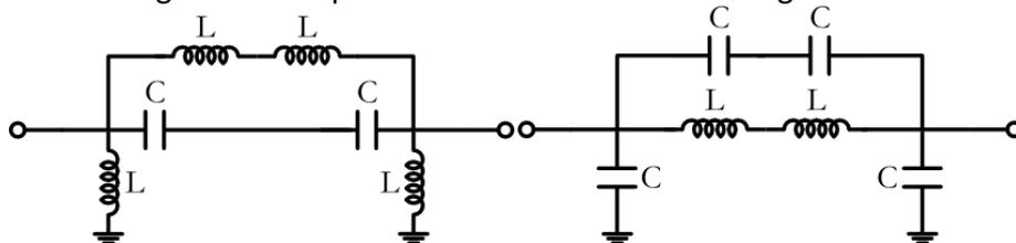
Figure 3-3. Series L and series C circuits respectively to analyze even and odd modes
