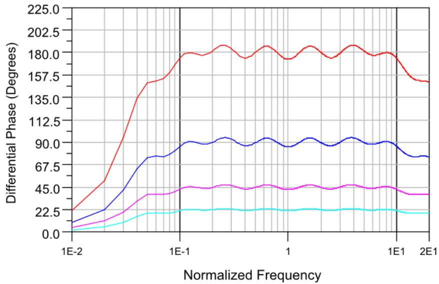
Figure 3-20. Ideal differential phase characteristics of eight-stage all-pass network phase shifter (Frequency is scaled to center frequency-normalized frequency in logarithmic scale) for a bandwidth of 100:1 (between the black vertical lines).
