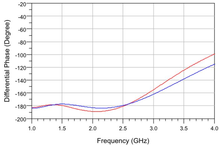
Figure 5-2. The differential phase shift response of 1 to 2 GHz phase shifter 180° phase shift bit configuration # 1 (red line represents the present case, and blue line represents the ideal case).
