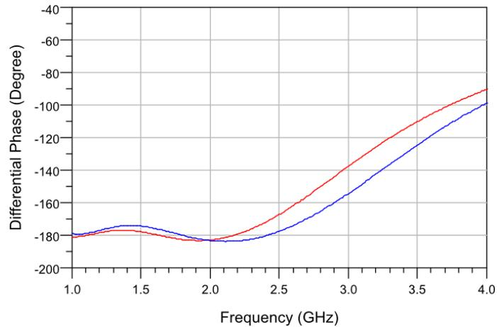
Figure 6-5. Differential phase response of 1-2 GHz 180° DCF phase shift bit measurement in comparison with practical design (red line represents the practical design and blue line represents the measurement result).
