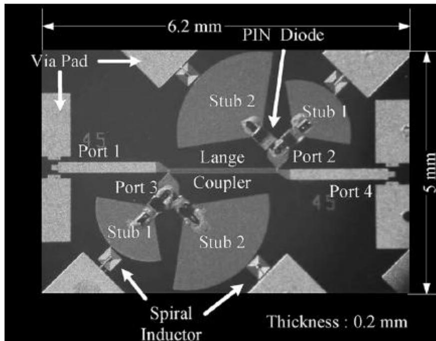
Figure 2-3. Photograph of fabricated 6–18 GHz  $45^\circ$  phase shifter [5].
