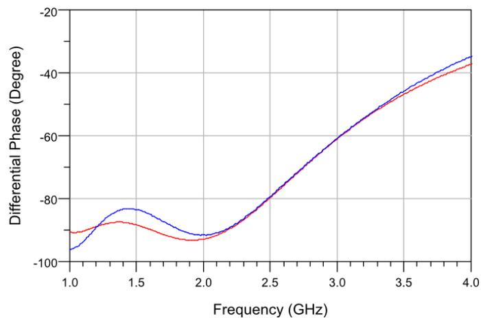
Figure 6-6. Differential phase response of 1-2 GHz 90° M phase shift bit measurement in comparison with practical design (red line represents the practical design and blue line represents the measurement result).
