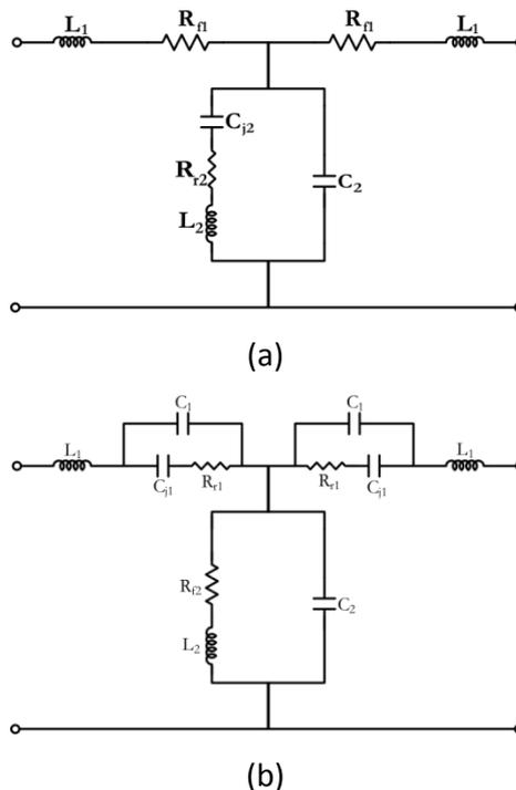
Figure 2-9. Bias States of the Proposed Phase Shifter (a) diodes-1 are forward biased and diode-2 is reverse biased (b) diodes-1 are reverse biased and diode-2 is forward biased.
