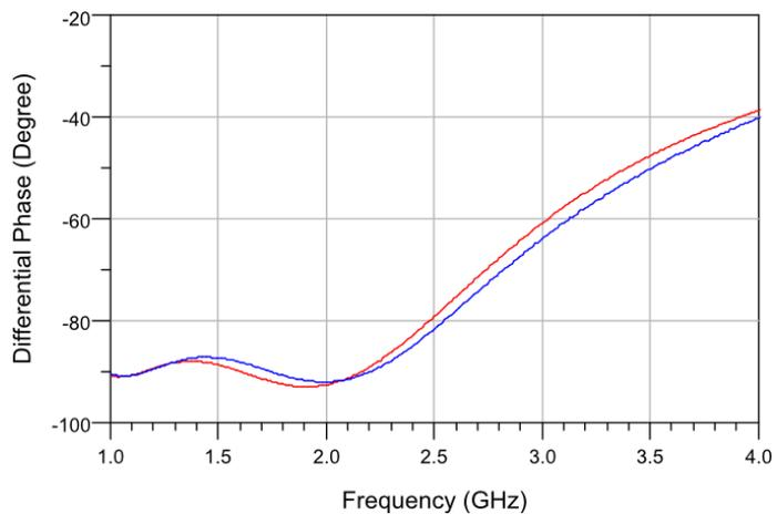
Figure 6-8. Differential phase response of 1-2 GHz 90° DCF phase shift bit measurement in comparison with practical design (red line represents the practical design and blue line represents the measurement result).
