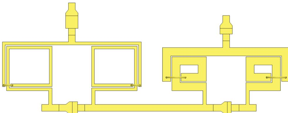
Figure B-3. Upper branch of 3 to 6 GHz phase shifter 180° phase shift bit (Length: 4.134 mm, Width: 1.628 mm, Separation between inductors: 304 μm).
