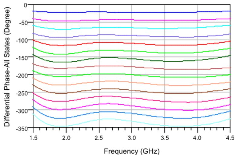
Figure 5-33. The overall differential phase shift performance of 2 to 4 GHz phase shifter for all 15 phase shift states with respect to reference phase shift state.
