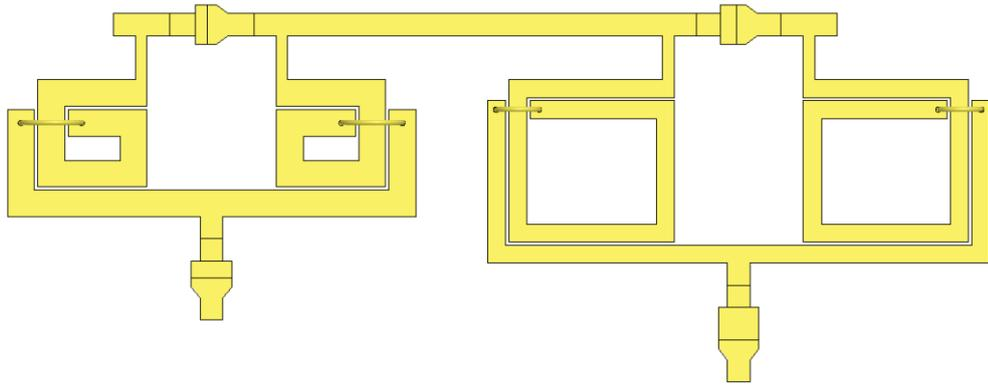
Figure A-8. Lower branch of 2 to 4 GHz phase shifter 90° phase shift bit (Length: 4.374 mm, Width: 1.709 mm, Separation between inductors: 318 μm).
