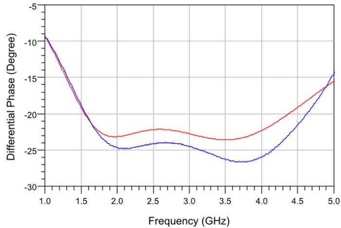
Figure 6-17. Differential phase response of 2-4 GHz 22.5° M phase shift bit measurement in comparison with practical design (red line represents the practical design and blue line represents the measurement result).
