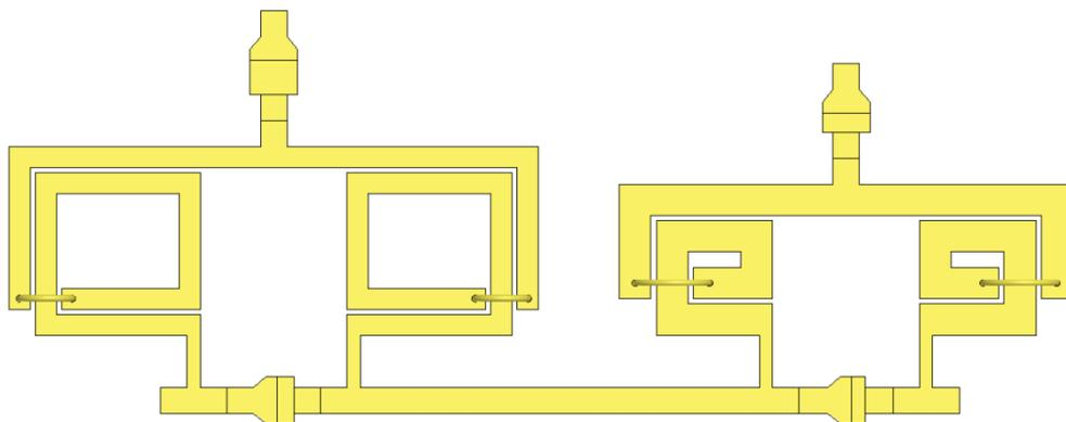
Figure B-15. Upper branch of 3 to 6 GHz phase shifter 22.5° phase shift bit (Length: 4.026 mm, Width: 1.546 mm, Separation between inductors: 306 μm).
