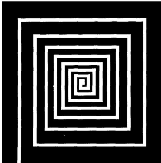
Figure 4-1. Optimized layout of a 20 nH inductor [49].
