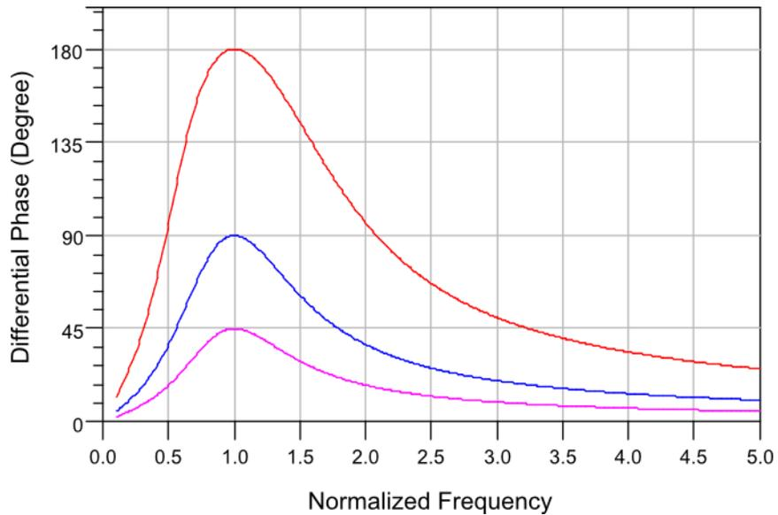
Figure 3-6. Differential phase shift plots for 45° (pink line), 90° (blue line), and 180° (red line).
