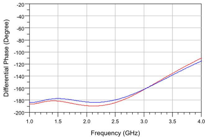
Figure 5-4. The differential phase shift response of 1 to 2 GHz phase shifter 180° phase shift bit configuration # 1 with iterated shunt MIM capacitors (red line represents the present case, and blue line represents the ideal case).
