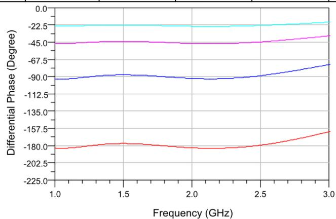
Figure 3-25. Ideal differential phase characteristics of two-stage, four-bit, 1 to 2 GHz phase shifter.
