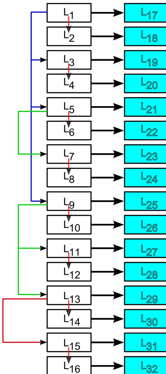
Figure 3-19. The sequence and ability to derive the inductor formulae diagram for sixteen-stage, all-pass network phase shifter.
