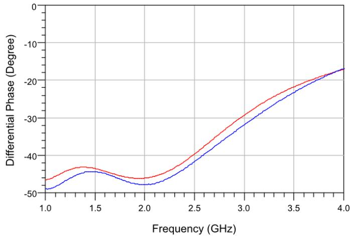
Figure 6-9. Differential phase response of 1-2 GHz 45° M phase shift bit measurement in comparison with practical design (red line represents the practical design and blue line represents the measurement result).
