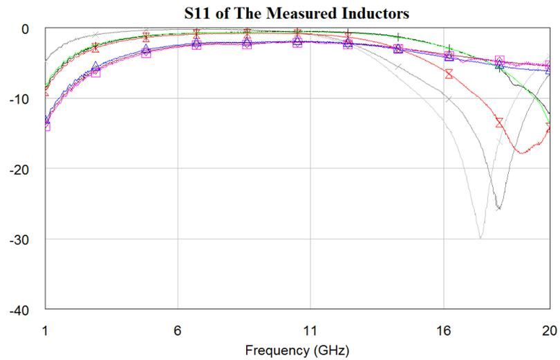
Figure 4-18. dB(S11) responses of the measured inductors with SOLT calibration and without de-embedding.
