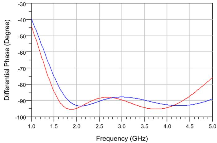
Figure A-6. The differential phase shift response of 2 to 4 GHz phase shifter 90° phase shift bit layout considered, and iterated shunt MIM capacitors (red line represents the present case, and blue line represents the ideal case).
