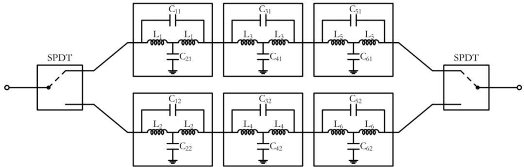
Figure 3-22. The three-stage all-pass network phase shifter with component names. Only one bit is illustrated.
