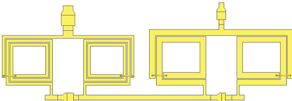
Figure 5-17. Upper branch of 1 to 2 GHz phase shifter 90° phase shift bit (Length: 5.856 mm, Width: 2.026 mm, Separation between inductors: 308 μm).
