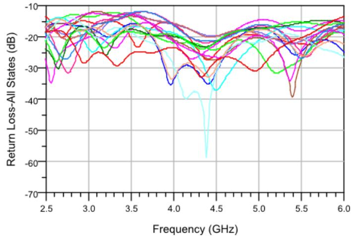
Figure 5-35. The overall performance of 3 to 6 GHz for all 16 phase shift states and the reference state  $S_{11}$  plots (Return losses).
