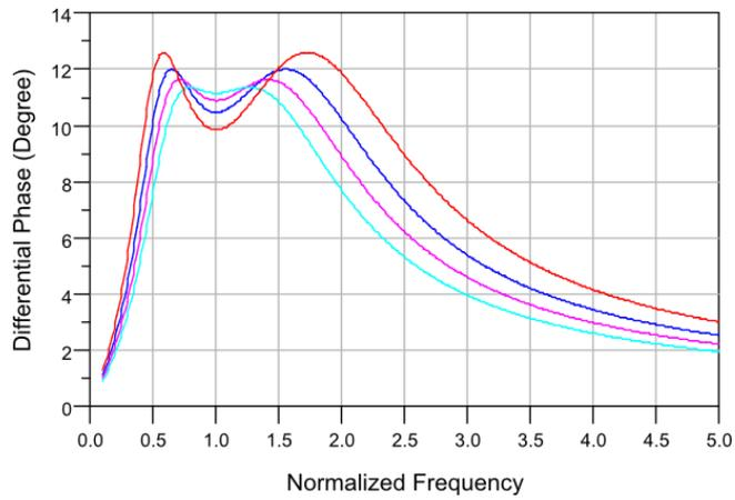
Figure 3-9. Differential phase shift plots for 11.25° bit two-stage for bandwidths of 2:1 (turquoise line), 3:1 (pink line), 4:1 (blue line), and 6:1 (red line).
