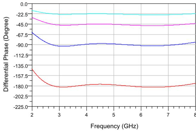
Figure 3-27. Ideal differential phase characteristics of two-stage, four-bit, 3 to 6 GHz phase shifter.
