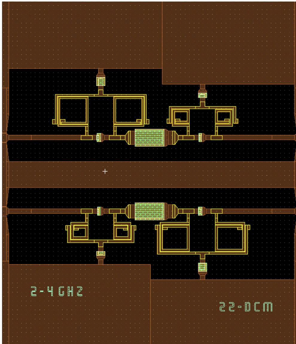
Figure 6-1. An example phase shift bit layout with DC blocking capacitor between the two all-pass filters for each upper and lower branches.
