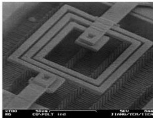
Figure 4-2. SEM image of a suspended inductor [50].
