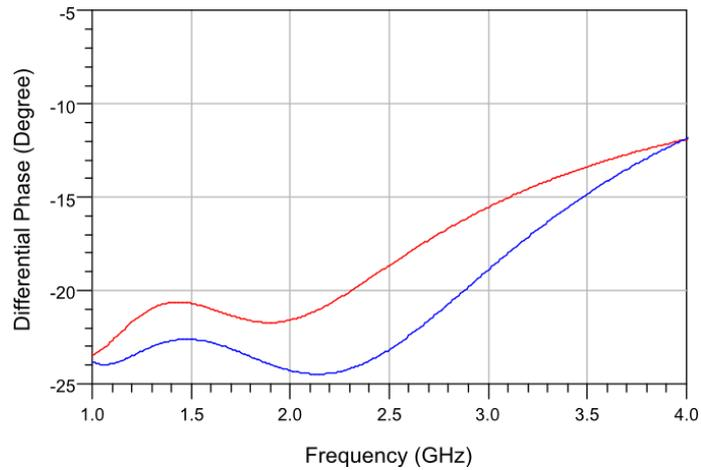
Figure 5-24. The differential phase shift response of 1 to 2 GHz phase shifter 22.5° phase shift bit configuration # layout considered, and iterated shunt MIM capacitors (red line represents the present case, and blue line represents the ideal case).
