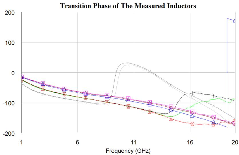
Figure 4-20. Phase angle(S21) responses of the measured inductors with SOLT calibration and without de-embedding.
