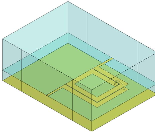
Figure 4-8. 1.75 turn square planar spiral inductor drawn parametrically in 3D EM simulator HFSS [76] (the substrate is chosen as alumina, and the metal is chosen as gold with a thickness  $1\ \mu\text{m}$ ).
