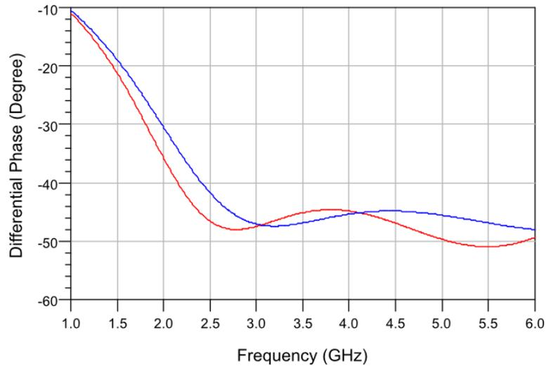
Figure B-10. The differential phase shift response of 3 to 6 GHz phase shifter 45° phase shift bit layout considered, and iterated shunt MIM capacitors (red line represents the present case, and blue line represents the ideal case).
