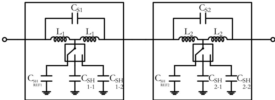
Figure 5-39. Novel 2 bit SPDT-less all-pass network phase shifter.
