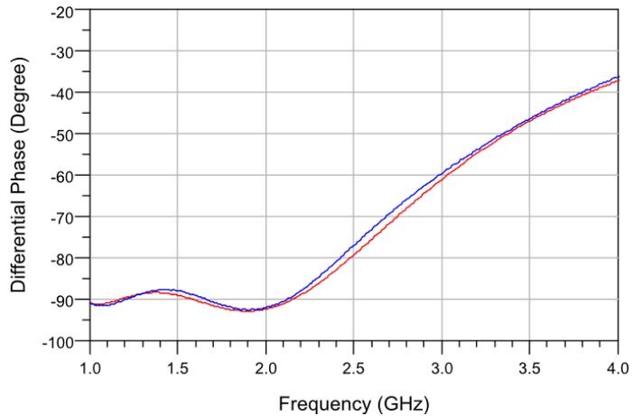
Figure 6-7. Differential phase response of 1-2 GHz 90° DCM phase shift bit measurement in comparison with practical design (red line represents the practical design and blue line represents the measurement result).
