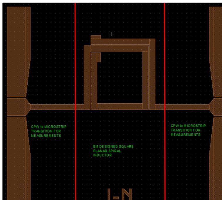
Figure 4-16. An example of the designed square planar spiral inductor, in which fixtures for measurements could be observed.
