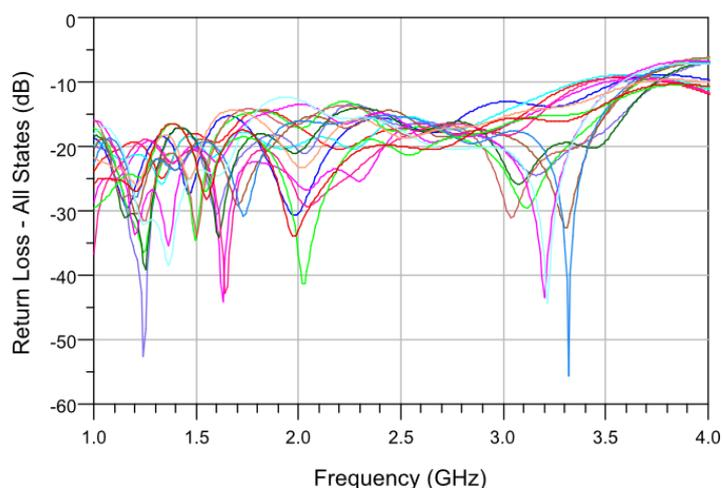
Figure 5-27. The overall performance of 1 to 2 GHz for all 16 phase shift states and the reference state  $S_{11}$  plots (Return losses).
