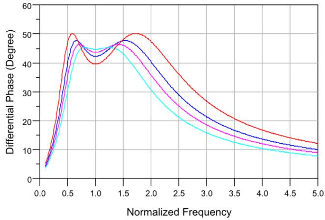
Figure 3-11. Differential phase shift plots for 45° bit two-stage for bandwidths of 2:1 (turquoise line), 3:1 (pink line), 4:1 (blue line), and 6:1 (red line).
