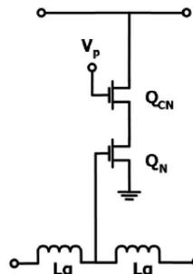
Figure 2-18. The schematic of a single T-section [12].
