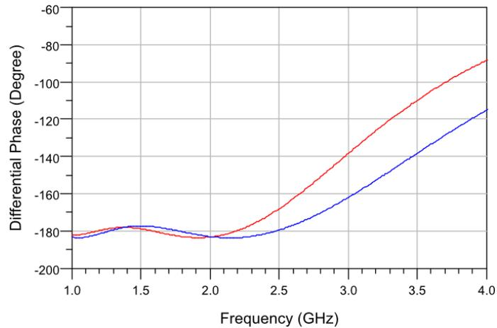
Figure 5-12. The differential phase shift response of 1 to 2 GHz phase shifter 180° phase shift bit layout considered, and iterated shunt MIM capacitors (red line represents the present case, and blue line represents the ideal case).
