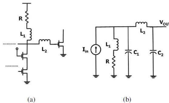
Figure 2-19. (a) Shunt and series peaking load (b) Simplified model [12].
