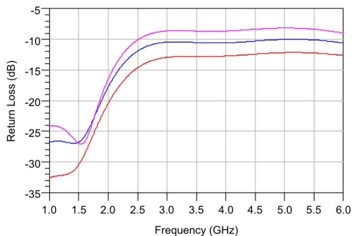
Figure 5-44. Return loss graphs of 5.625° and 11.25° practically constructed phase shifter; reference state (blue line), 5.625° phase shift state (red line), and 11.25° phase shift state (pink line).
