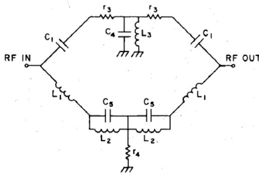
Figure 2-13. The circuit representation when state becomes  $V_2$  is equal to zero and  $V_1$  is below the pinch-off [9].
