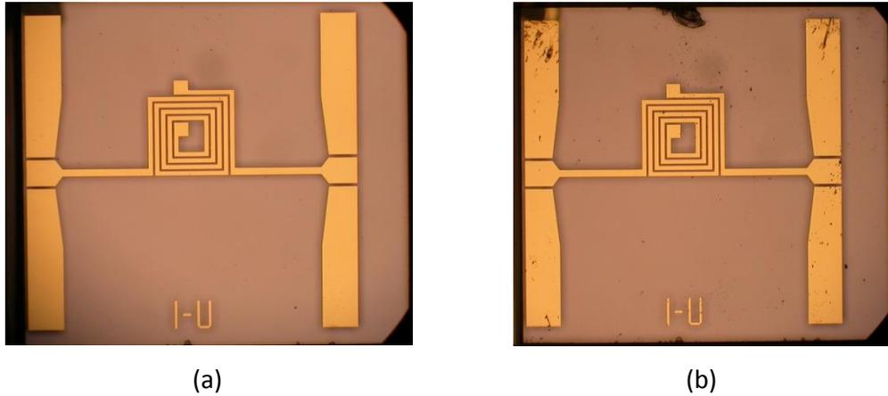
Figure 4-17. An example of an ultrasonically-bonded inductor, 1U (a) Before bonding (b) After bonding.
