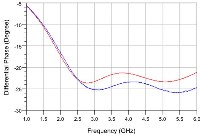
Figure 6-19. Differential phase response of 3-6 GHz 22.5° DCF phase shift bit measurement in comparison with practical design (red line represents the practical design and blue line represents the measurement result).
