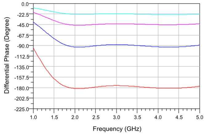
Figure 3-26. Ideal differential phase characteristics of two-stage, four-bit, 2 to 4 GHz phase shifter.
