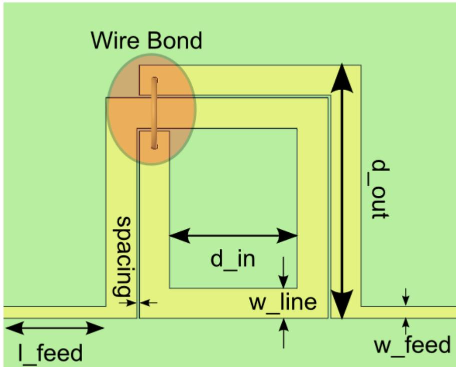
Figure 4-7. Illustration of square planar spiral inductor with geometrical parameters, and wire bond.
