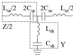
Figure 2-25. Equivalent circuit mode for the ideal TL unit cell of RH MMs [19]
