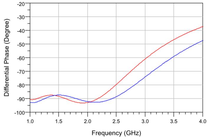
Figure 5-16. The differential phase shift response of 1 to 2 GHz phase shifter 90° phase shift bit layout considered, and iterated shunt MIM capacitors (red line represents the present case, and blue line represents the ideal case).
