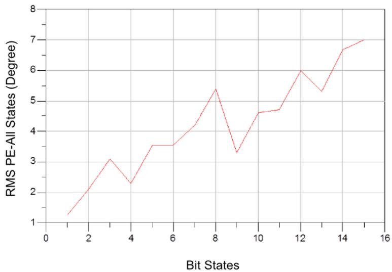
Figure 5-38. Phase rms error graph for bit states of 3 to 6 GHz 4-bit phase shifter.
