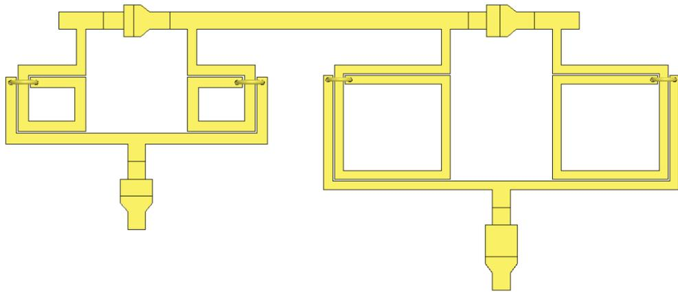
Figure A-16. Lower branch of 2 to 4 GHz phase shifter 22.5° phase shift bit (Length: 3.766 mm, Width: 1.617 mm, Separation between inductors: 314  $\mu\text{m}$ ).
