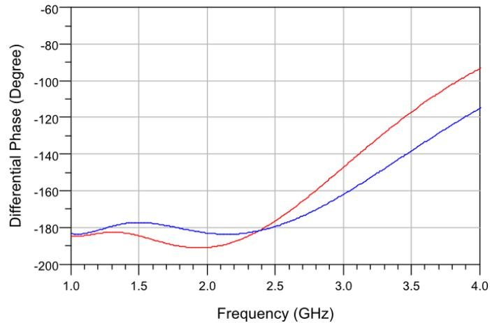
Figure 5-10. The differential phase shift response of 1 to 2 GHz phase shifter 180° phase shift bit configuration # layout considered (red line represents the present case, and blue line represents the ideal case).
