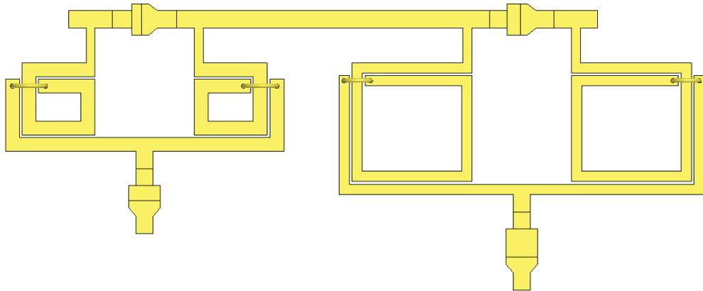
Figure A-12. Lower branch of 2 to 4 GHz phase shifter 45° phase shift bit (Length: 4.006 mm, Width: 1.656 mm, Separation between inductors: 316  $\mu\text{m}$ ).
