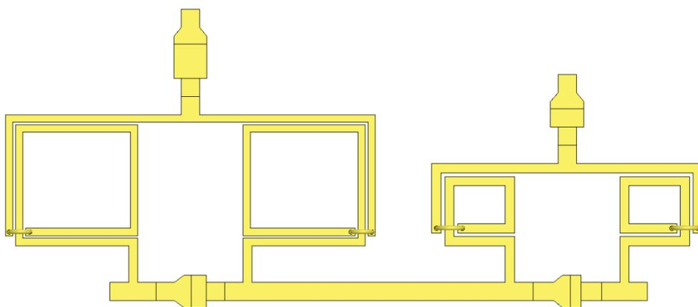
Figure A-15. Upper branch of 2 to 4 GHz phase shifter 22.5° phase shift bit (Length: 3.774 mm, Width: 1.633 mm, Separation between inductors: 306 μm).
