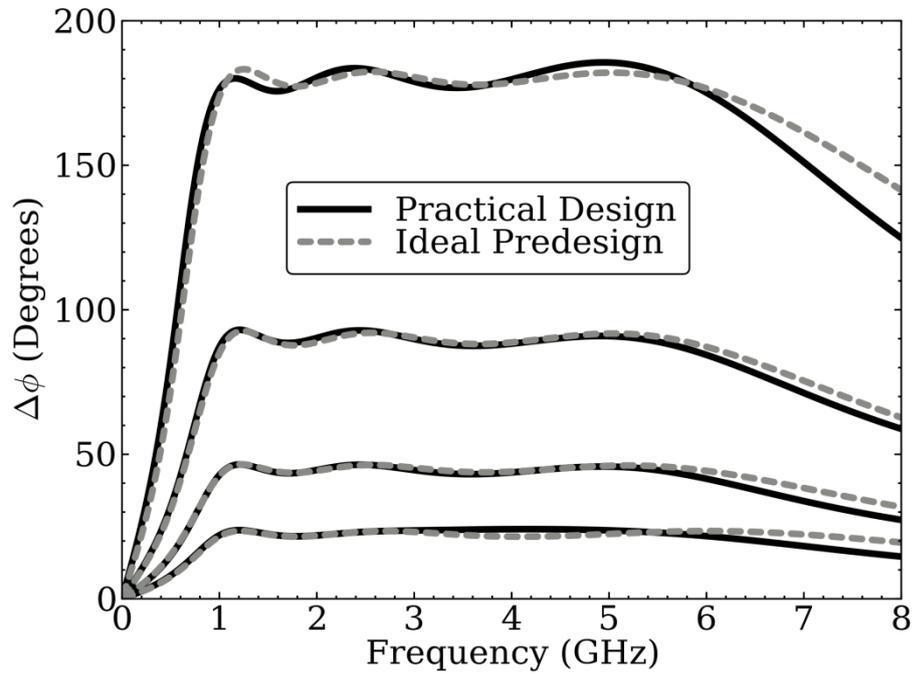
Figure 5-47. A comparison of the single-bit differential phase responses between the ideal UWB phase shifter design (using ideal elements) and the practical design (using surface micromachined lumped elements).
