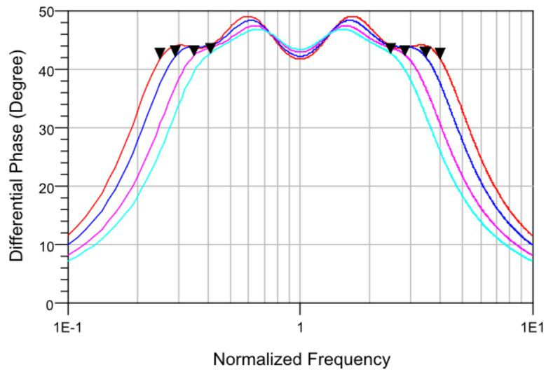
Figure 3-16. Differential phase shift plots for 45° bit four-stage for bandwidths of 6:1 (turquoise line), 8:1 (pink line), 12:1 (blue line), and 16:1 (red line).
