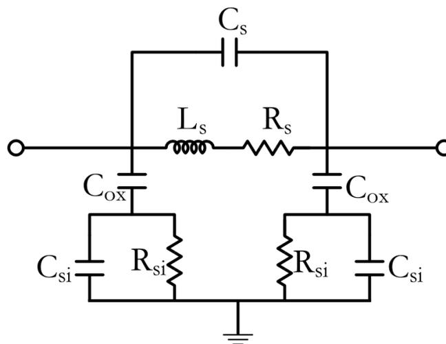
Figure 4-9. Lumped equivalent circuit for planar spiral inductors on silicon.
