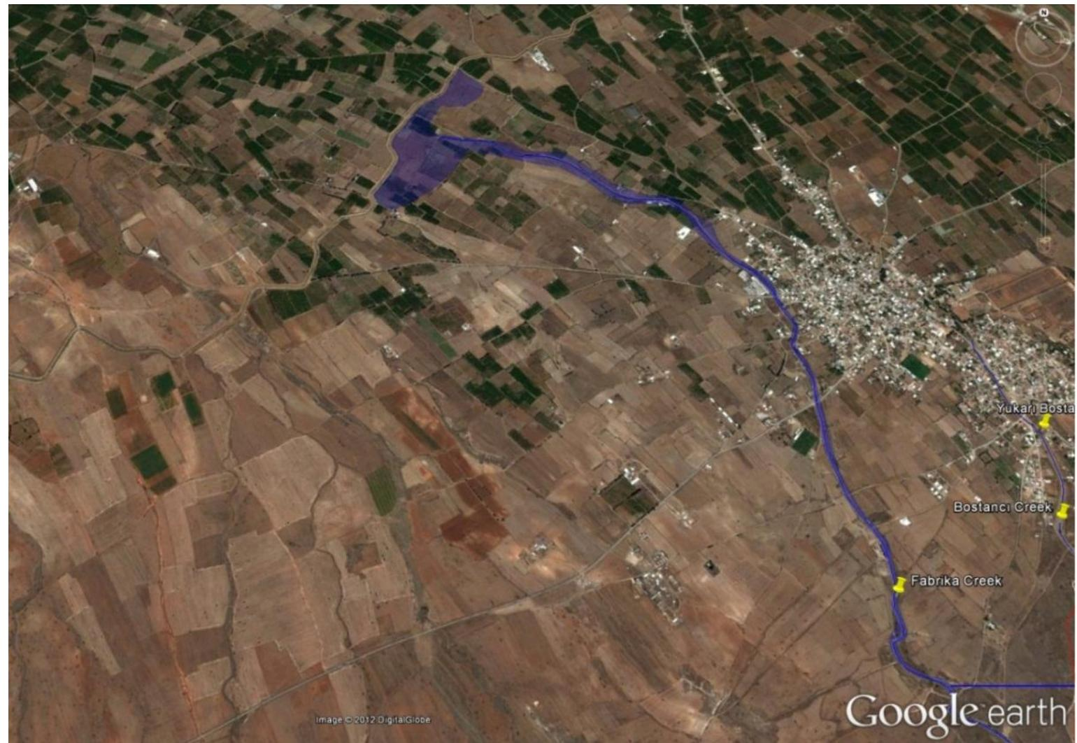
Figure 6.14 Flood inundation map of Fabrika Creek for  $Q=183.75 \text{ m}^3/\text{s}$  (Google Earth, 2011)
