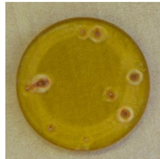
*Figure 19 ZnSe target with different sized craters on it due to different spot sizes of the focusing laser*
