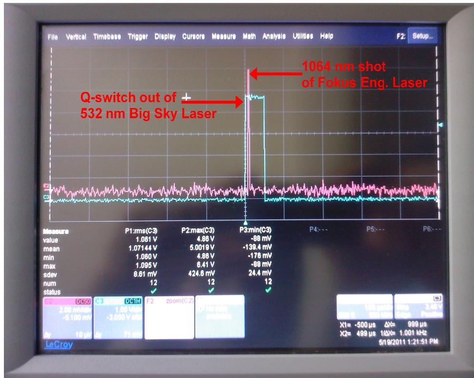
Figure 25. Pulse timings of the laser shown in oscilloscope screen
