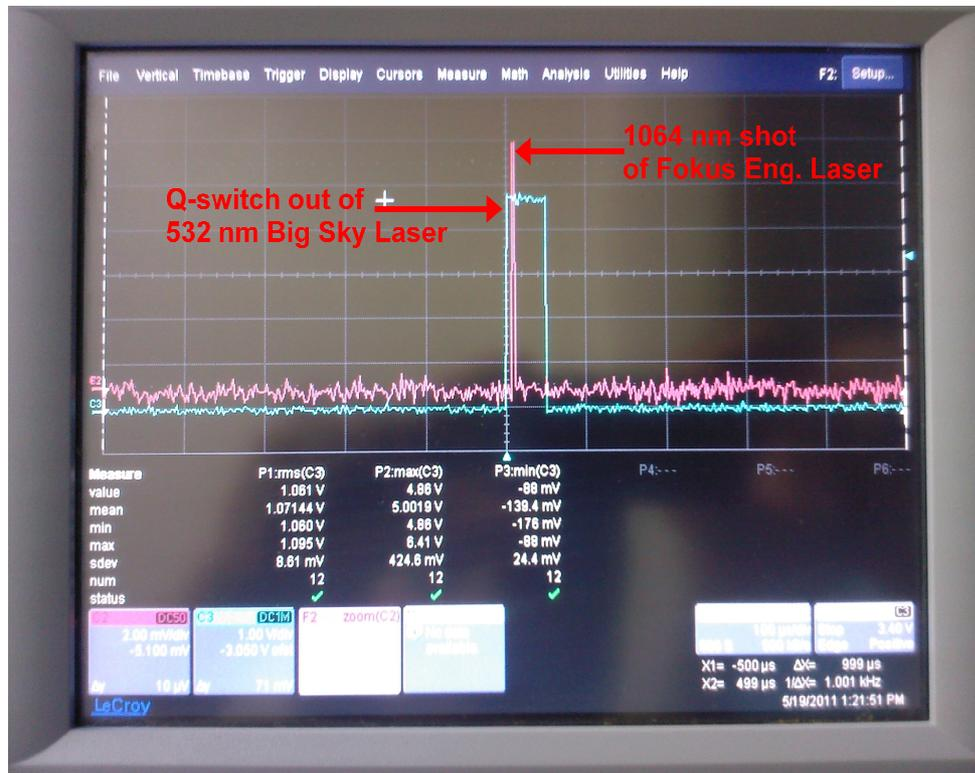
Figure 25. Pulse timings of the laser shown in oscilloscope screen
