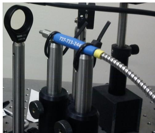
*Figure 20 A converging lens and fiber optic cable for collecting the spectral emission*
