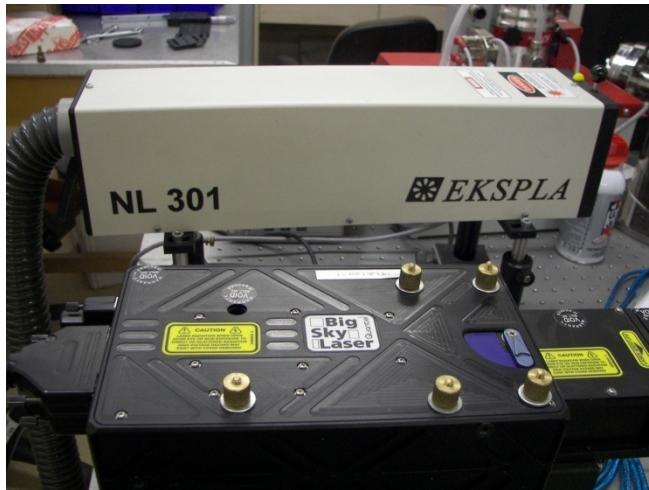
*Figure 17. Two different Nd:YAG lasers, One at 1064 nm (Ekspla NL 301) and the other is the second harmonic, i.e. at 532 nm (Big Sky)*
