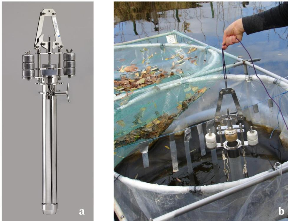
**Figure 6: a) Kajak core sampler, b) View from benthic macroinvertebrate sampling**
