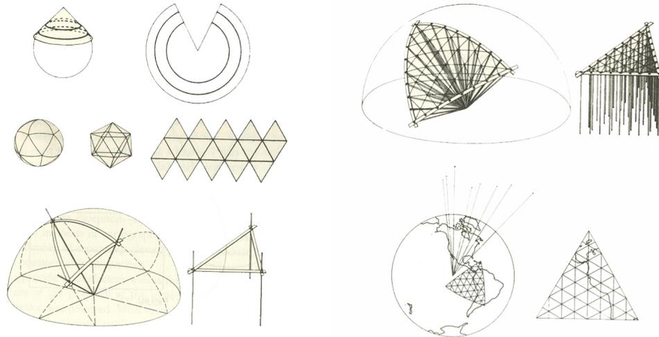
**Figure 2.9** Buckminster Fuller's sketches about the development of geodesic domes.
