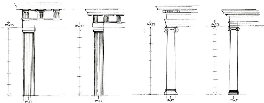
**Figure 2.1** Vitruvius’ illustrations on the proportional evolution of Doric and Ionian Columns, depending on the alteration of analogy object, from a man to a slender woman (from left to right).
