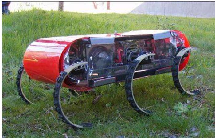
Figure 2.2: SensoRHex is a robot platform that can walk on irregular terrain which is a useful property especially for outdoors
