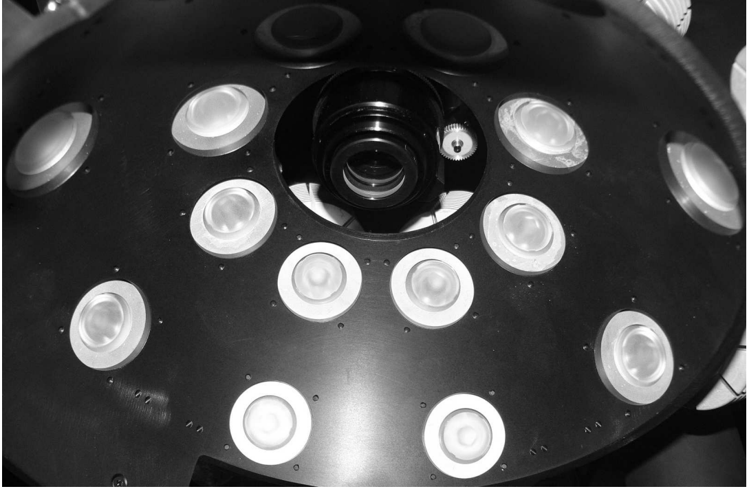
Figure 6.2: (a) Imaging camera at middle and 16 LEDs placed around it
