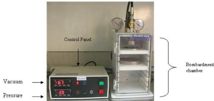
Figure 2. 12. Obitek Biolab Gene Transfer System
