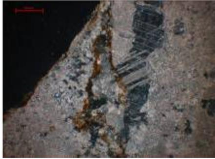
**Figure 3.17** View of a crack with karstic vein having iron oxides and calcite crystals, cross nicols, scale bar: 100  $\mu$
