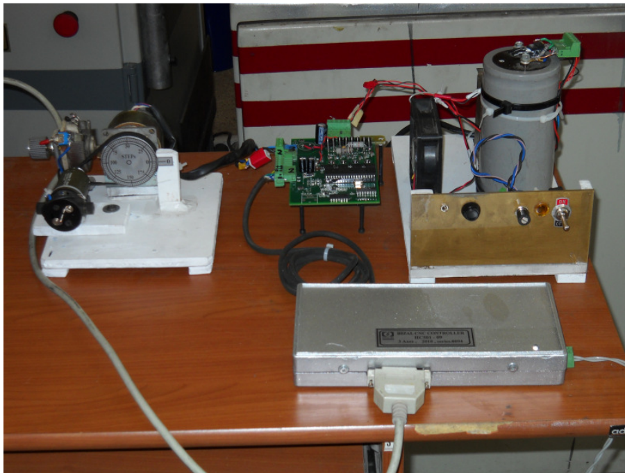
Figure 33 Experimental setup: step motor and load on the left, driver in the middle and the power supply on the right. PC controller interface is seen in the front.
