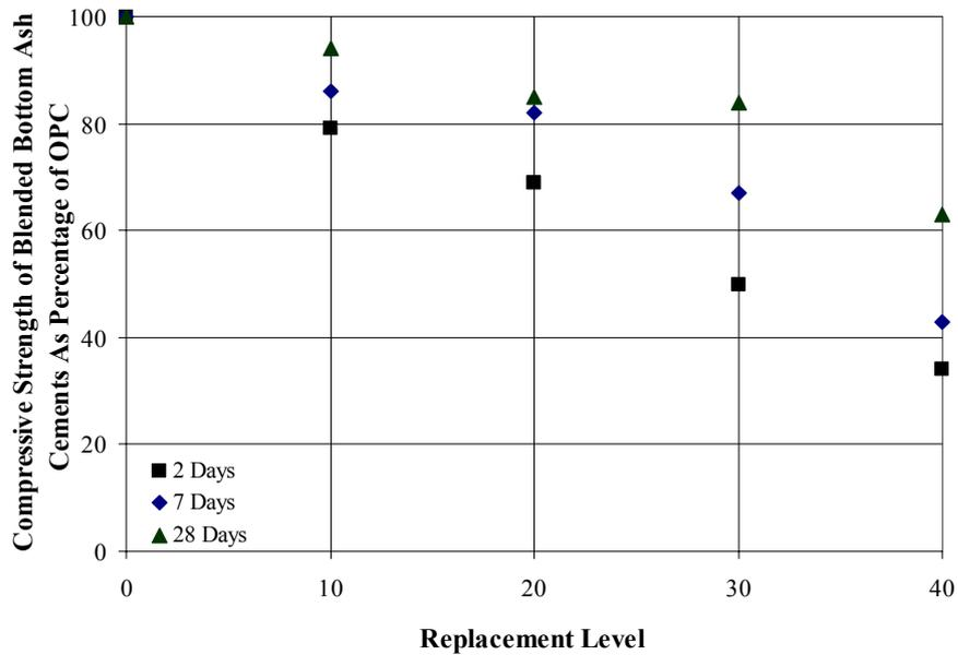
Figure 4.7 Strengths of Blended Bottom Ash Cements as Percentage of that of OPC
