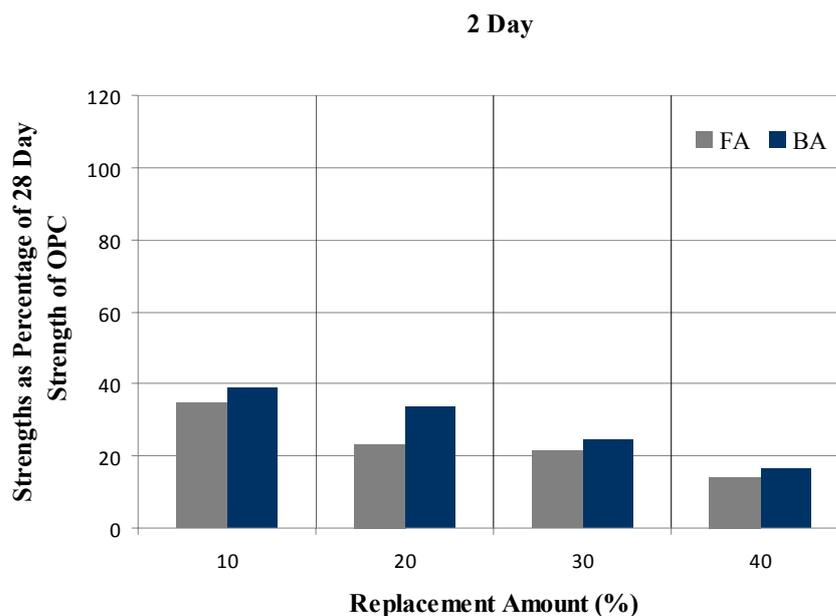
Figure 4.8 Compressive Strengths of Blended Cements at 2<sup>nd</sup> Day as Percentage of Strength of OPC at 28<sup>th</sup> Day
