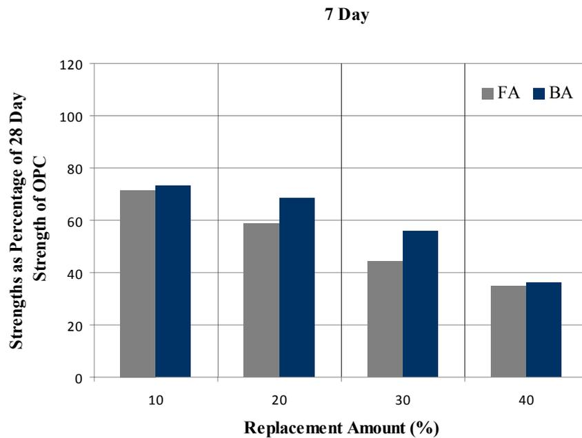
Figure 4.9 Compressive Strengths of Blended Cements at 7<sup>th</sup> Day as Percentage of Strength of OPC at 28<sup>th</sup> Day
