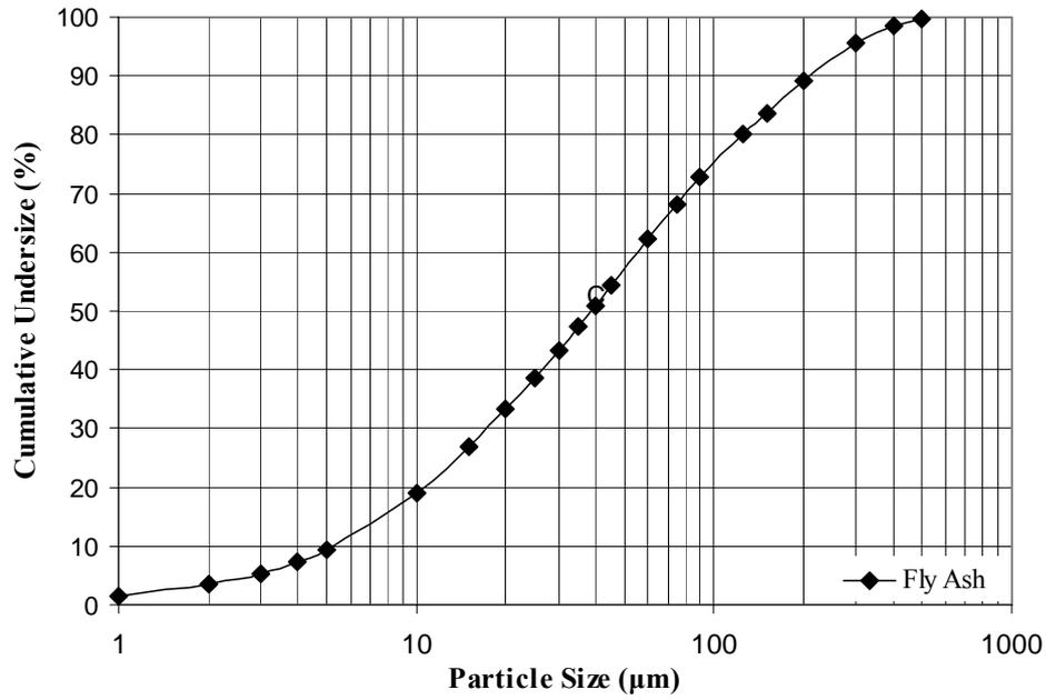
Figure 4.3 Particle Size Distribution of Fly Ash
