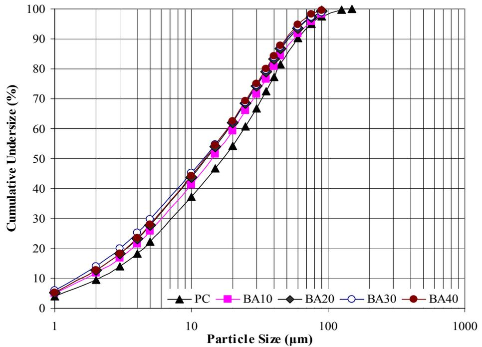
Figure 4.5 Particle Size Distributions of Blended Bottom Ash Cements
