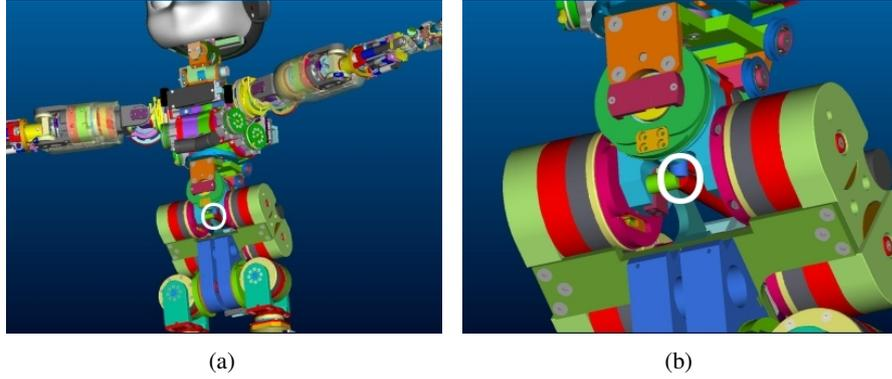
Figure B.1: Origin of the root reference frame for the iCub robot is shown with a white circle. Figure taken from [3].
