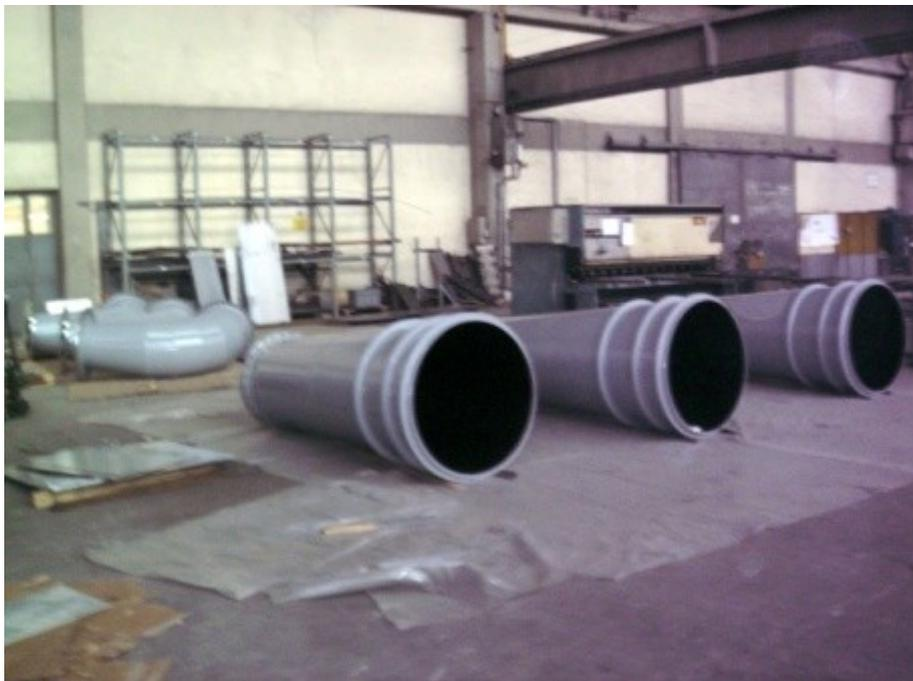
Figure 73. Manufactured draft tube parts according to final design
