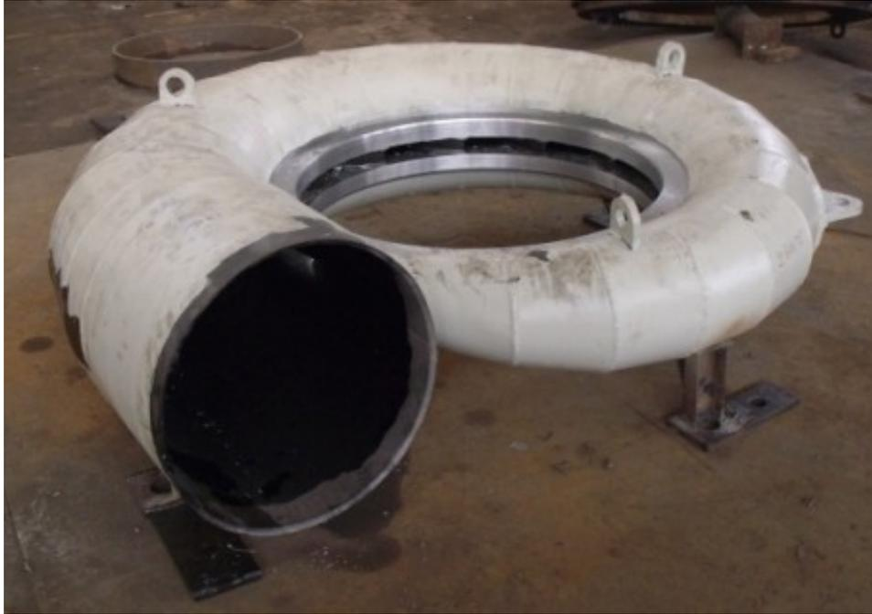
Figure 70. Manufactured spiral case according to final design
