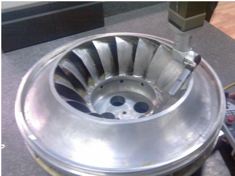
Figure 71. Manufactured turbine runner according to CFD design
