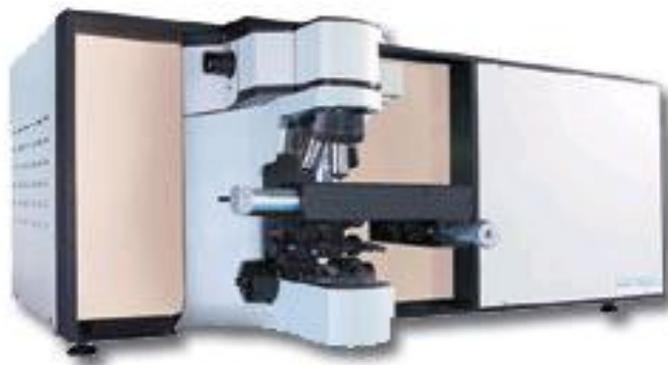
**Figure 2.3** Raman spectroscopy [67]
