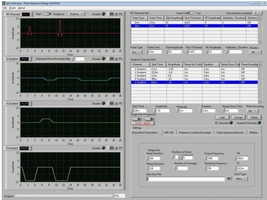
Figure 3.8 - Screenshot of the data acquisition front panel while spin echo pulse sequence is being applied.
