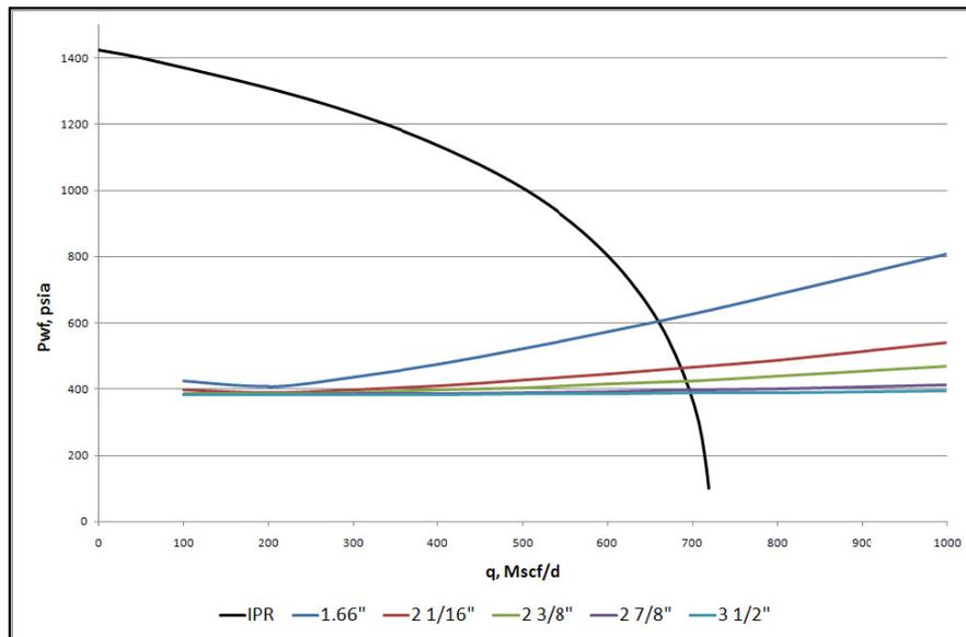
Figure 6.8 – Nodal Analysis for #28 with Different Tubing Sizes
