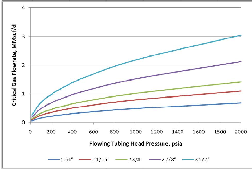
Figure 6.3 – Turner *et al.*'s Critical Flowrate for Different Tubing Sizes
