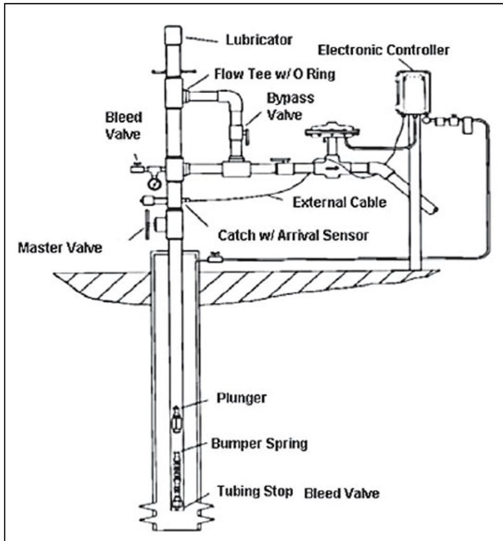
Figure 4.15 – A Typical Plunger Lift Installation<sup>10</sup>
