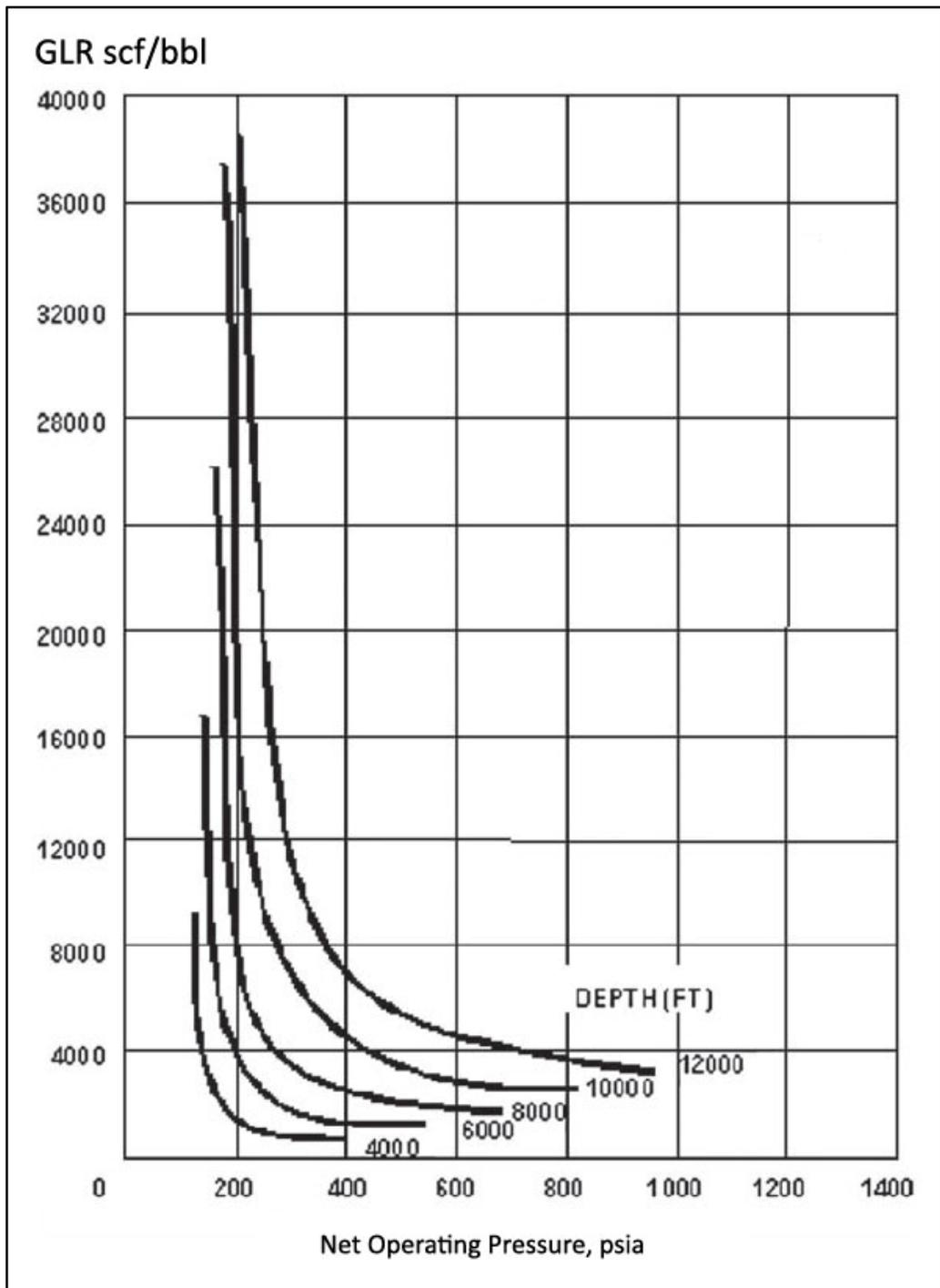
Figure B.3 – 2 1/2" Plunger Feasibility Chart for 2 7/8" Tubing<sup>15</sup>
