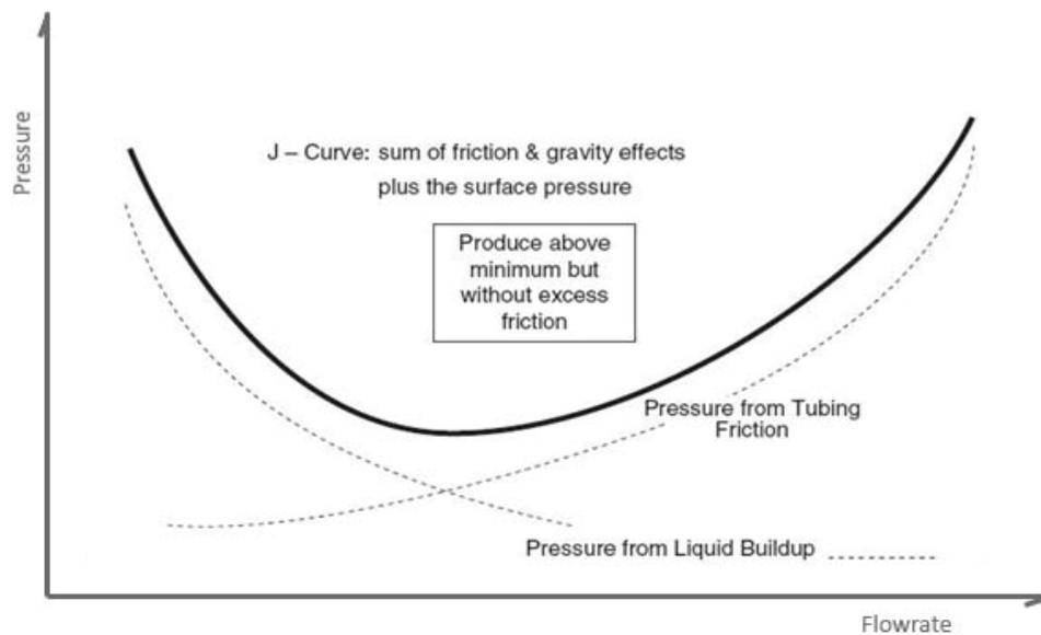
Figure 4.7 – Tubing Performance Curve<sup>10</sup>
