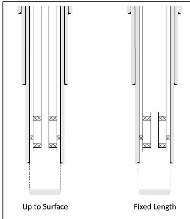
Figure 4.13 – Velocity String Application Schematic<sup>14</sup>
