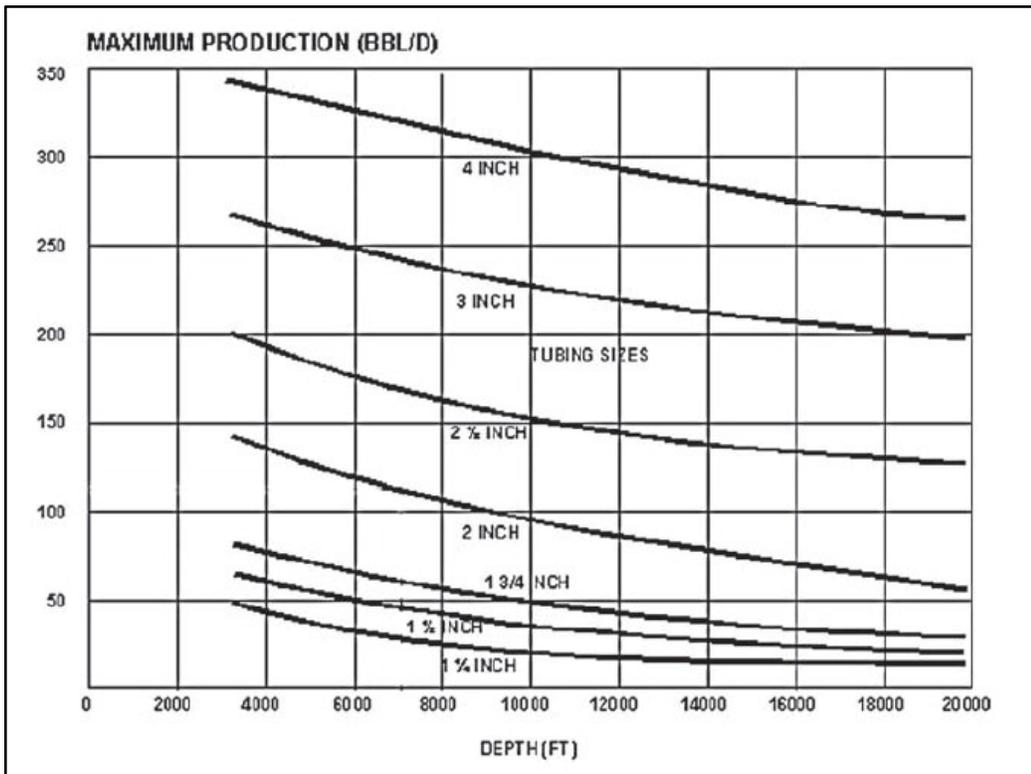
Figure B.1 – Liquid Production Chart for Plunger Lift<sup>16</sup>
