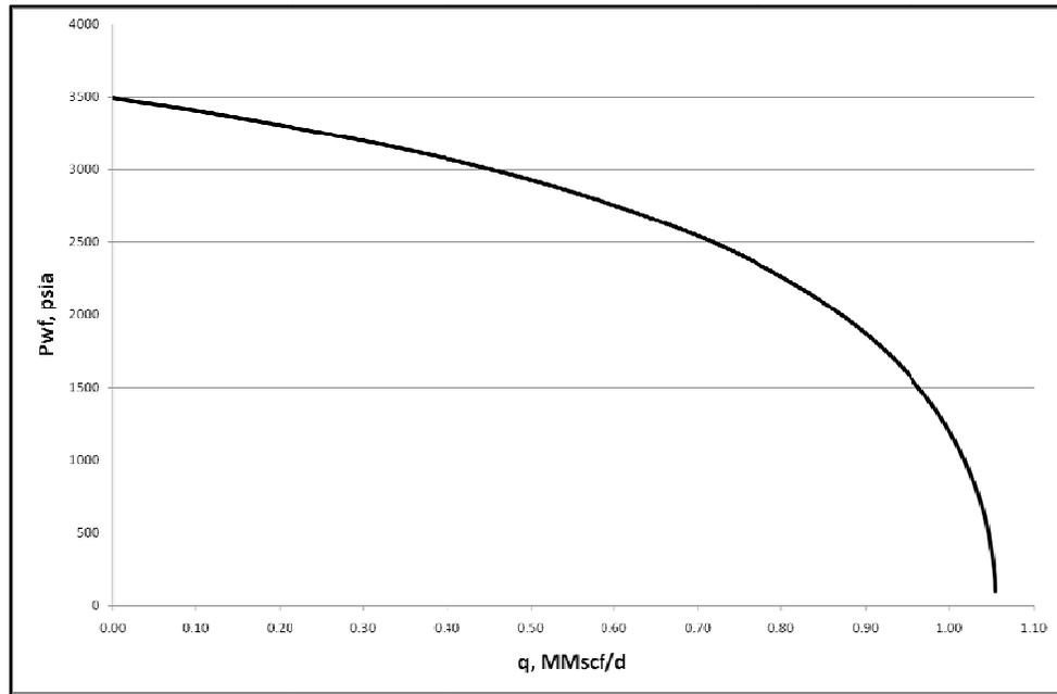
Figure C.1 – IPR curve of Well #10
