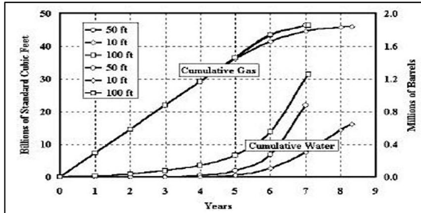
Figure 4.10 – Impact of Length of Perforation Interval on Cumulative Water and Gas Production in Years<sup>12</sup>
