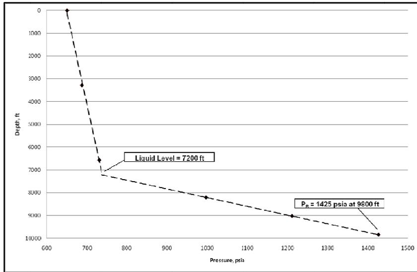
Figure 6.7 – Pressure Survey for #28 Showing Liquid Level
