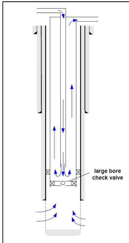
Figure 4.18 – Continuous Gas Lift Schematic<sup>14</sup>
