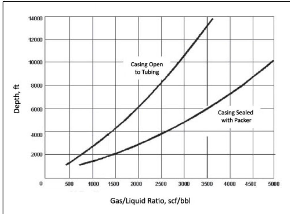
Figure 4.17 – Gas Requirement for Plunger Lift with or without Packer<sup>16</sup>
