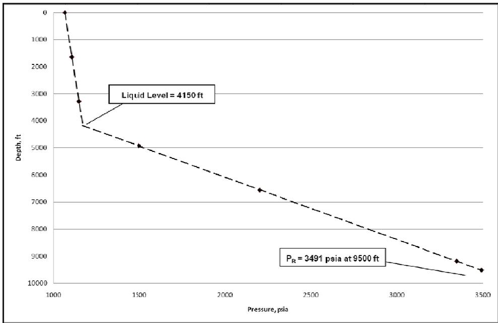
Figure 6.2 – Pressure Survey for #10 Showing Liquid Level
