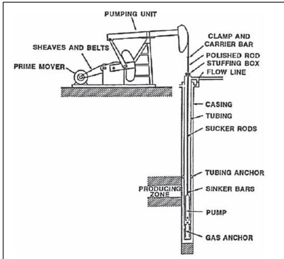
Figure 4.21 – A Simple Beam Pumping System<sup>12</sup>
