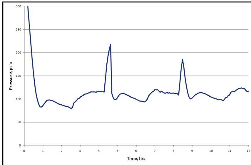
Figure 6.1 – Tubing Flowing Pressure Showing Erratic Flow in #10
