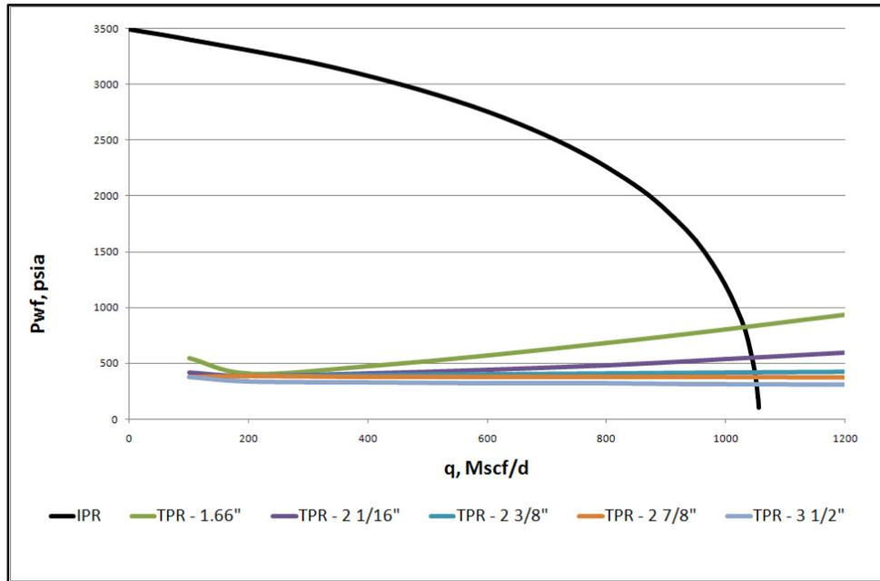
Figure 6.5 – Nodal Analysis for #10 with Different Tubing Sizes
