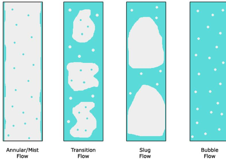
Figure 1.1 – Basic Profile of Multiphase Flow in the Well
