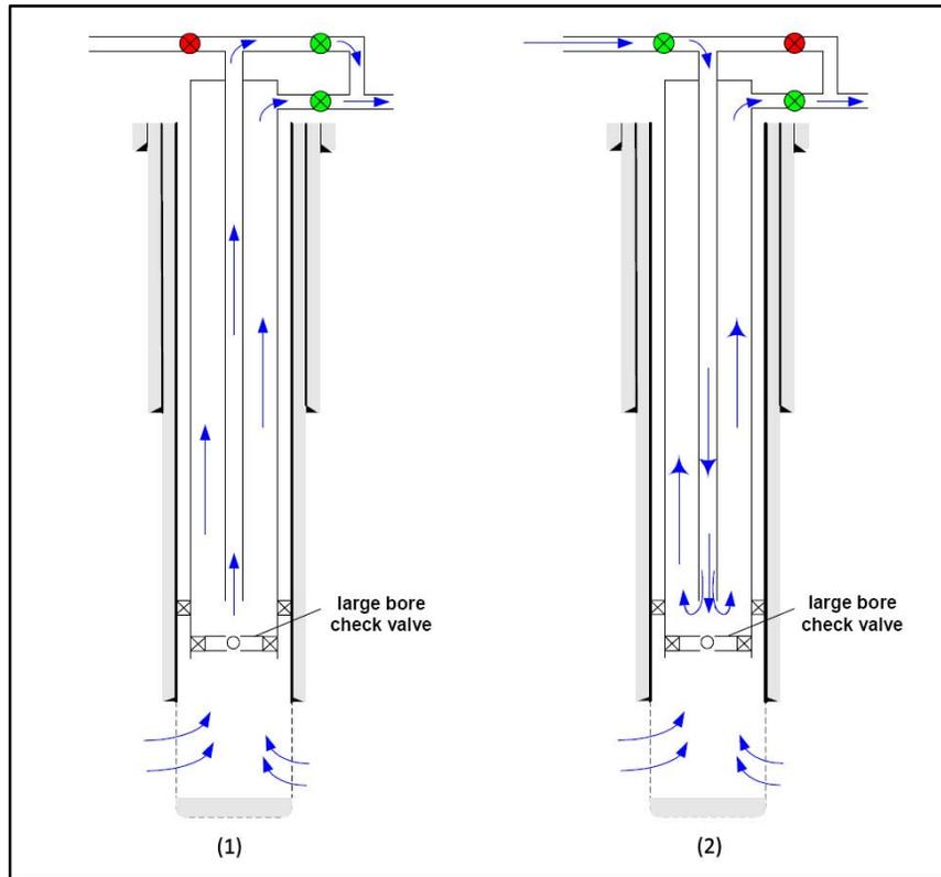
Figure 4.19 – Intermittent Flow Gas Lift Schematic<sup>14</sup>
