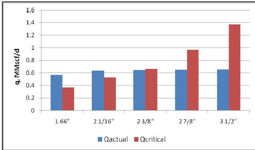
Figure 6.9 – Actual Rates vs. Critical Rates for #28
