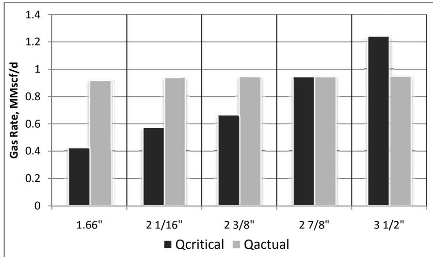
Figure 7.2 – Actual Rates vs. Critical Rates for #10
