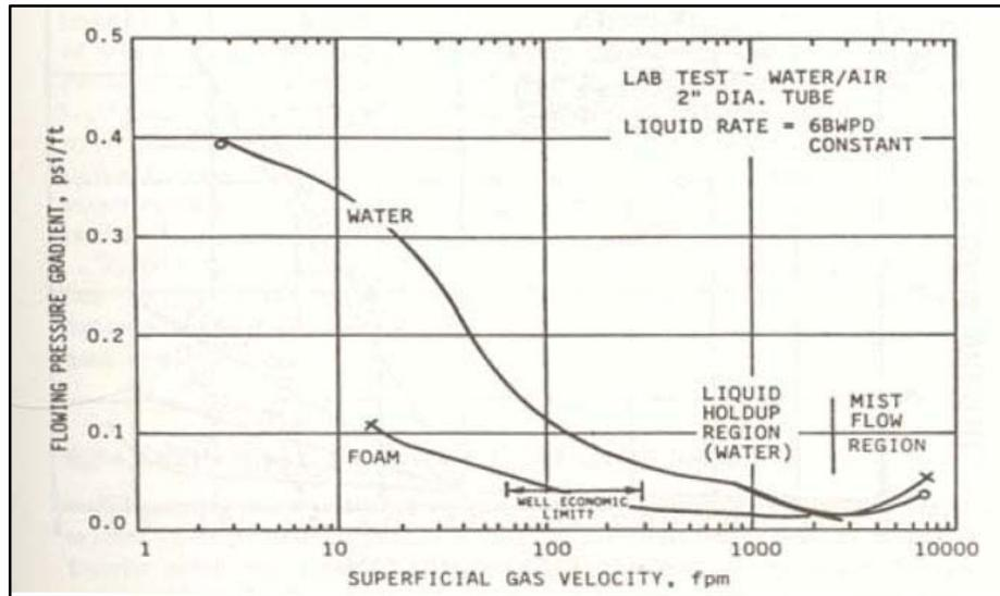
Figure 4.20 – Flowing Pressure Gradient of Water and Foam<sup>18</sup>
