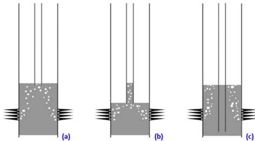
Figure 4.9 – The Effect of Setting the End of Tubing<sup>10</sup>
