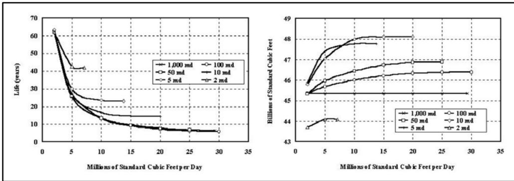
Figure 4.12 – Impact of Gas Production Rate and Permeability on Well Life (left) and Ultimate Gas Recovery (right)<sup>12</sup>
