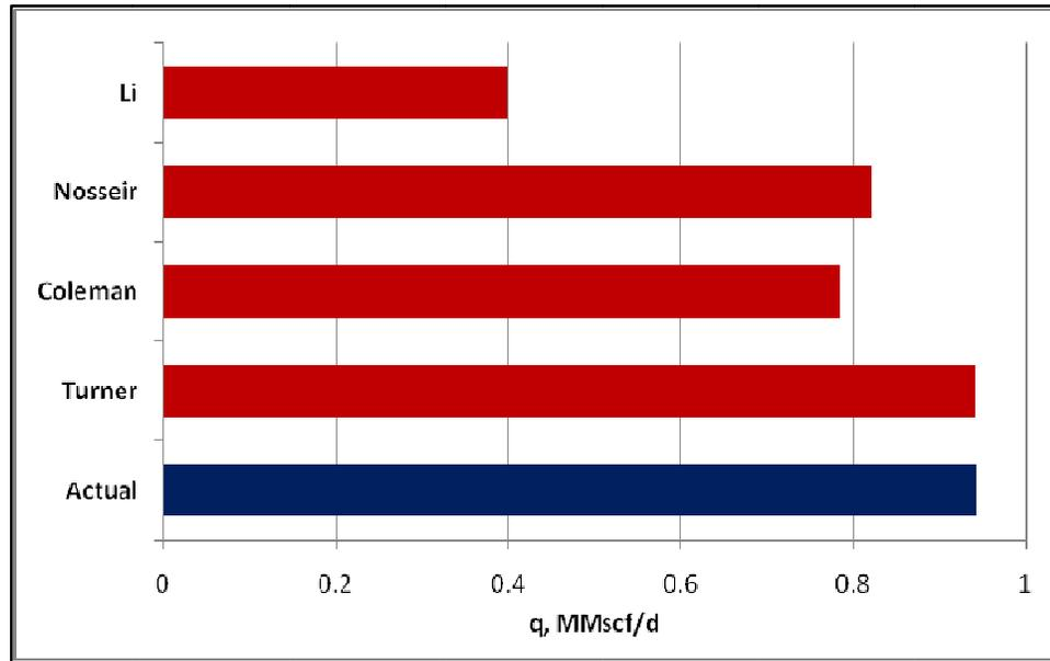
Figure 7.1 – Comparison of Critical Rate Equations
