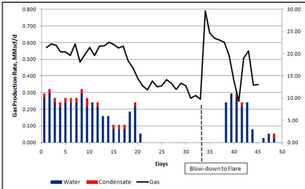
Figure 6.10 – Gas and Liquid Production Chart of #28
