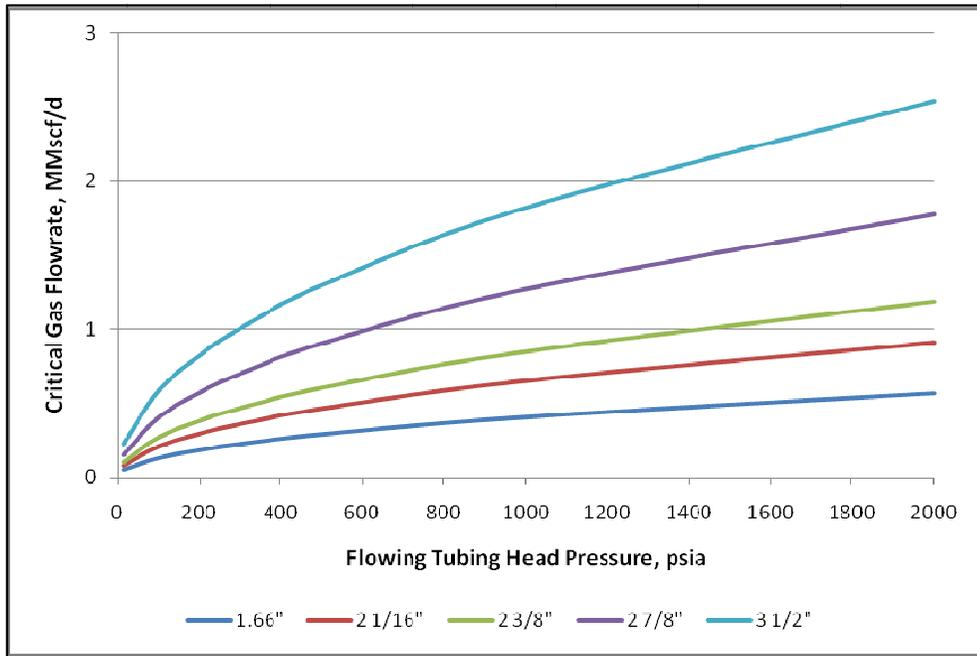
Figure 6.4 – Coleman *et al.*'s Critical Flowrate for Different Tubing Sizes
