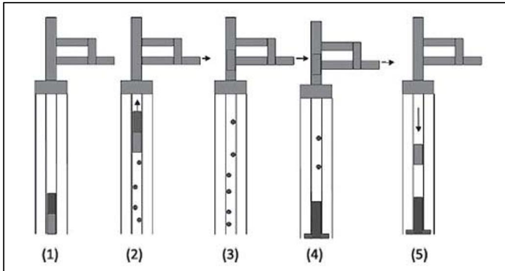
Figure 4.16 – A Simple Illustration of Plunger Lift Cycles<sup>10</sup>
