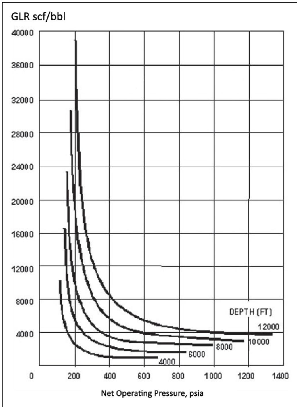
Figure B.2 – 2" Plunger Feasibility Chart for 2 3/8" Tubing<sup>15</sup>
