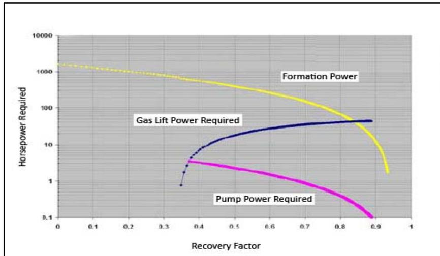
Figure 7.3 – Power vs. Recovery for Tight Reservoir<sup>22</sup>
