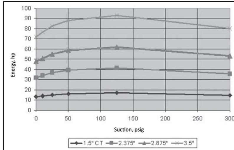
Figure 4.14 – Energy Required for Different Tubing Sizes to Stay above Critical Rate<sup>10</sup>
