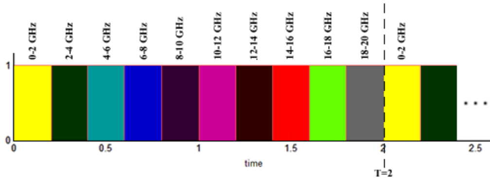
Figure 3-1: Simple periodic search strategy of a SHR for 10 frequency bands with T_{rcv} = 2
