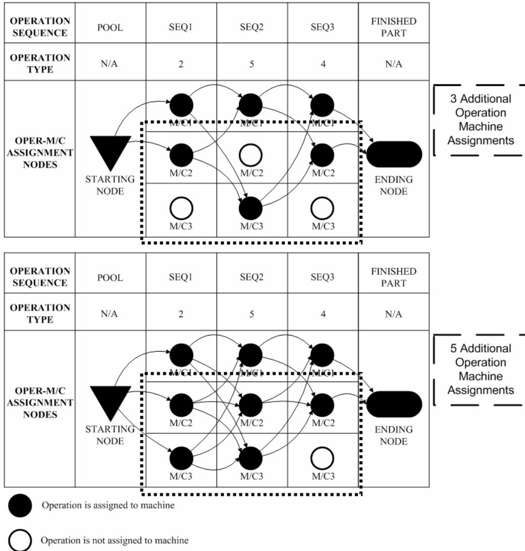
**Figure 4.3 Example Case with 3 and 5 Additional Operation-Machine Assignments**
