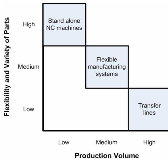
**Figure 3.1 Application Characteristics of FMSs, (reproduced from [23])**
