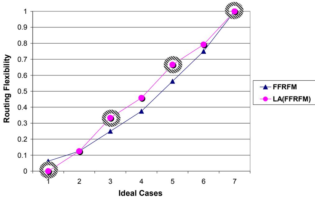
**Figure 4.6 PF Corrected Graph for a Shop with 4 Machines and a Part with 2 Operations**
