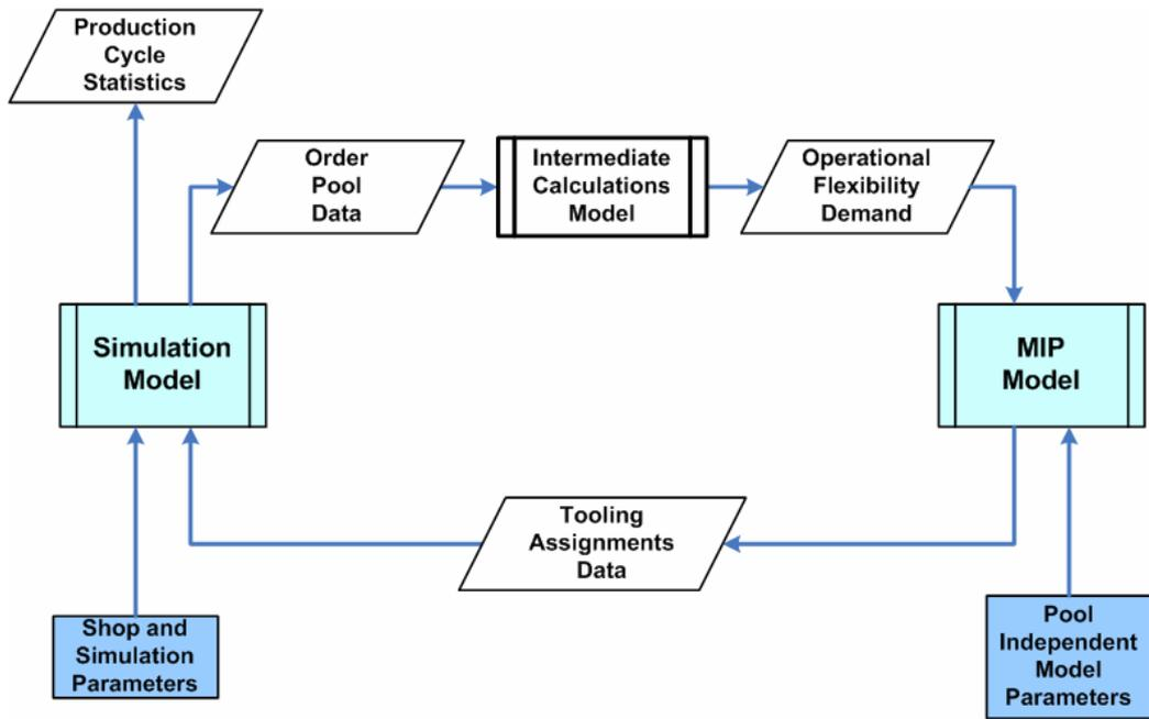
**Figure 4.15 The Combined Operation and the Interaction between the MIP and the Simulation Models**
