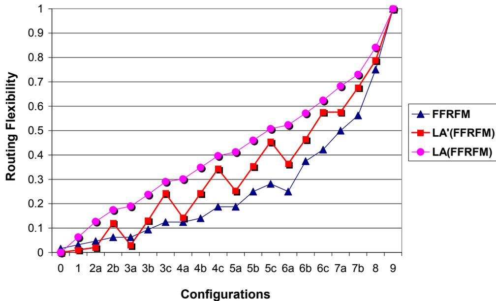
**Figure 4.8 PF Corrected Graph with the Two Methods for a Shop with 4 Machines and a Part with 3 Operations**
