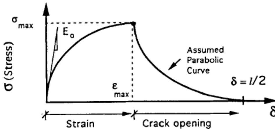
Figure 3.5: Tension curve of SIFCON [Naaman et al., (1993)]
