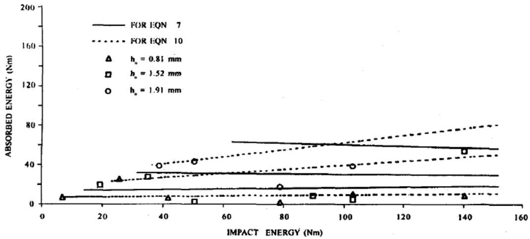
Figure 2.22: In obliquity of 30 degrees, absorbed energy versus impact energy [Khan et al., (2003)]
