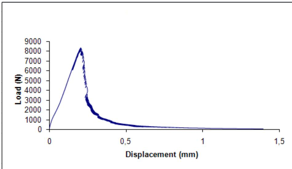
Figure 3.12: C55 Beam deflection test results
