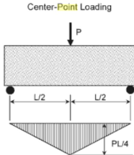
Figure 3.10: Moment diagram of center point loading [Lamond, Pielert , (2006)]
