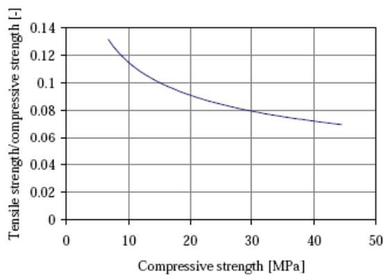
Figure 4.22: Tensile strength/compressive strength versus compressive strength [Nyström and Gylltoft, (2008)].
