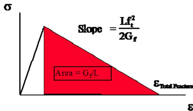
Figure 4.24: Crack softening in AUTODYN [AUTODYN, (2007)]
