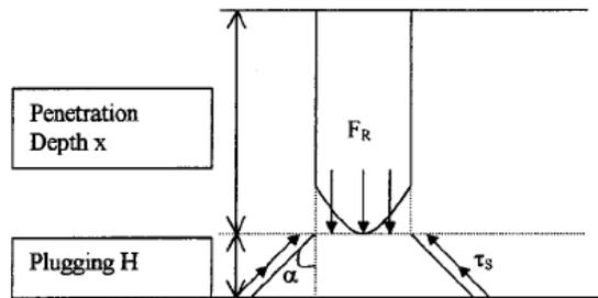
Figure 2.28: Scheme of the plugging work [Li and Tong, (2003)]
