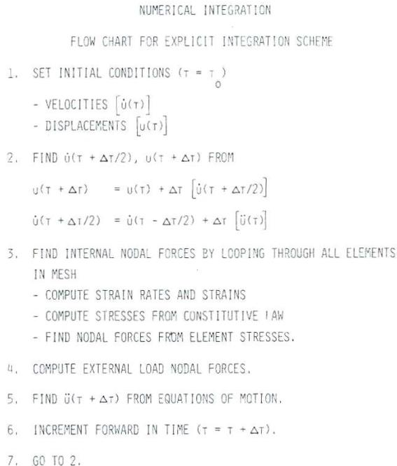
Figure 4.3: Implementation of the Central Difference Scheme [Zukas J.A., (2004)]
