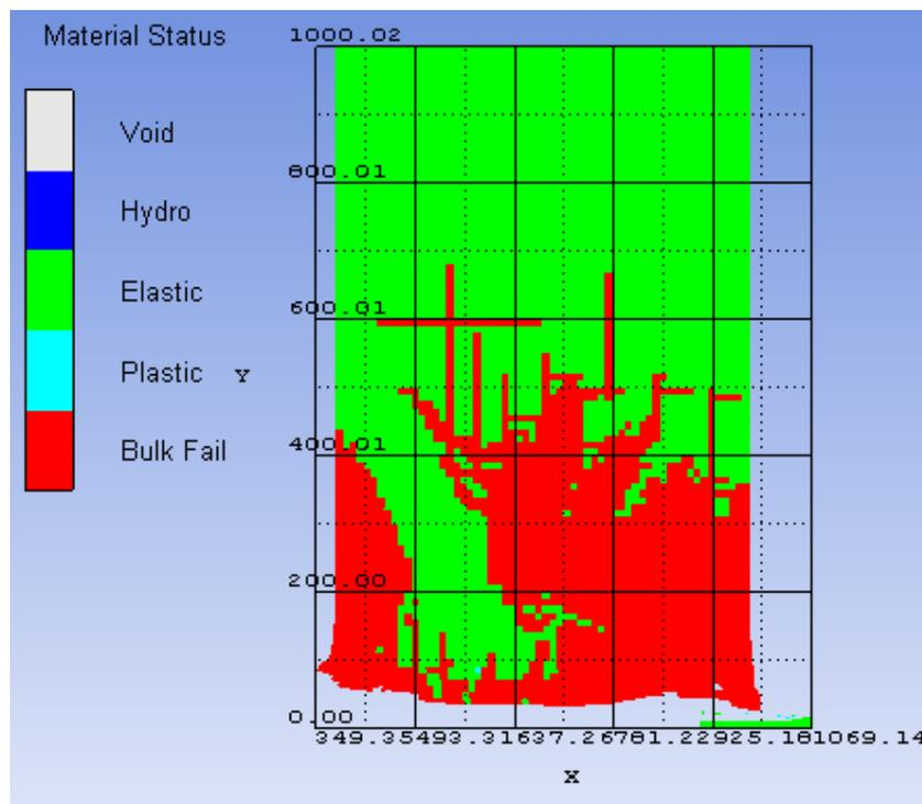
Figure 4.6: Result of projectile Impact on concrete target-10 mm mesh size
