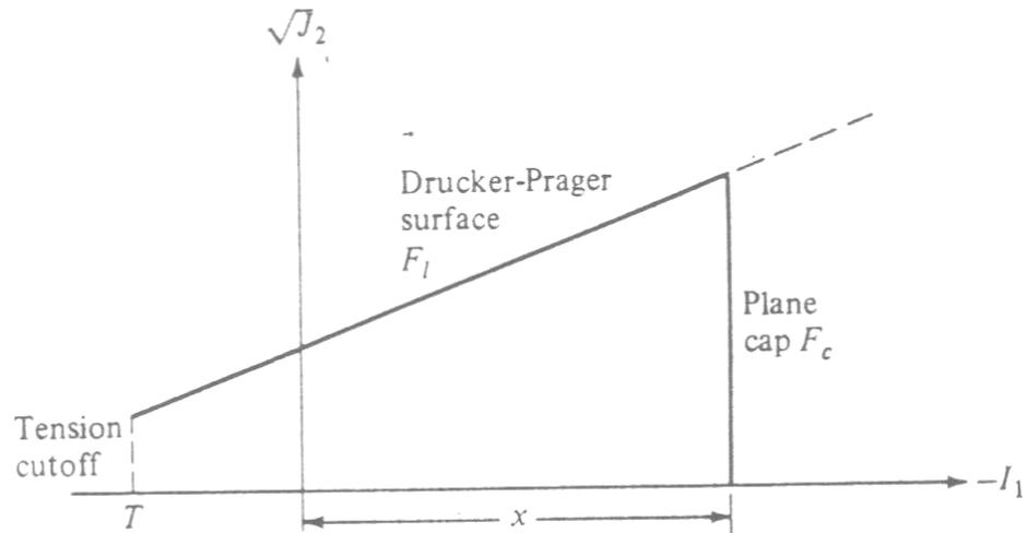
Figure 4.11: Drucker-Prager simple plane cap model [Chen, 1982]
