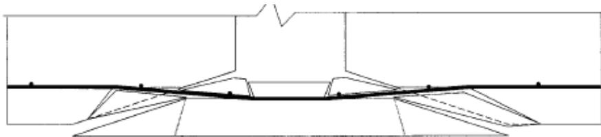
Figure 2.32: Failure process at rear faces [Dancygier, (1997)]
