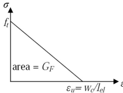
Figure 4.10: Linear crack softening relation used in AUTODYN
