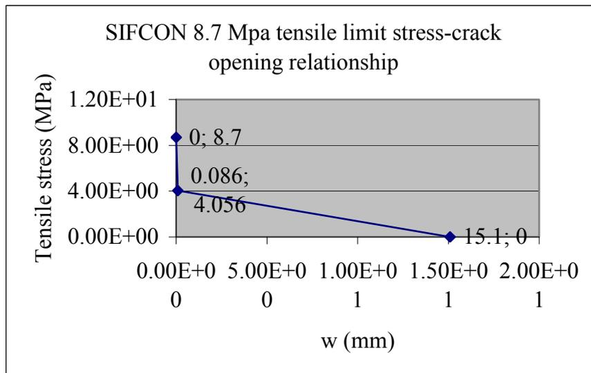
Figure 4.29: Bi-linear stress-crack opening relation for SIFCON (12 percent) with tensile strength 8.7 MPa with the method in [Nyström, (2008)]
