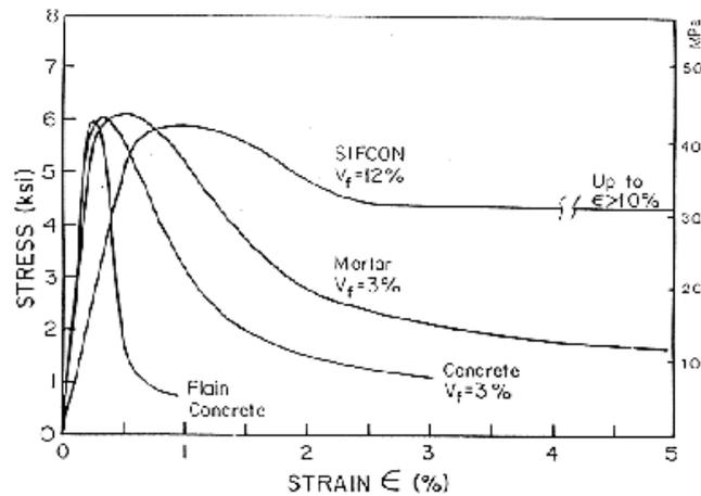
Figure 2.31: Comparison of experimentally observed stress-strain curves of plain concrete, fiber reinforced concrete and mortar, and SIFCON [Li et al., (1989)]
