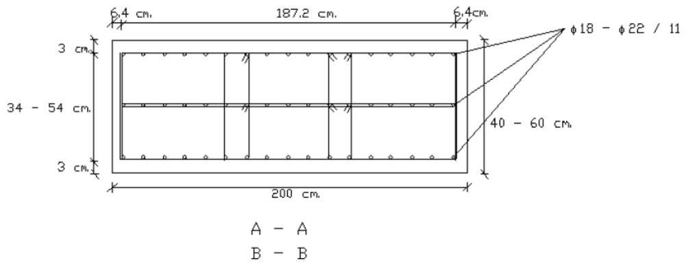
Figure 3.7: Cross-sectional view of the reinforcement configuration
