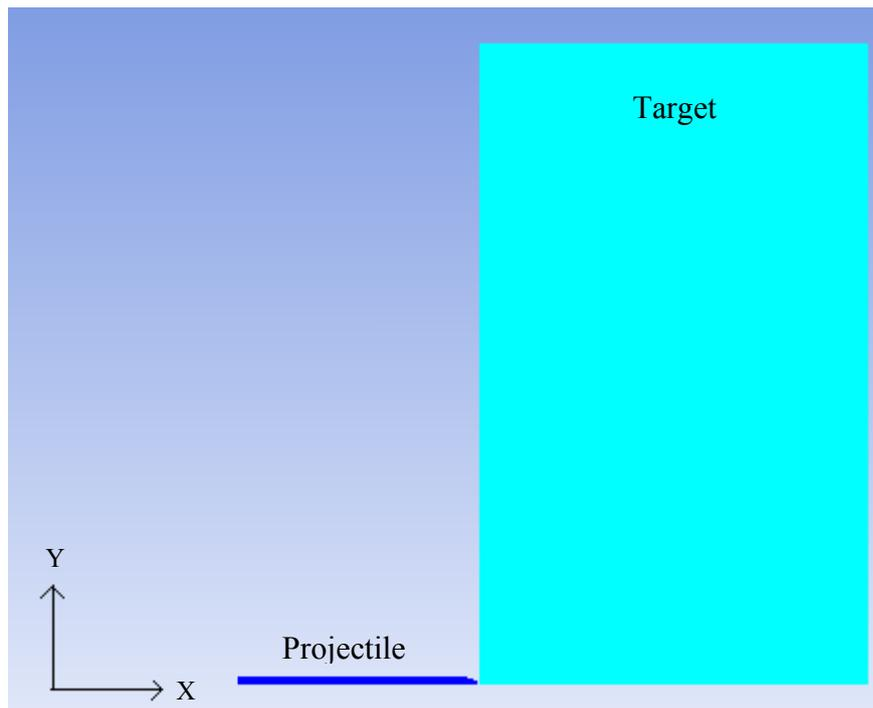
Figure 4.1: Undeformed projectile- first SIFCON wall before strike
