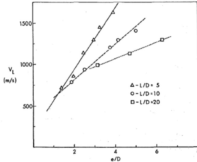
Figure 2.5: Ballistic limit versus normalized target thickness for different L/D ratios [Zukas et al., (1982)]
