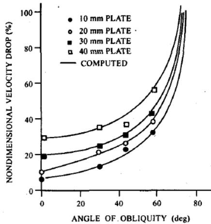
Figure 2.24: Angle of obliquity versus non-dimensional velocity drop for aluminum target [Madhu et al., (2003)]
