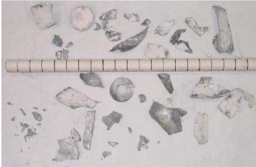
Figure 2.7: CRH=0.5 projectile pieces from the 721 m/s experiment. [Phillabaum II et al.,(2008)]
