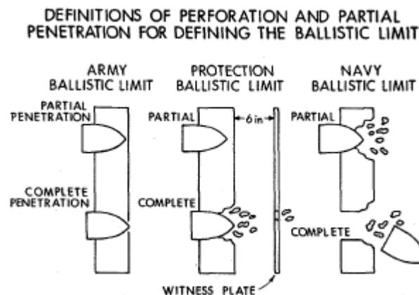
Figure 2.1: Different approaches for complete penetration [Zukas et al., (1982)]
