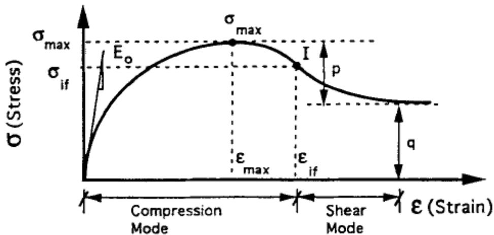
Figure 3.4: Compression curve of SIFCON [Naaman et al., (1993)]
