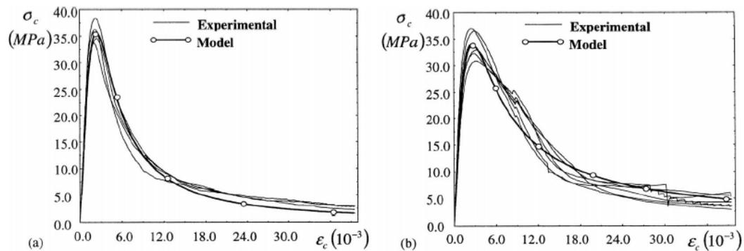
Figure 3.1: Comparison of experimental and analytical SFRC compression curves
