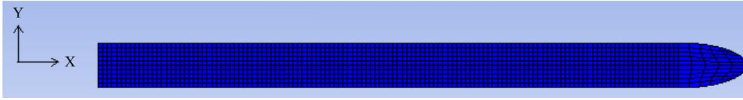
Figure 4.5: Full view of the projectile mesh by the help of mirror in y-plane option
