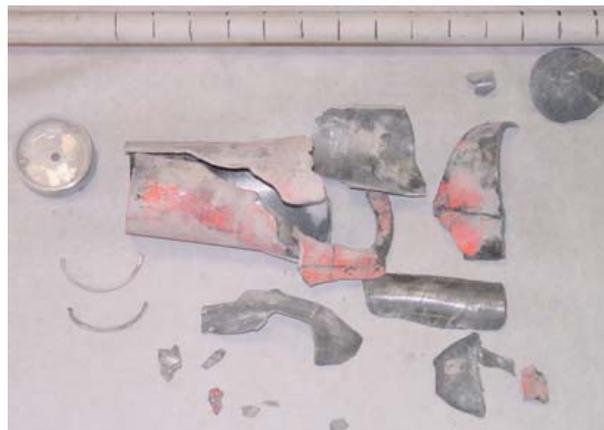
Figure 2.6: CRH=0.5 projectile pieces from the 529 m/s experiment. [Phillabaum II et al.,(2008)]
