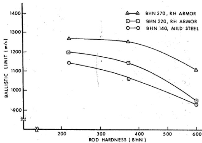
Figure 2.13: Outcomes of the experiments for ballistic limit versus rod hardness [Zukas et al., (1982)]
