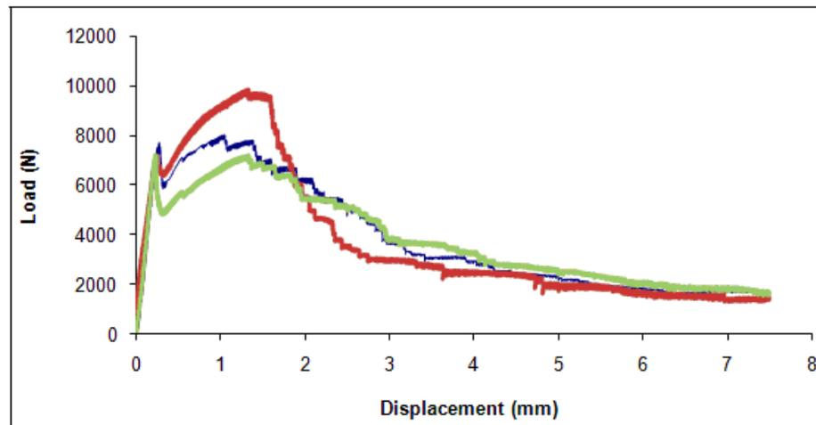
Figure 3.13: SFRC Beam deflection test results
