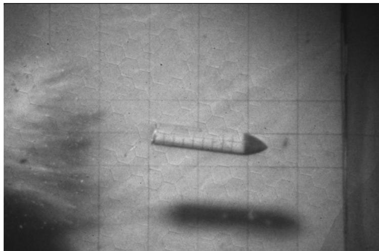
Figure 2.9 : High-speed camera image of the CRH=2 projectile after exiting the DRC target in the 707-m/s experiment [[Phillabaum II et al.,(2008)]
