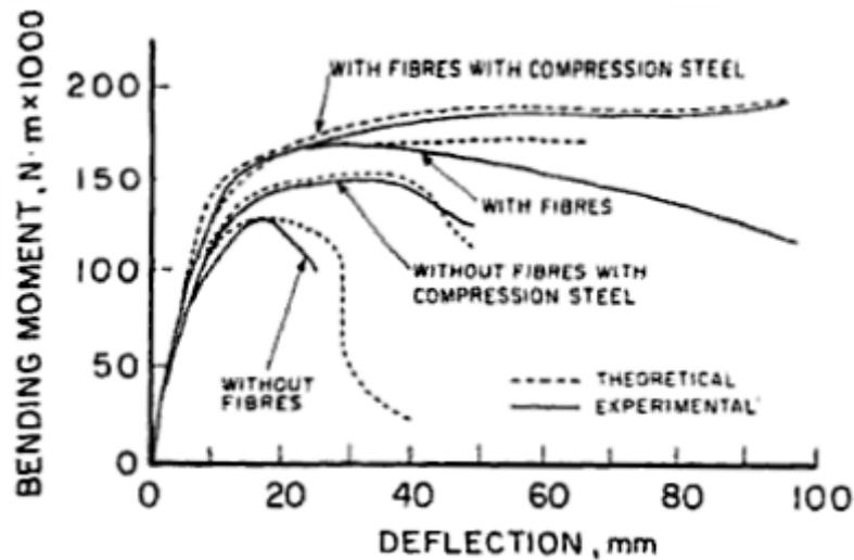
Figure 2.36: Bending moment versus deflection for different concrete forms[Bentur and Mindess, (2006)]
