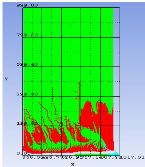
Figure 4.8: Result of projectile Impact at concrete target-3 mm mesh size
