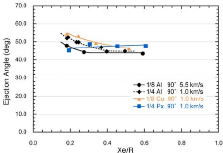
Figure 2.15: Result of experiments in terms of ejection angles versus ejection position scaled by the average final crater radius [Anderson and Schultz, (2005)]
