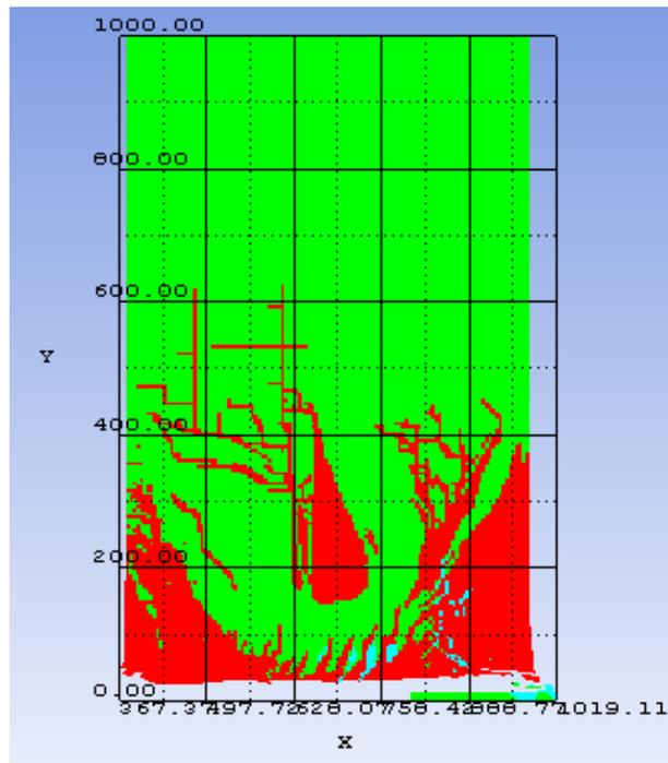
Figure 4.7: Result of projectile Impact at concrete target-5 mm mesh size
