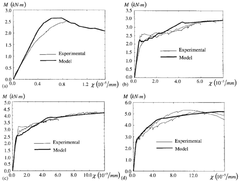
Figure 3.3: Moment-curvature relationship of slab strips reinforced with different amounts of fibers: (a) 0 kg/m<sup>3</sup>; (b) 30 kg/m<sup>3</sup>; (c) 45 kg/m<sup>3</sup>; (d) 60 kg/m<sup>3</sup> [Barros and Figueiras (1999)]
