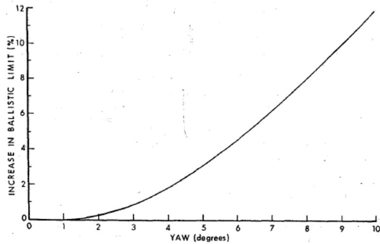
Figure 2.26: Effect of yaw on ballistic limit [Zukas et al., (1982)]
