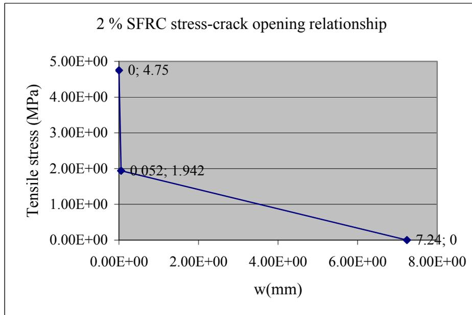
Figure 4.26: Bi-linear stress-crack opening relation for steel fiber reinforced concrete with the method in [Nyström, (2008)]
