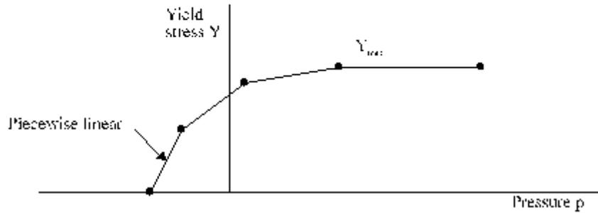
Figure 4.12: Piecewise yield stress versus pressure model used in AUTODYN
