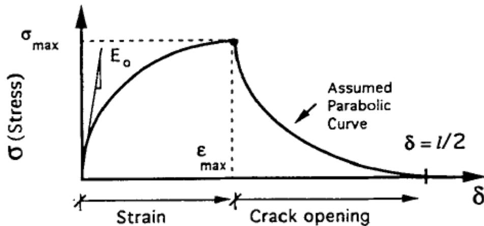
Figure 4.27: Schematic representation of the stress-elongation curve of SIFCON in tension [Naaman et al. (1993)]
