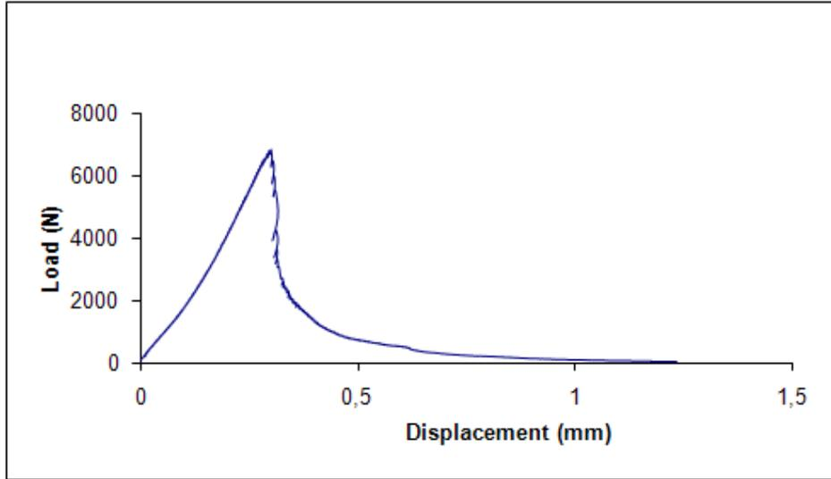
Figure 3.11: C30 Beam deflection test results
