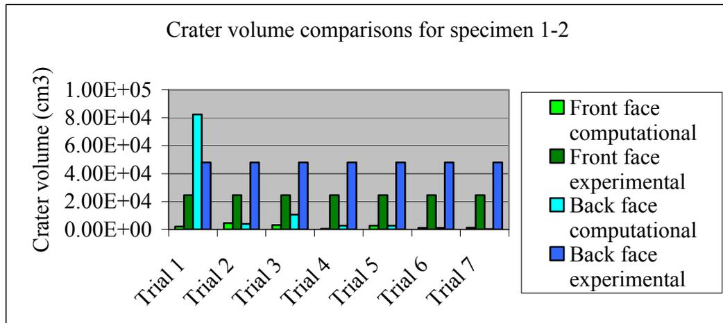
Figure 5.33: Crater volume Comparisons for Specimen 1-2
