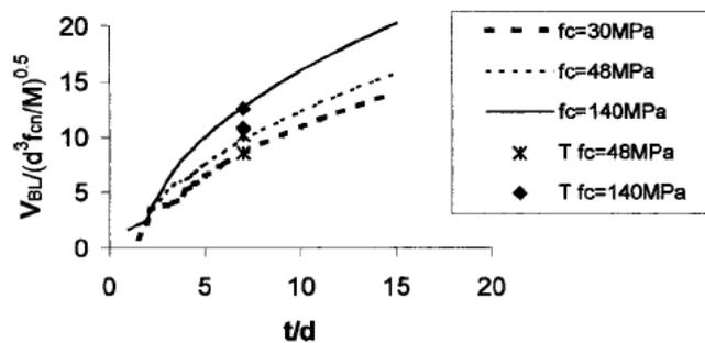
Figure 2.29 Effect of concrete strength on dimensionless ballistic limit [Hanchak et al., (1992)]
