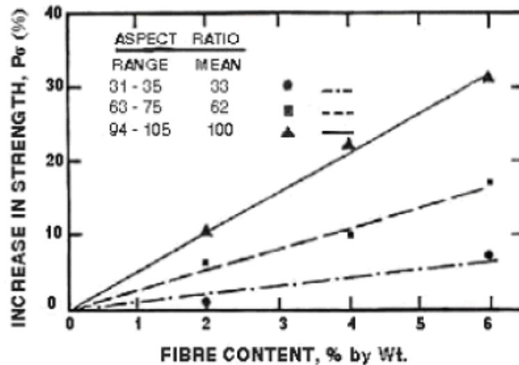
Figure 4.20: Increase in strength according to fiber content and aspect ratio
