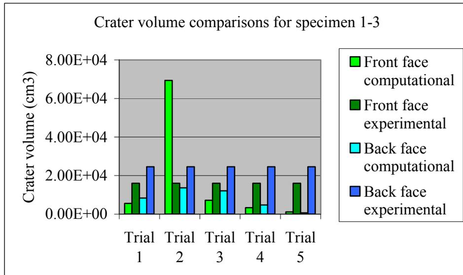
Figure 5.31: Crater volume comparisons for trials of Specimen 1-3
