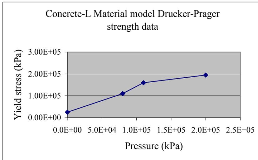
Figure 4.13: Concrete-L Drucker-Prager strength data in terms of yield stress versus pressure, [AUTODYN, (2007)]
