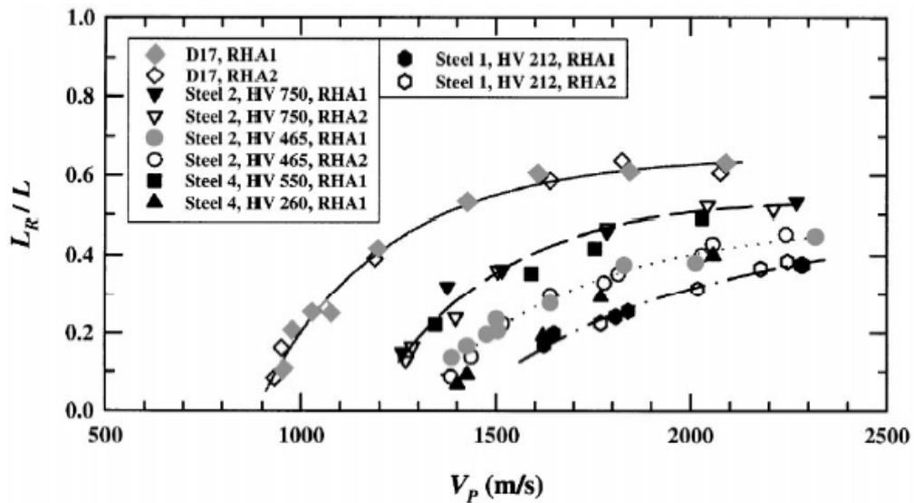
Figure 2.11: Normalized residual length versus impact velocity [Anderson Jr. et al., (1999)]
