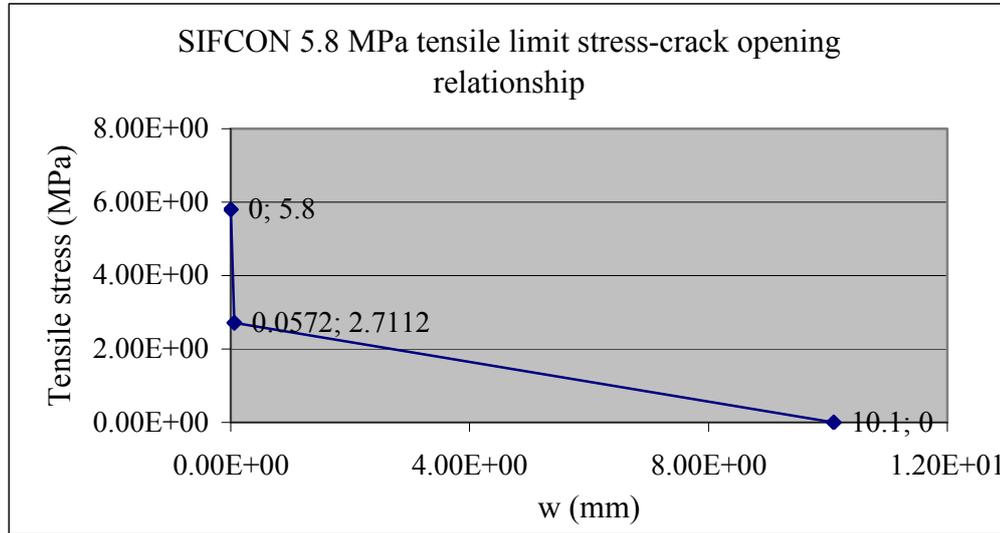
Figure 4.28: Bi-linear stress-crack opening relation for SIFCON (12 percent) with tensile strength 5.8 with the method in [Nyström, (2008)]
