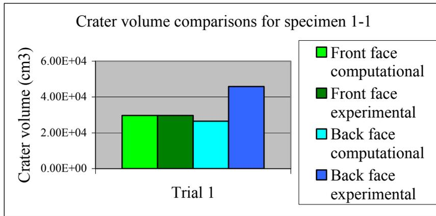
Figure 5.32: Crater volume Comparisons for Specimen 1-1
