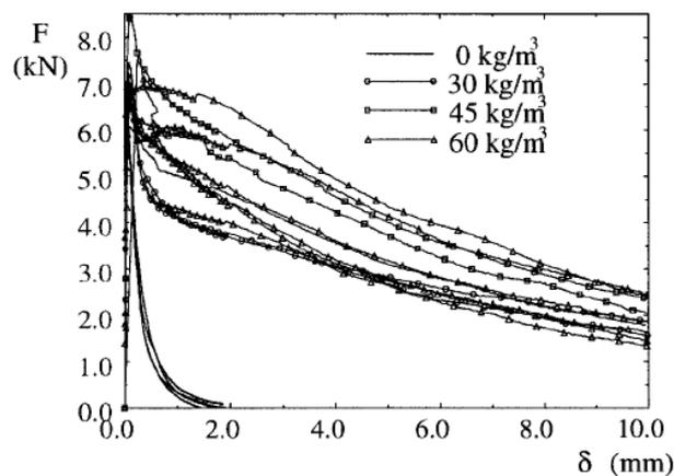
Figure 3.2: Load-displacement relationship obtained from a group of specimen in three-point bending tests of notched beams, [Barros and Figueiras (1999)]
