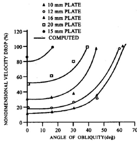
Figure 2.23: Angle of obliquity versus non-dimensional velocity drop for mild steel target [Madhu et al., (2003)]
