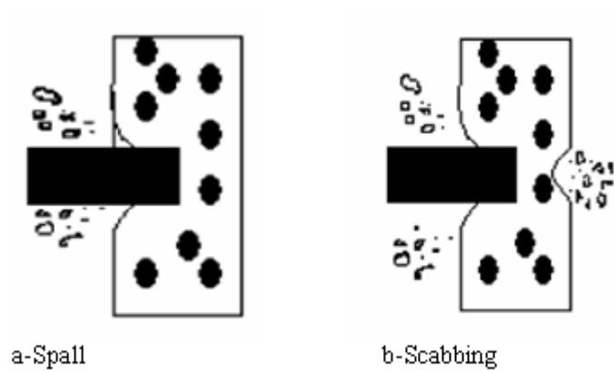
Figure 2.3: Possible spalling and scabbing views [Lia et al., (2005)]
