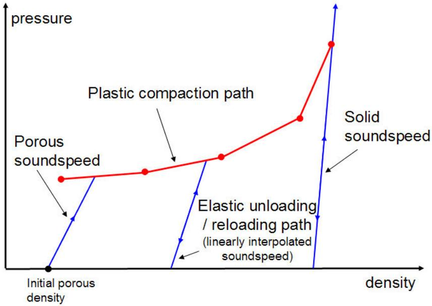
Figure 4.16: The Piecewise-Linear Porous EOS Model, [AUTODYN, (2007)]
