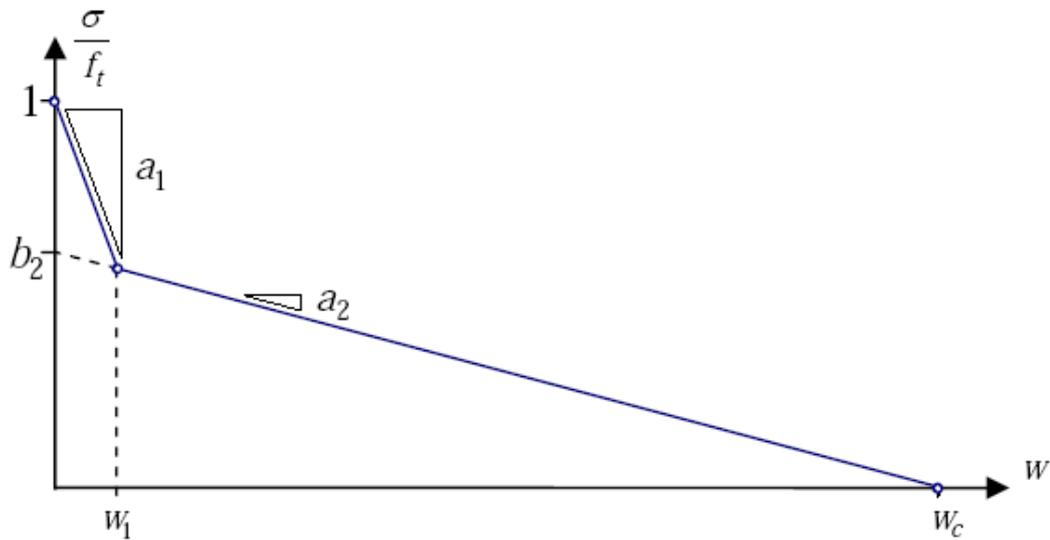
Figure 4.25: Bi-linear stress-crack opening relation for steel fiber reinforced concrete [Nyström, (2008)]
