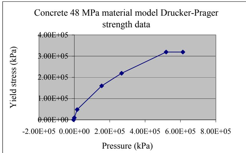
Figure 4.14: Concrete 48 MPa material model Drucker-Prager strength data in terms of yield stress versus pressure, [Tham, (2005)]
