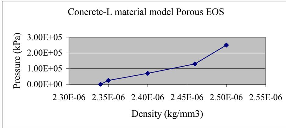
Figure 4.17: Concrete-L material model Porous EOS data in terms of pressure versus density [AUTODYN, (2007)]
