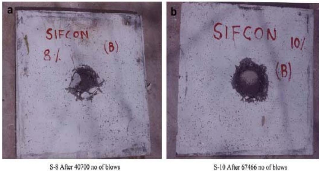
Figure 2.34: Failed SIFCON specimens without conventional reinforcement- a-) containing 8 percent fiber b-) containing 10 percent fiber [Rao et al., (2009)]
