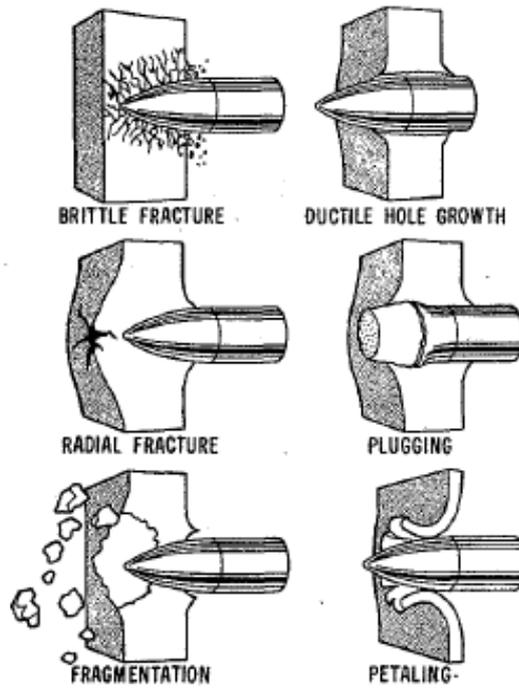
Figure 2.2: Images of possible failure models [Zukas et al., (1982)]
