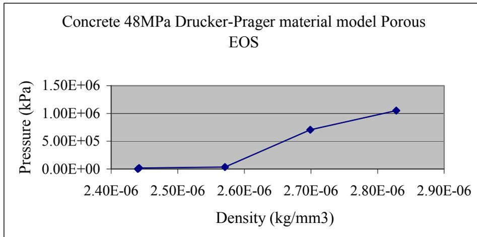
Figure 4.18: Concrete-L 48 MPa material model Porous EOS data in terms of pressure versus density, [Tham, (2005)]
