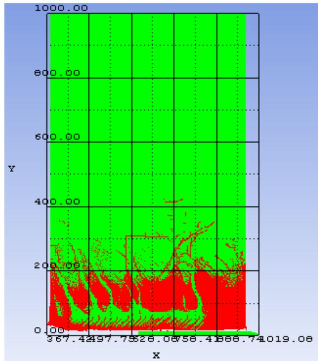
Figure 4.9: Result of projectile Impact at concrete target-2 mm mesh size
