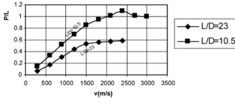
Figure 2.4: Efficiency of the penetration versus impact velocity for different L/D ratios [Daneshjou et al. (2005)]
