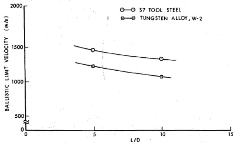
Figure 2.17: Experimental outcomes for same weight, different density projectiles in terms of ballistic limit versus L/D [Zukas et al., (1982)]
