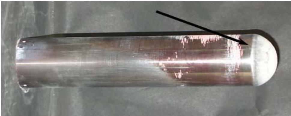
Figure 2.8: CRH=0.5 projectile pieces from the 400 m/s experiment. [Phillabaum II et al.,(2008)]
