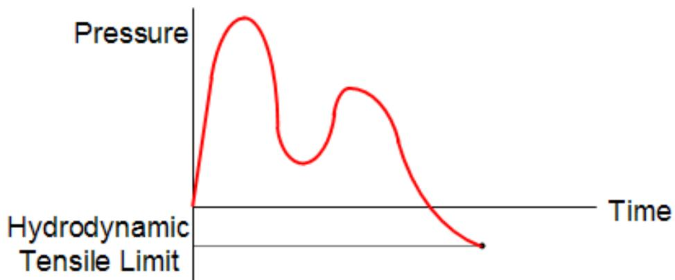
Figure 4.19: Hydrodynamic tensile failure model [AUTODYN, (2007)]
