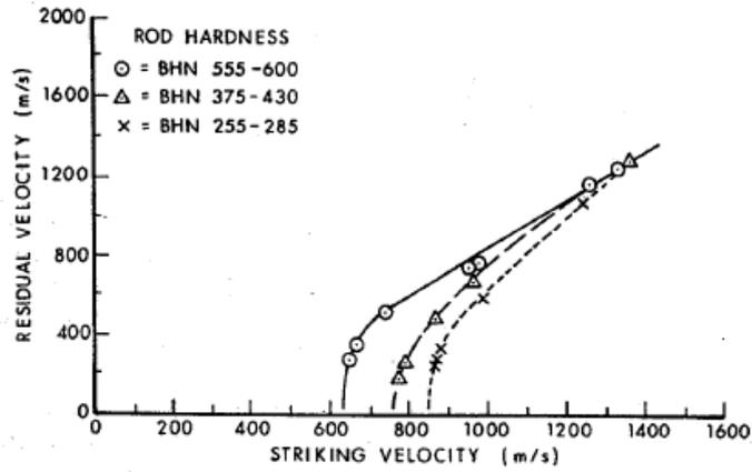
Figure 2.12: Outcomes of the experiments for residual velocity versus striking velocity for different rod hardness [Zukas et al., (1982)]
