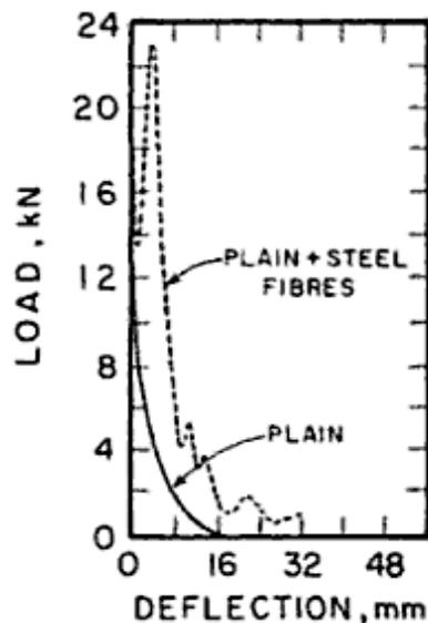
Figure 2.35: Behavior of plain concrete and SFRC under impact loading -drop-weight machine [Bentur and Mindess, (2006)]
