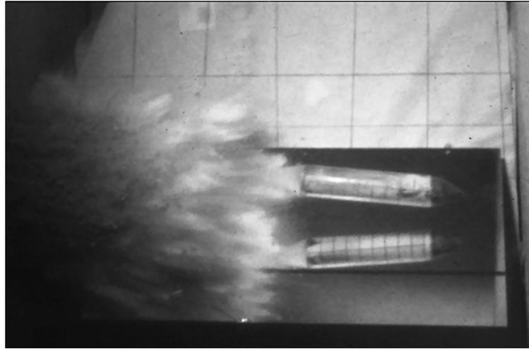
Figure 2.10: High-speed camera image of the CRH=2 projectile after exiting the DRC target in the 784-m/s experiment [[Phillabaum II et al.,(2008)]]
