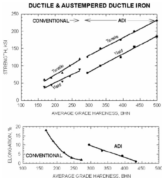
Figure 2.30 Differences of austempered and conventional ductile iron [Warrick et al. (2000)]
