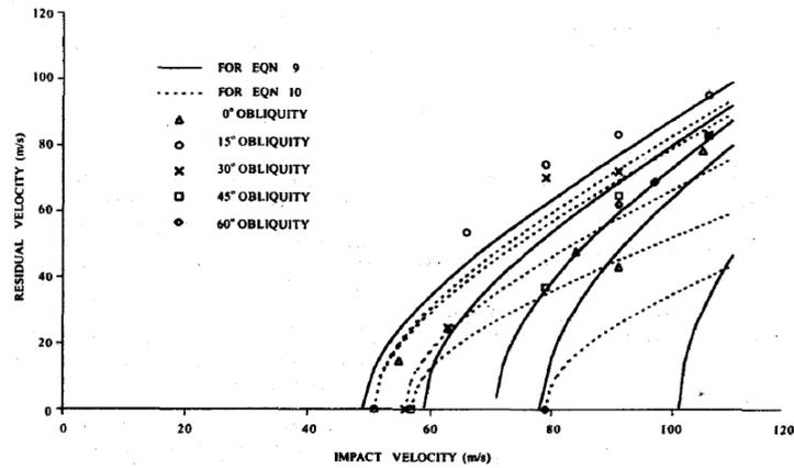
Figure 2.20: Outcomes of the experiments for residual versus impact velocity point of view [Khan et al., (2003)]
