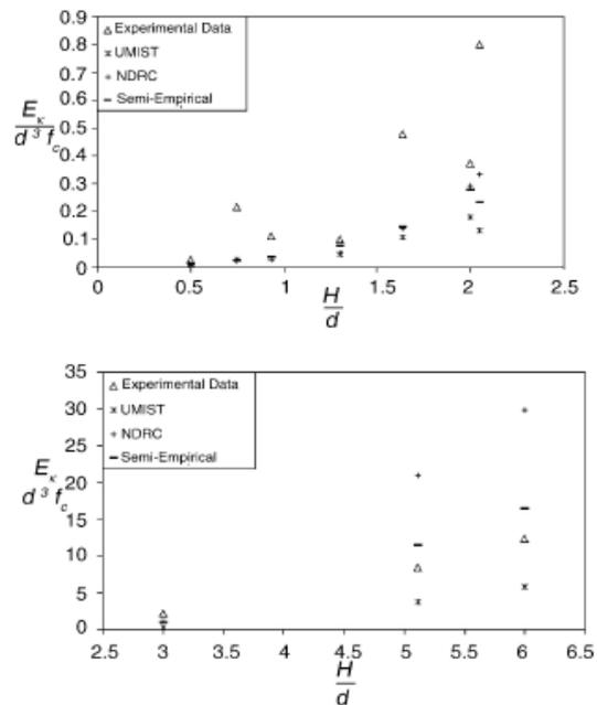
Figure 2.19: Comparison of these empirical, semi-empirical formulae outcomes with experimental values in Bainbridge, (1988)[ Li et al., (2006)]
