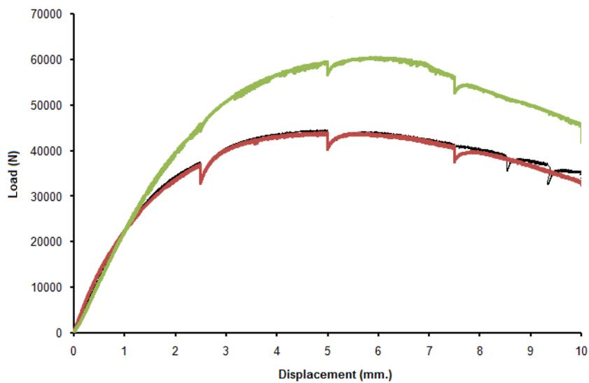
Figure 3.14: SIFCON Beam deflection test results
