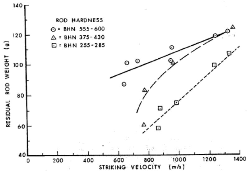
Figure 2.14: Outcomes of the experiments for residual rod weight versus striking velocity [Zukas et al., (1982)]
