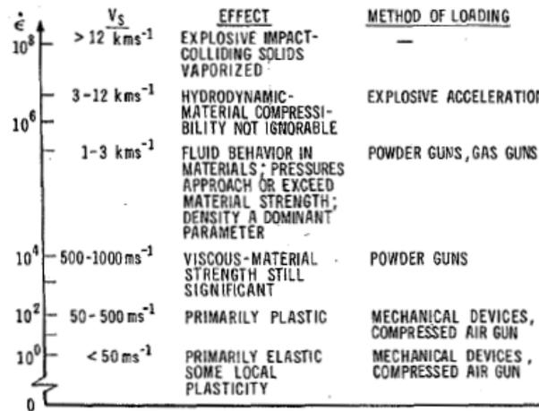
Figure 2.18: Effect of impact with method of loading and strain rate [Zukas et al., (1982)]
