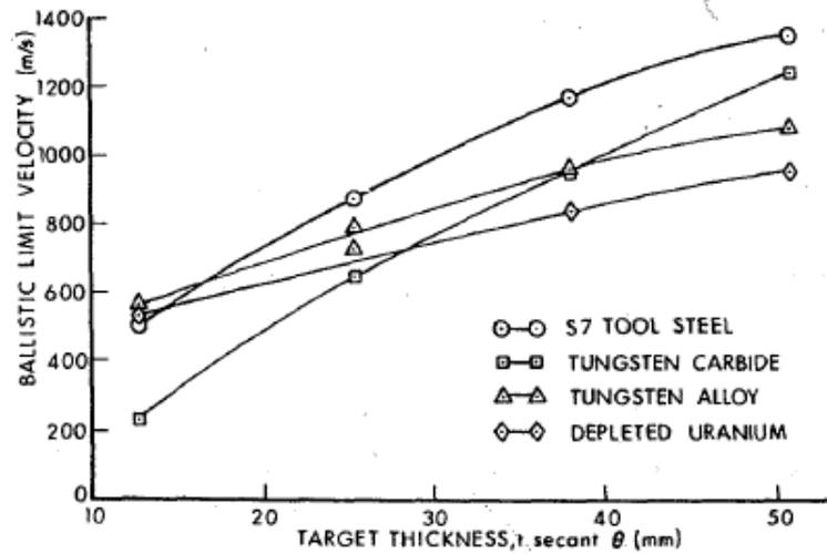
Figure 2.16: Experiment results for ballistic limit versus target thickness for different densities [Zukas et al., (1982)]
