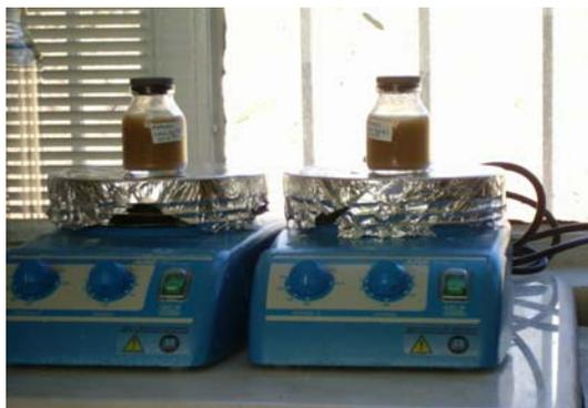
Figure 3.5 Ammonium ion removal in the dark fermenter effluent of sugar-beet thick juice molasses using clinoptilolite.
