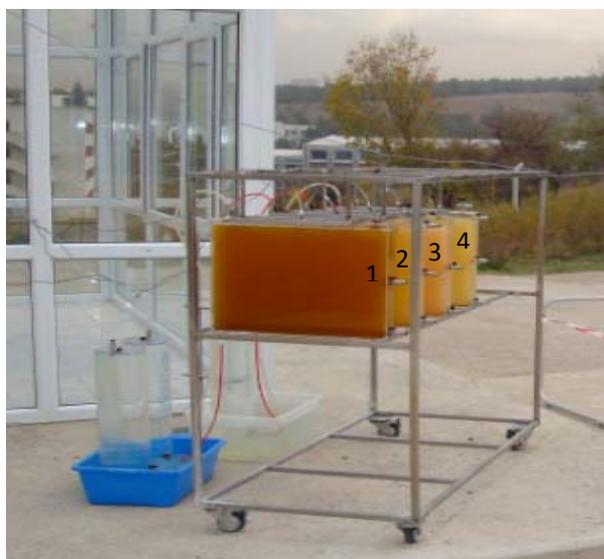
Figure 3.3 The outdoor hydrogen production experimental setup. (1, 2) *Rhodobacter capsulatus* YO3 (Hup<sup>-</sup>), (3) Heat adapted *Rhodobacter capsulatus* (DSM 1710) and (4) *Rhodobacter capsulatus* (DSM 1710).
