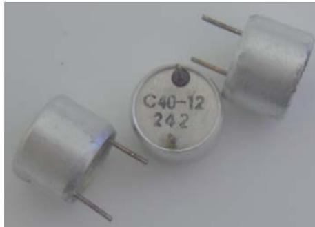
**Figure 3-3** C40-12 series ultrasonic transducers
