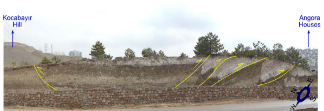
Figure 2.5 Photograph illustrating the geological units and positions of normal faults on the east bank of the road.
