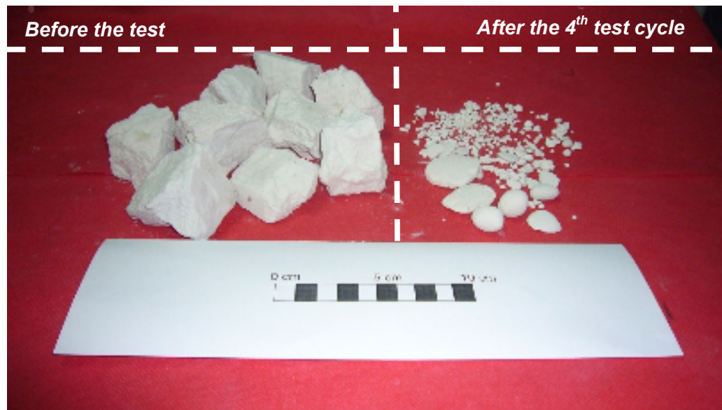
Figure 3.9 Alteration in shape and size of the tuffite lumps after the 4 th test cycle of slake durability test in distilled water.
