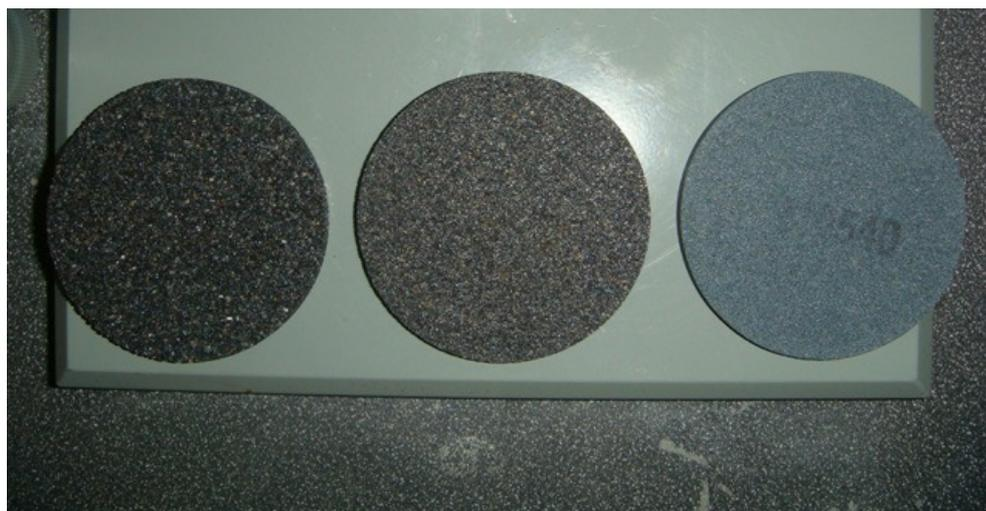
**Figure 4-2: Ceramic Disks (left to right 35μ, 60 μ, and 90 μ)**
