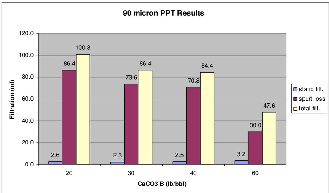
**Figure C-5: Effect of Concentration of CaCO<sub>3</sub> B (90 μ Ceramic Disks)**
