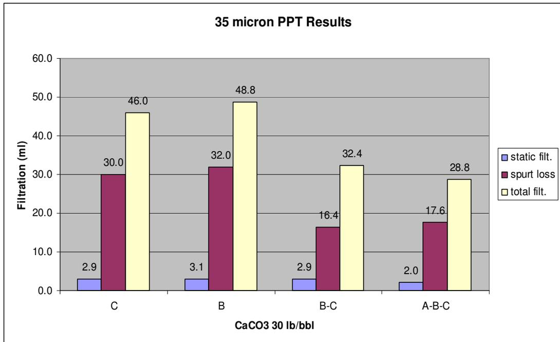
**Figure 5-10: Effect of particle size for 35  $\mu$  ceramic disks**
