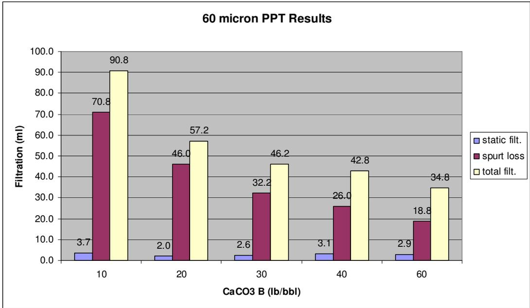
**Figure C-4: Effect of Concentration of CaCO<sub>3</sub> B (60 μ Ceramic Disks)**
