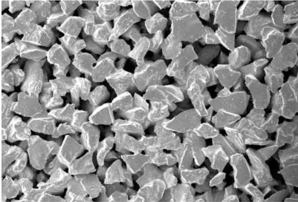
**Figure 5-5: 60 μ Ceramic Disk before PPT**
