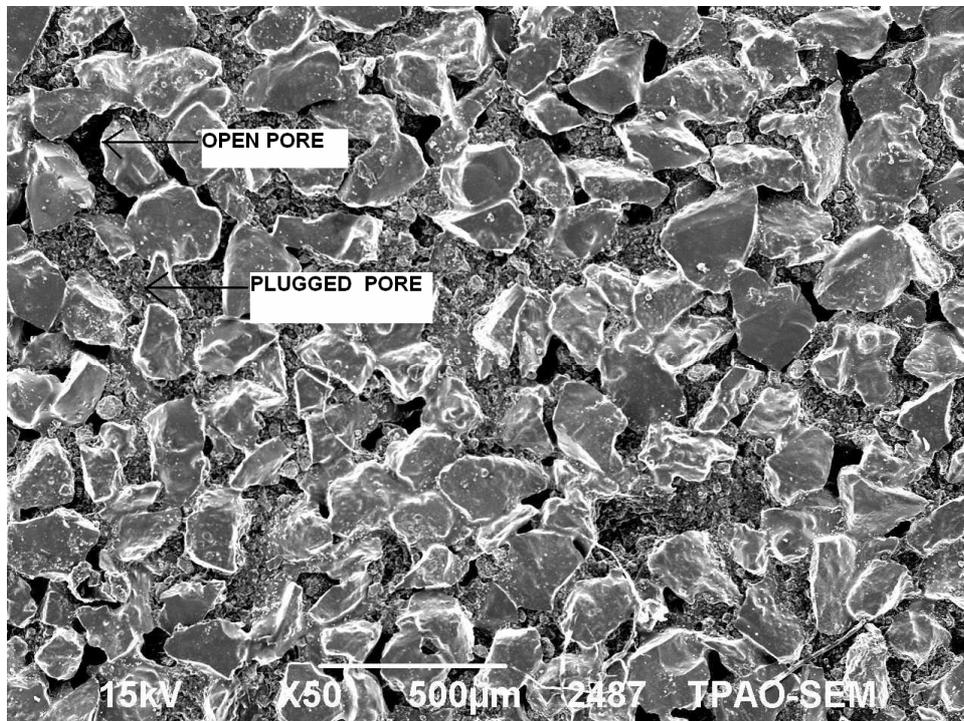
**Figure 5-6: 60 μ Ceramic Disk after PPT (30 lb/bbl of CaCO<sub>3</sub> C)**
