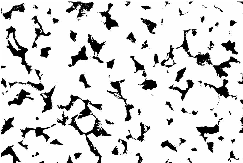
**Figure 4-5: Areas of Pores for 35  $\mu$  Ceramic Disk 70 X Focus**
