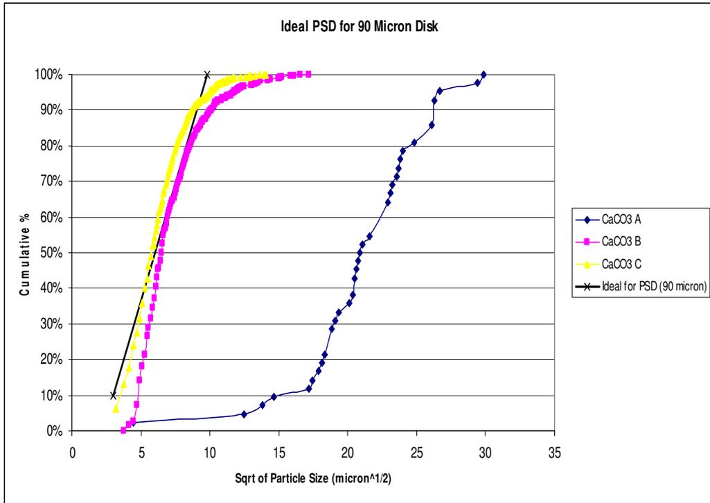
**Figure 5-15: Ideal PSD for 90  $\mu$  Ceramic Disks & CaCO<sub>3</sub> Grades**
