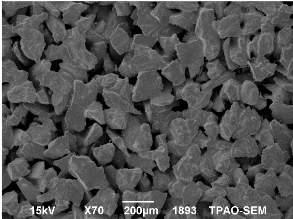
**Figure 4-4: SEM photograph of 35  $\mu$  Ceramic Disk 70 X Focus**
