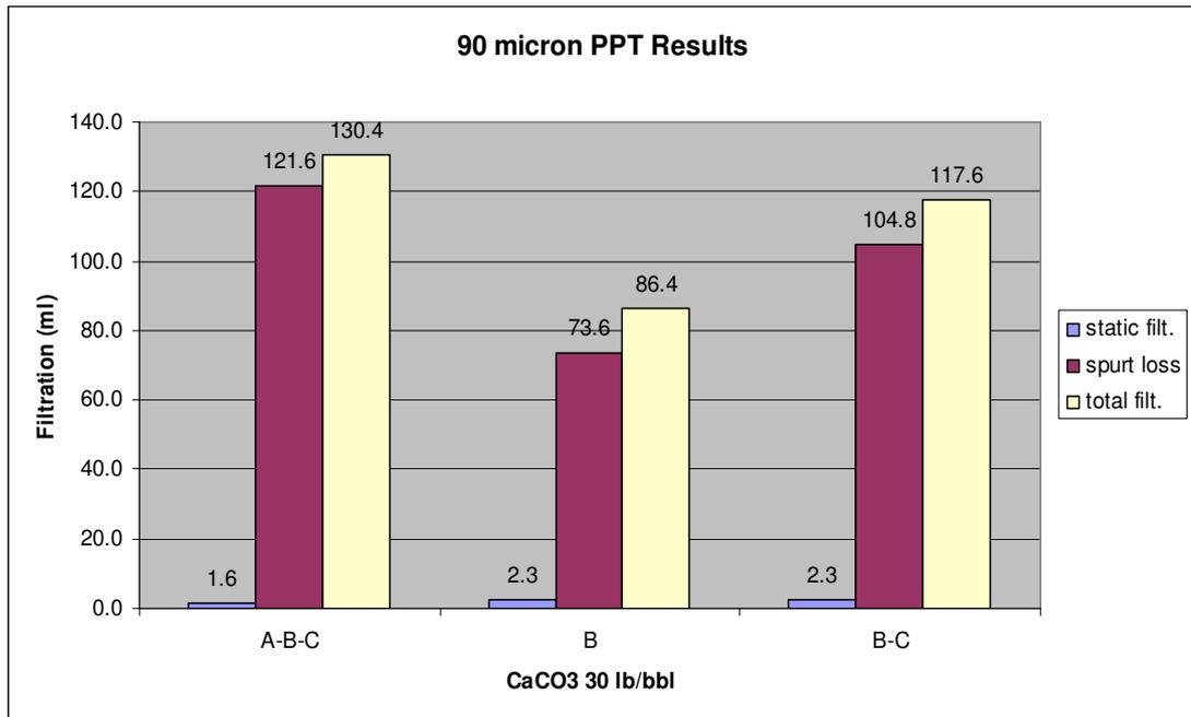
**Figure 5-12: Effect of particle size for 90 μ ceramic disks**
