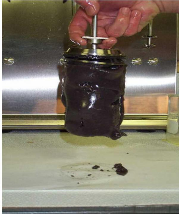
**Figure 2-3: Second generation CACP-firm, rubbery and ductile plug
