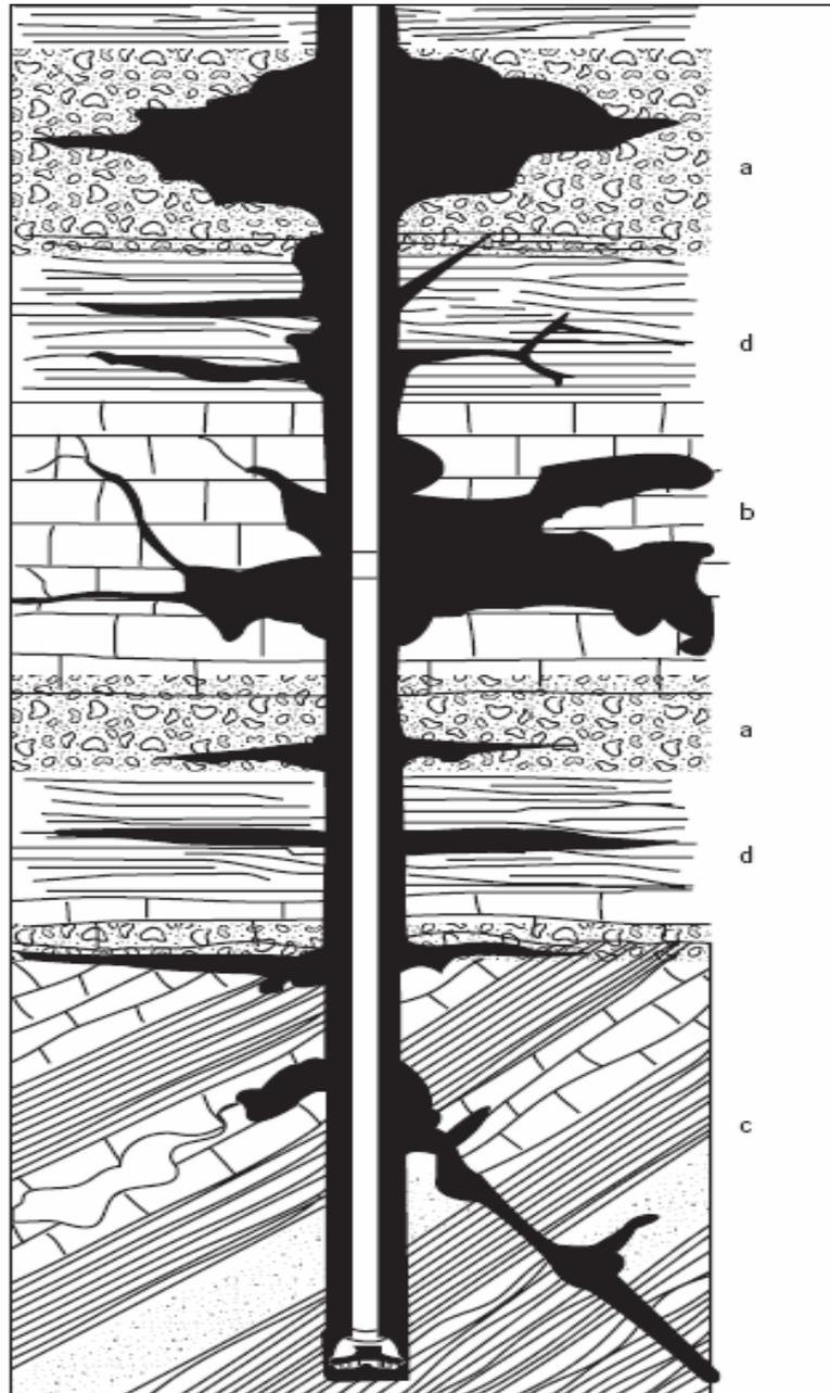
**Figure: 2-1: Lost Circulation Sections**
