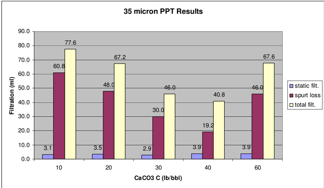
**Figure C-2: Effect of Concentration of CaCO<sub>3</sub> C (35 μ Ceramic Disks)**
