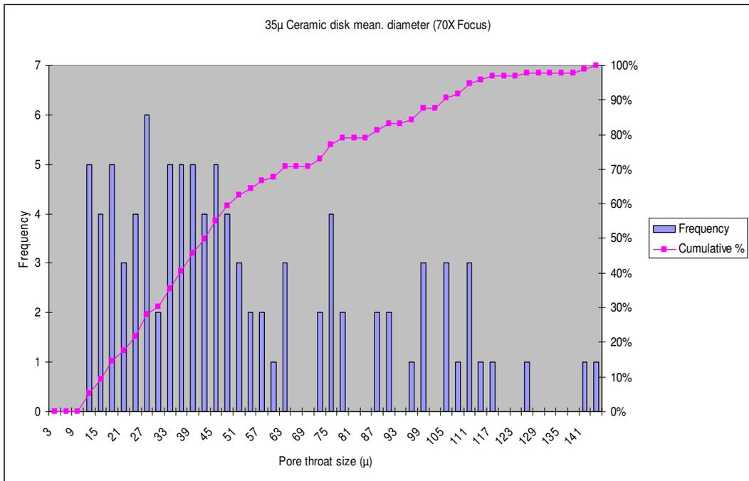
**Figure A-9: 35 $\mu$  Ceramic Disk Mean Diameter (70X Focus)**
