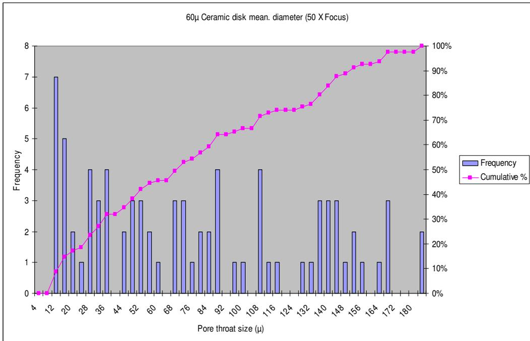
**Figure A-13: 60µ Ceramic Disk Mean Diameter (50X Focus)**
