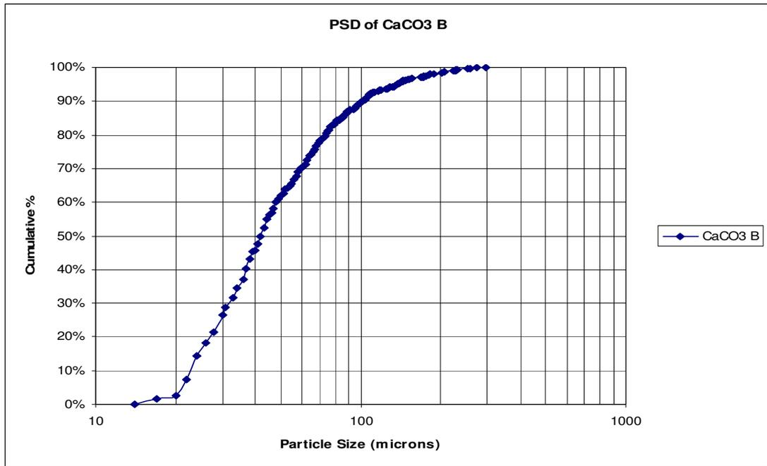
**Figure 5-3: PSD of CaCO<sub>3</sub> B**
