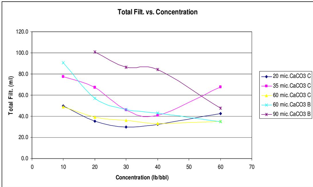
**Figure 5-8: Total Loss vs. Concentration**
