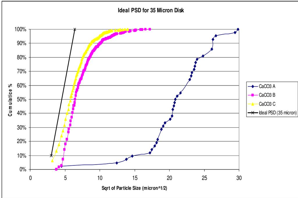
**Figure 5-13: Ideal PSD for 35  $\mu$  Ceramic Disks & CaCO<sub>3</sub> Grades**
