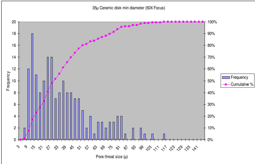
**Figure A-8: 35 $\mu$  Ceramic Disk Minimum Diameter (50X Focus)**
