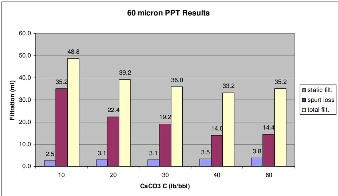
**Figure C-3: Effect of Concentration of CaCO<sub>3</sub> C (60 μ Ceramic Disks)**
