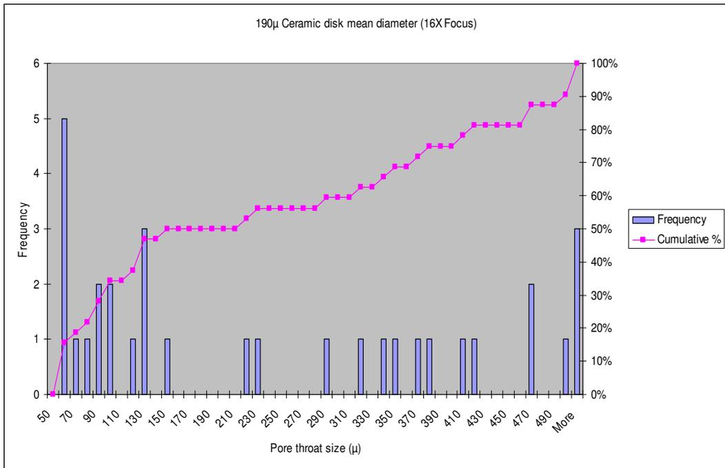
**Figure A-21: 190 $\mu$  Ceramic Disk Mean Diameter (16X Focus)**
