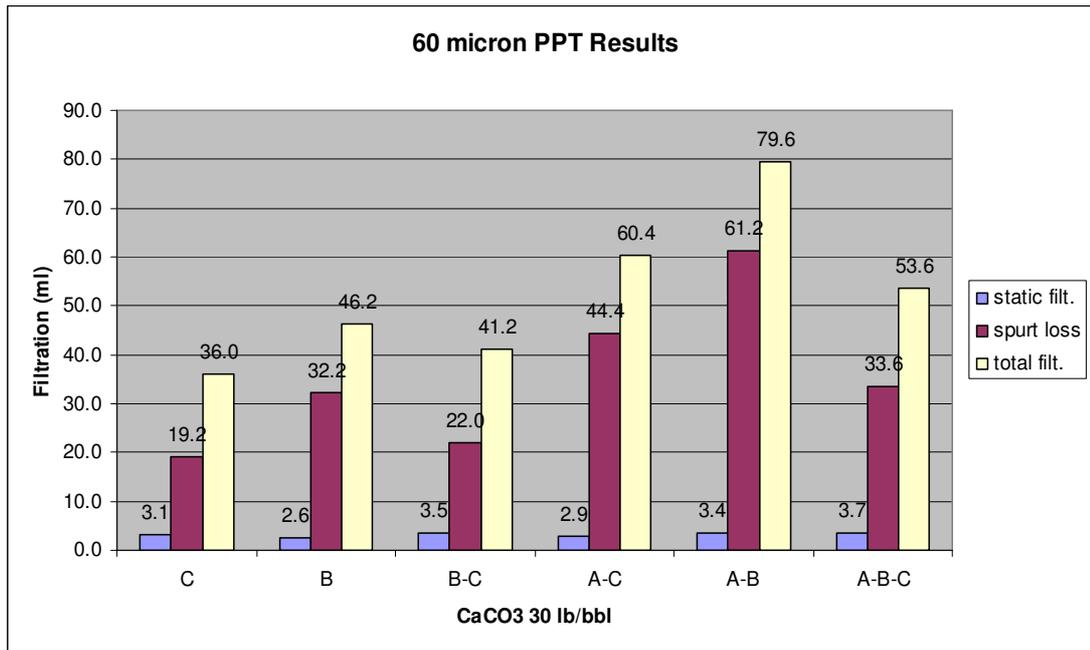
**Figure 5-11: Effect of particle size for 60  $\mu$  ceramic disks**
