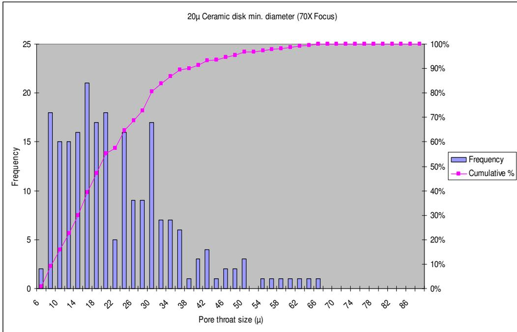
**Figure A-4: 20 $\mu$  Ceramic Disk Minimum Diameter (70X Focus)**
