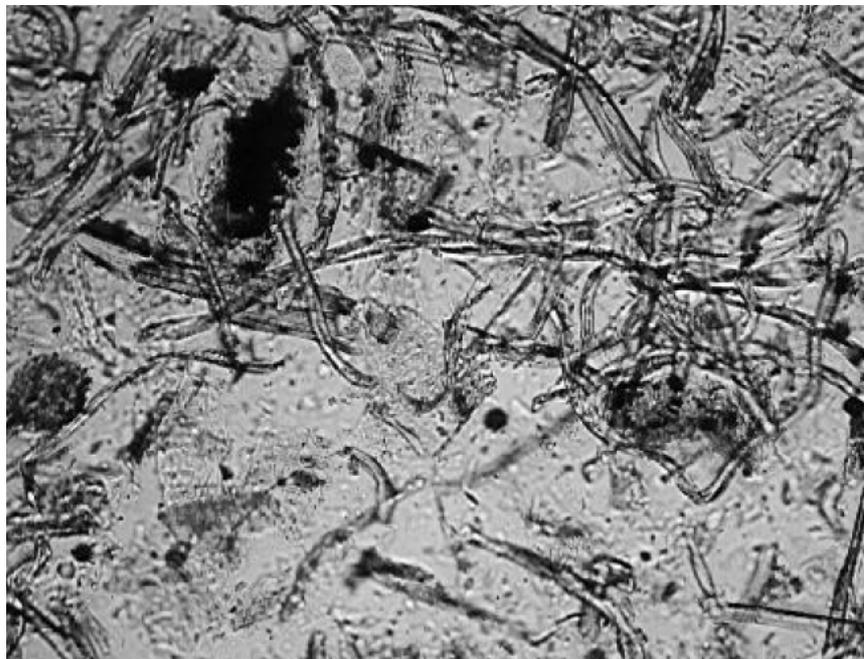
**Figure 2-4: Micronized Cellulose Fibers**
