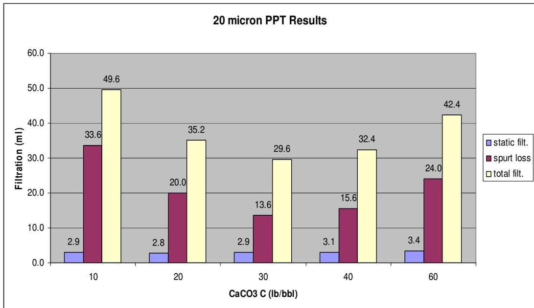
Figure C-1: Effect of Concentration of  $\text{CaCO}_3$  C (20  $\mu$  Ceramic Disks)
